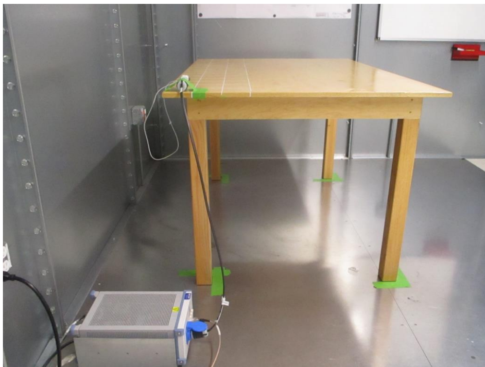
Figure 2: AC Line Conducted Emissions (Side View)
