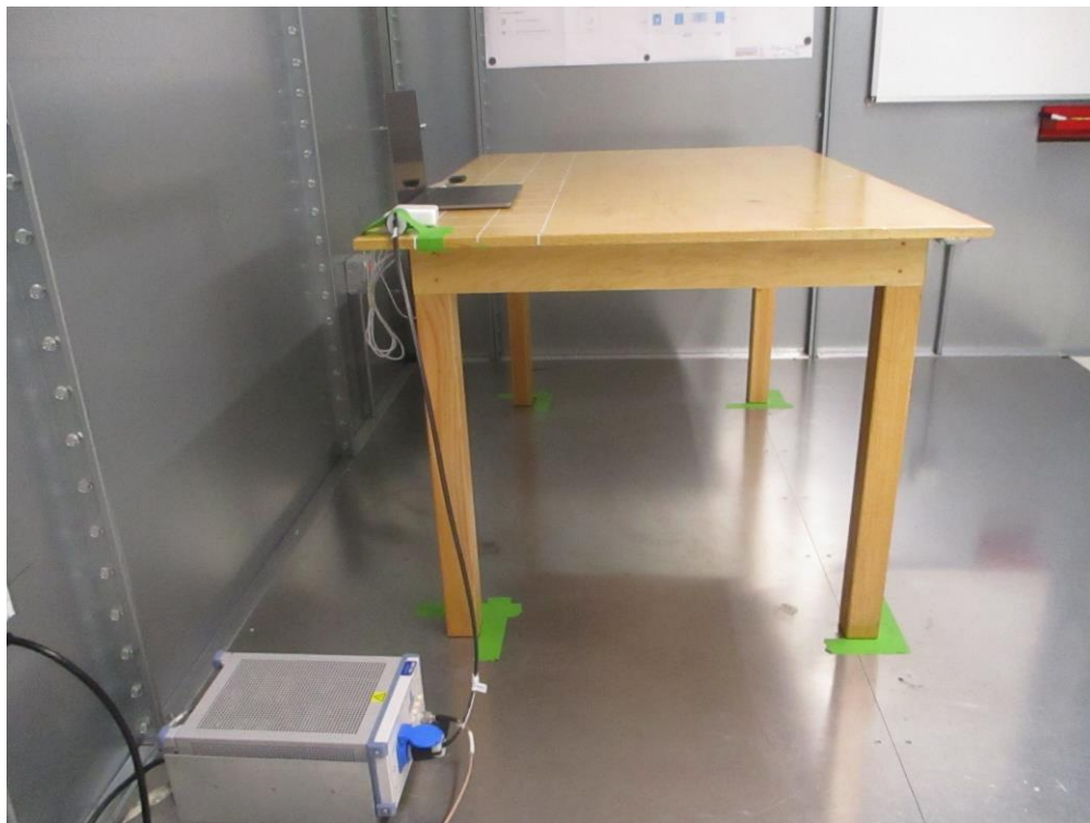
Figure 4: AC Line Conducted Emissions (Side View)
