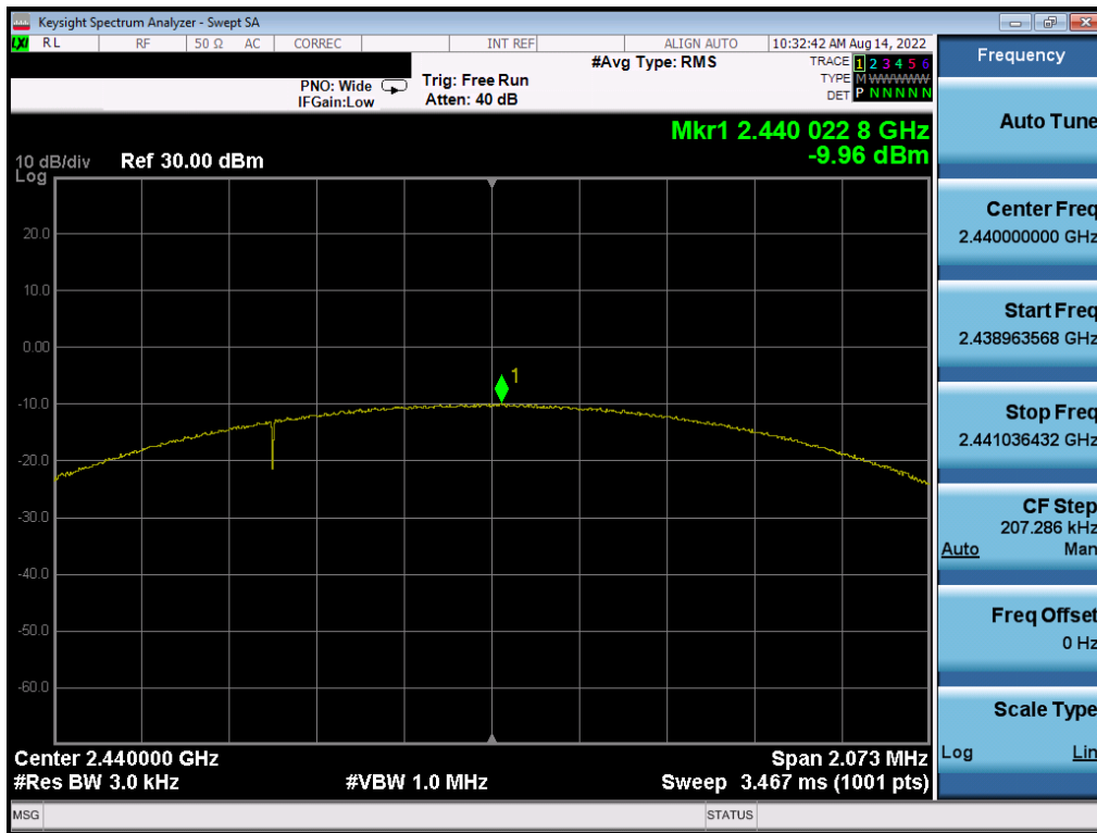
Plot 7-17. Power Spectral Density Plot (Bluetooth (LE), 2Mbps, iPA – Ch. 19)
