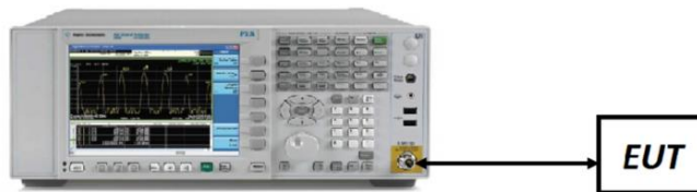
Figure 7-5. Test Instrument & Measurement Setup
