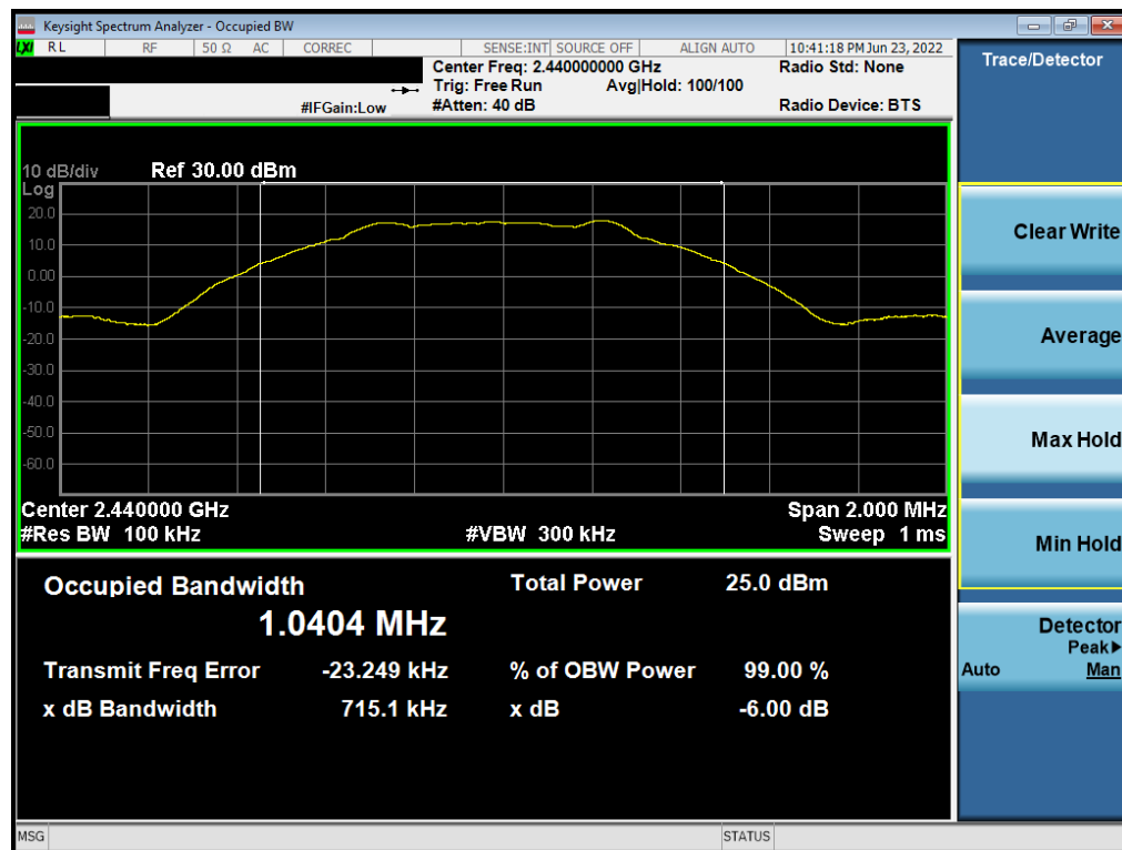
Plot 7-2. 6dB BW & 99% OBW Plot (Bluetooth (LE), 1Mbps, ePA – Ch. 19)
