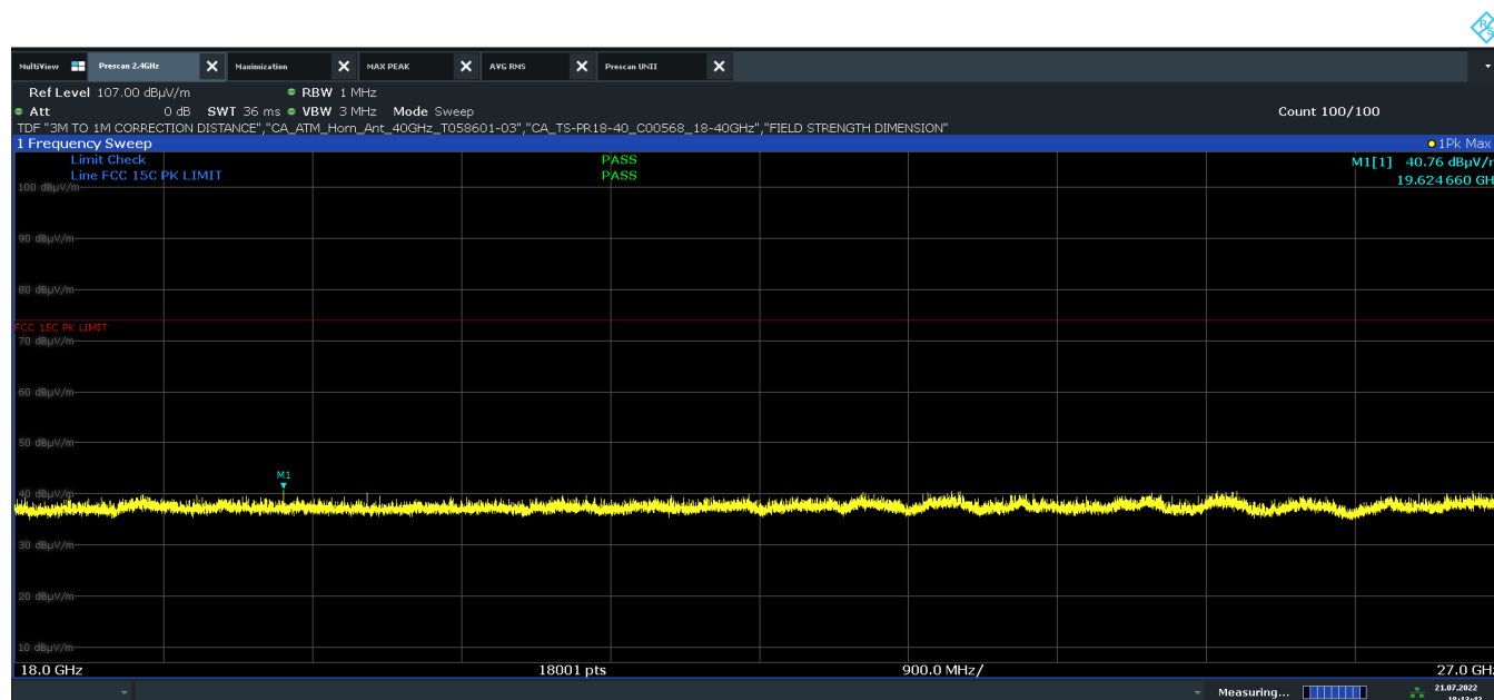
Plot 7-32. Radiated Spurious Plot Above 18GHz (1Mbps, ePA – Ch.19, Ant. Pol.H)
