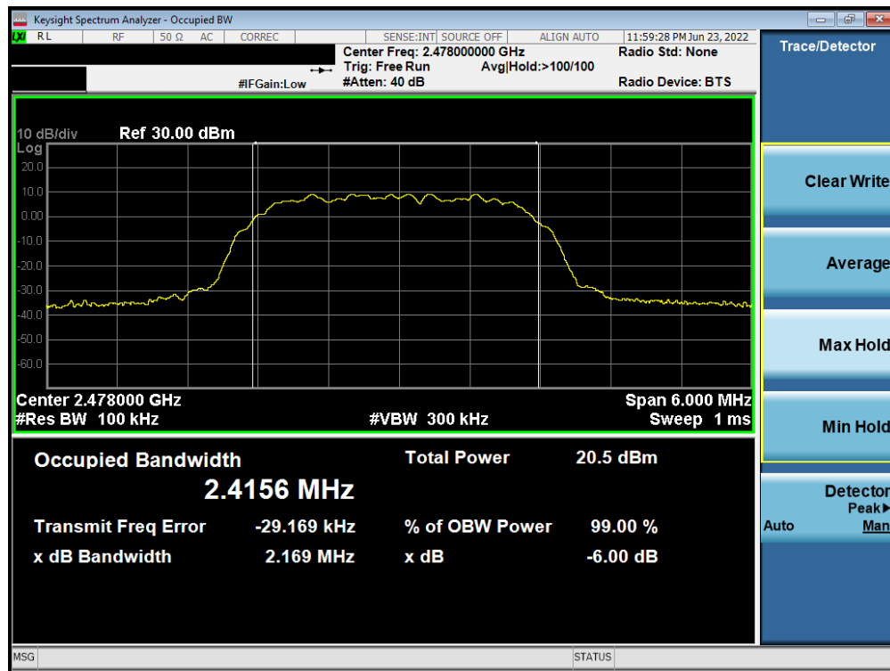
Plot 7-3. 6dB BW & 99% OBW Plot (Bluetooth (HDR4), 4Mbps, ePA – Ch. 75)
