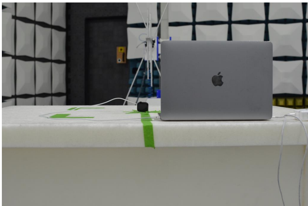
Figure 16: 30MHz-1GHz Test Setup (Rear View)
