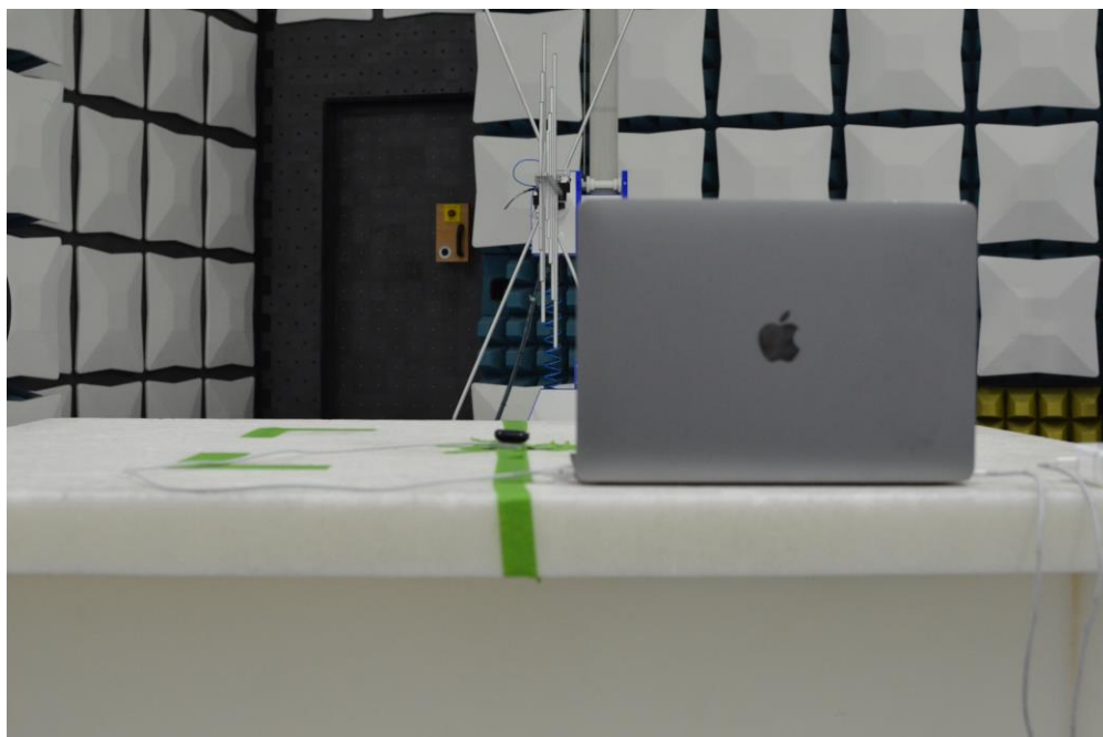
Figure 14: 30MHz-1GHz Test Setup (Rear View)
