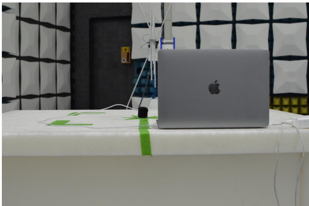
Figure 18: 30MHz-1GHz Test Setup (Rear View)
