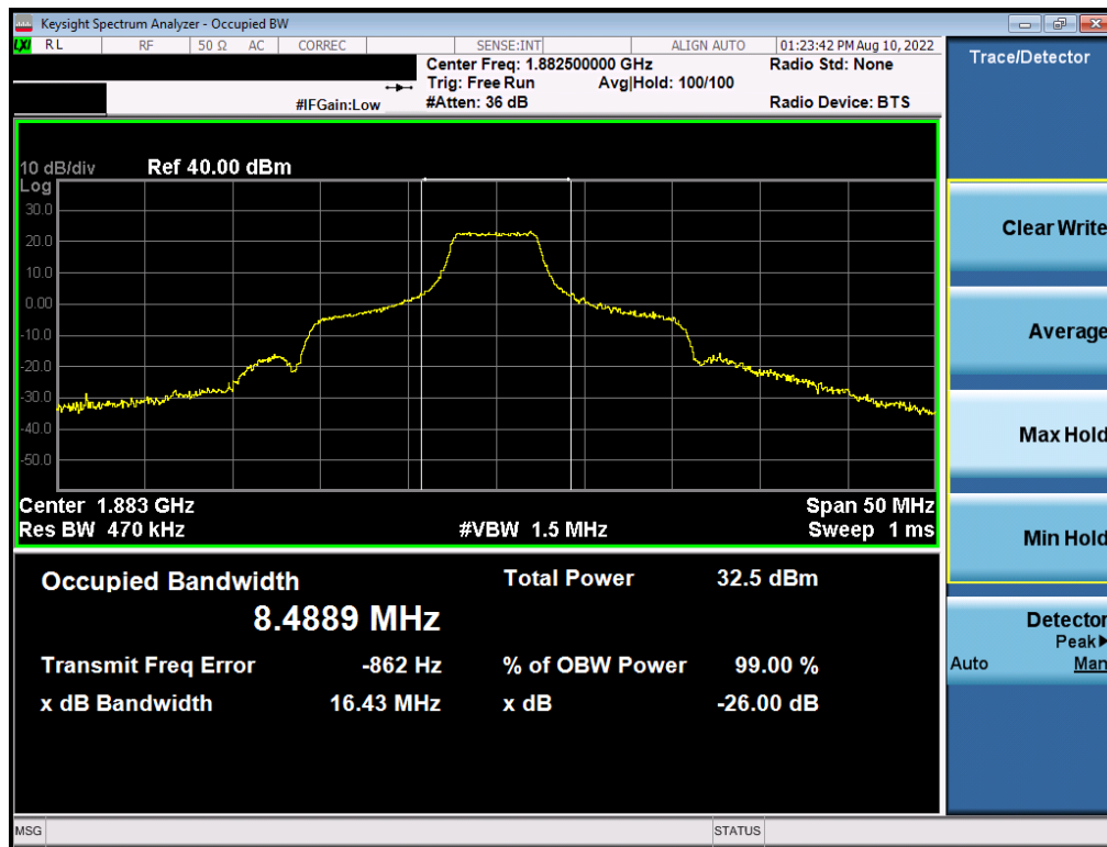
Plot 7-12. Occupied Bandwidth Plot (LTE Band 25/2 - 20MHz 16-QAM - Full RB Configuration)
