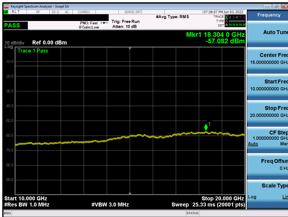
Plot 7-31. Conducted Spurious Plot (WCDMA Ch. 9538)
