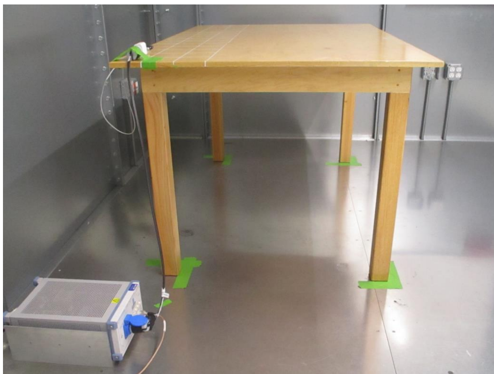
Figure 2: AC Line Conducted Emissions (Side View)
