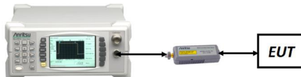
Figure 7-2. Test Instrument & Measurement Setup for Peak and Average Power Measurement
