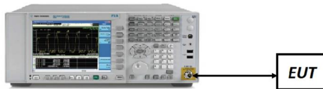
Figure 7-5. Test Instrument & Measurement Setup
