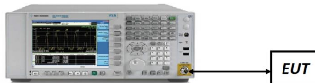
Figure 7-5. Test Instrument & Measurement Setup
