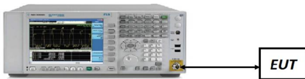
Figure 7-1. Test Instrument & Measurement Setup
