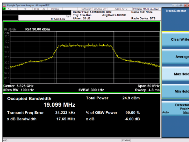
Plot 7-12. 6dB BW & 99% OBW (20MHz BW 802.11n – Ch. 165, MCS0)
