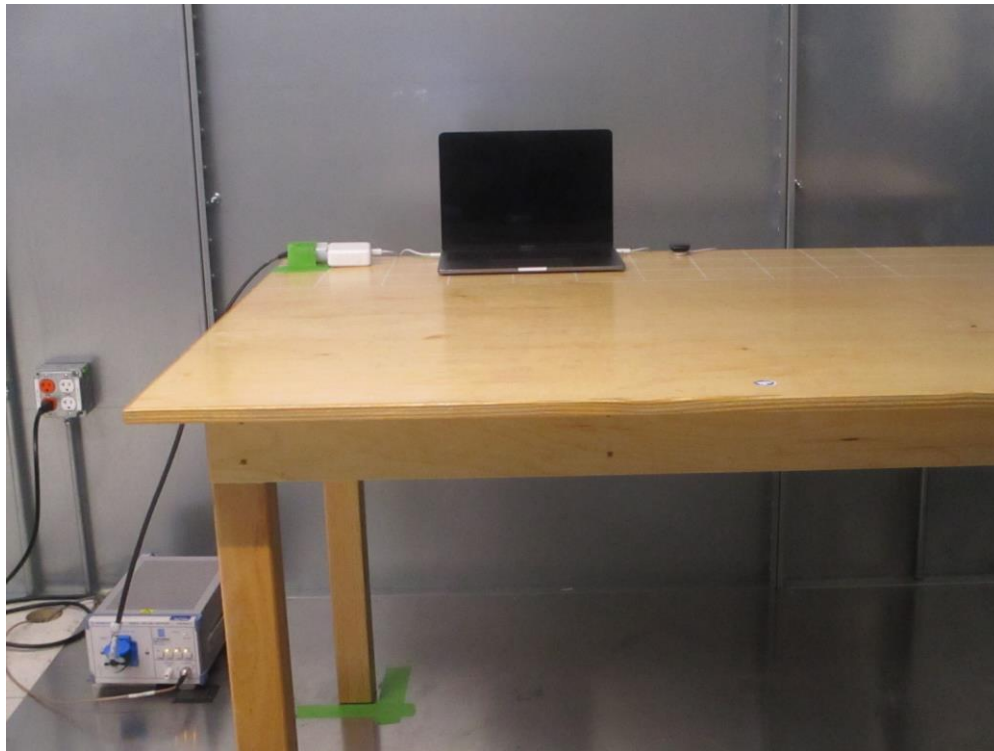
Figure 3: AC Line Conducted Emissions (Front View)
