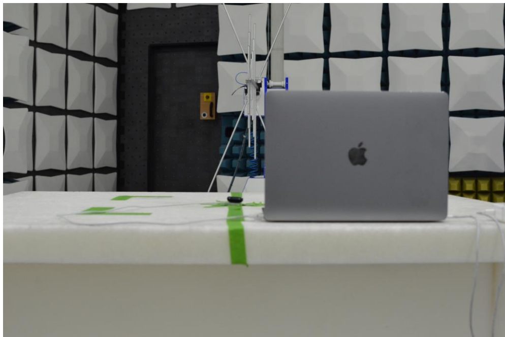
Figure 15: 30MHz-960MHz Test Setup (Rear View)
