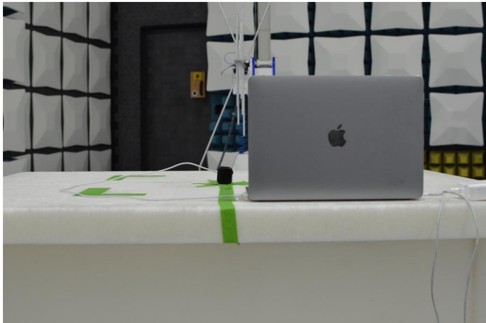
Figure 19: 30MHz-960MHz Test Setup (Rear View)
