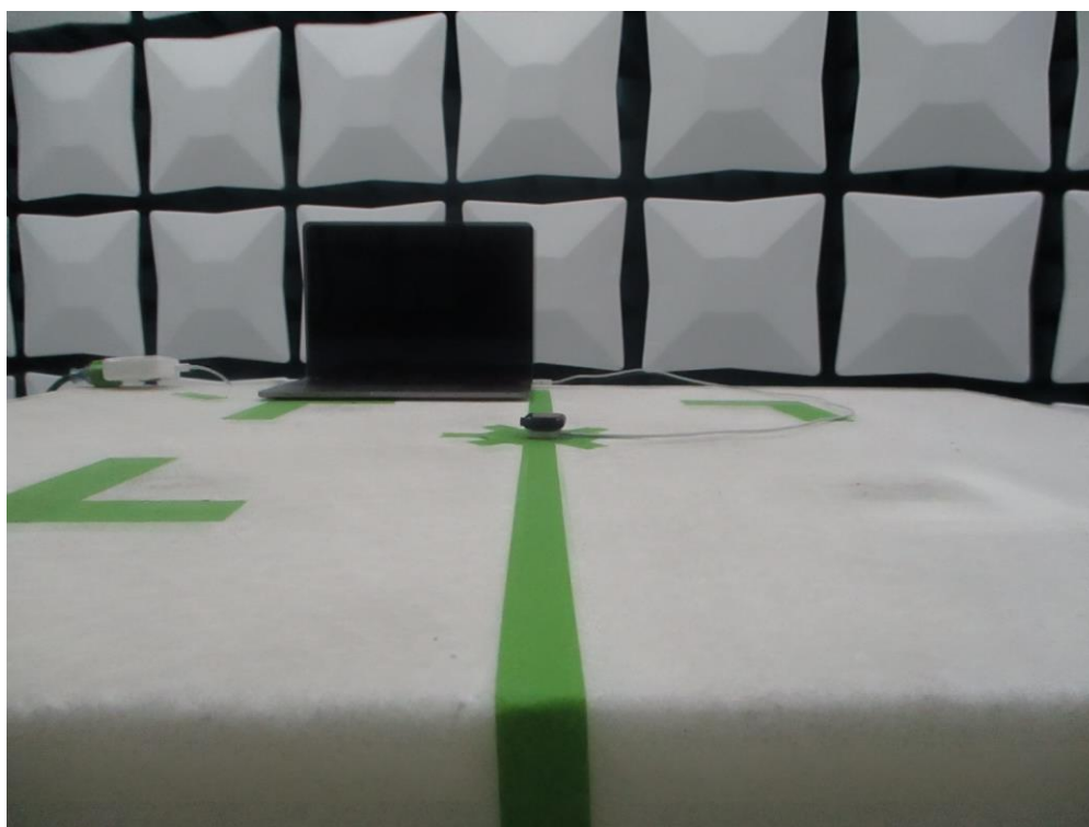
Figure 14: 30MHz-960MHz Test Setup (Front View)
