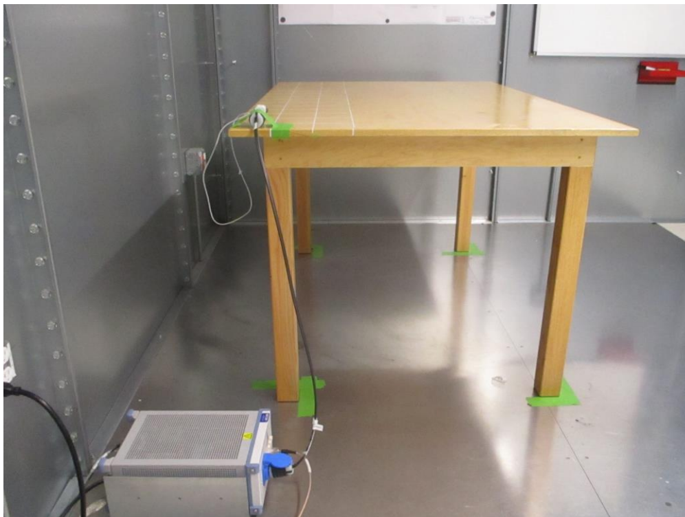
Figure 2: AC Line Conducted Emissions (Side View)
