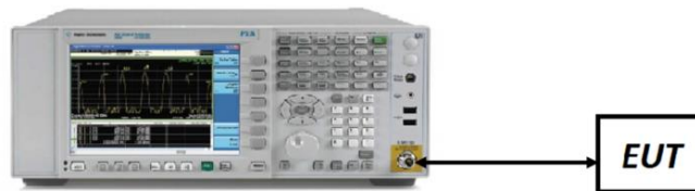
Figure 7-5. Test Instrument & Measurement Setup
