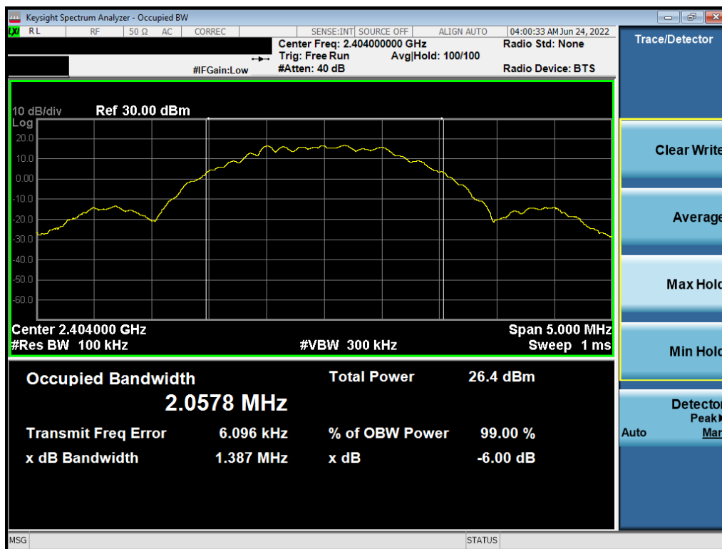
Plot 7-4. 6dB BW & 99% OBW Plot (Bluetooth (LE), 2Mbps, ePA – Ch. 1)
