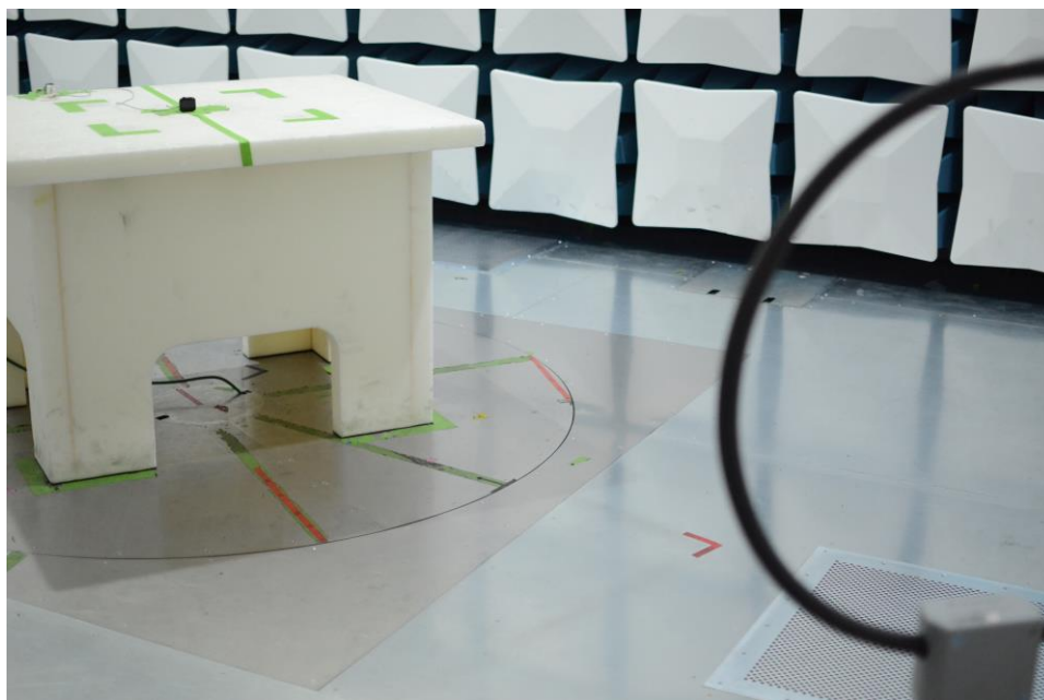
Figure 20: 9kHz-30MHz Test Setup (Front View)
