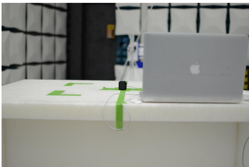
Figure 18: 30MHz-1GHz Test Setup (Rear View)
