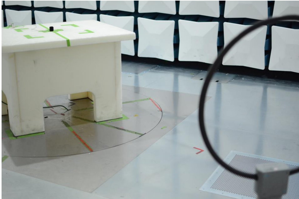
Figure 21: 9kHz-30MHz Test Setup (Front View)
