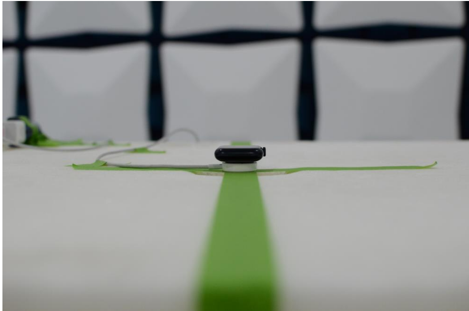
Figure 1: 1-18GHz Test Setup (Front View)
