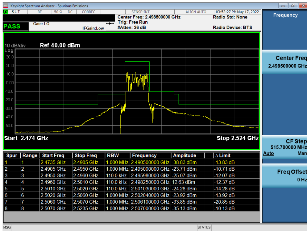
Plot 7-47. Lower ACP Plot (LTE Band 41 - 5MHz QPSK – Full RB)
