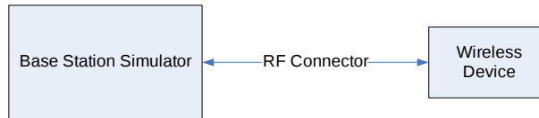
Figure 8-2 Power Measurement Setup
