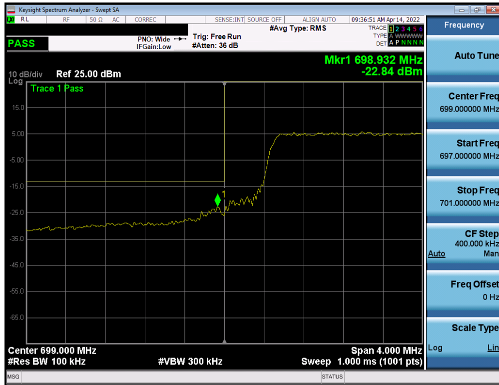
Plot 7-110. Lower Band Edge Plot (LTE Band 12 - 10MHz QPSK – Full RB)
