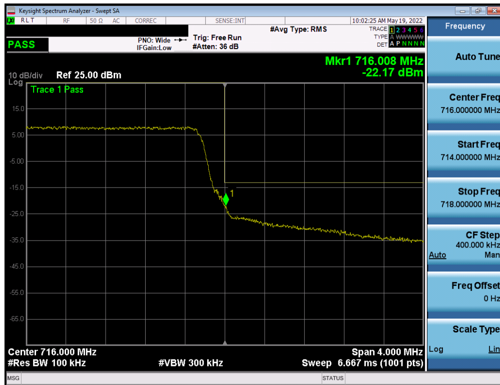
Plot 7-109. Upper Band Edge Plot (LTE Band 12 - 5MHz QPSK – Full RB)
