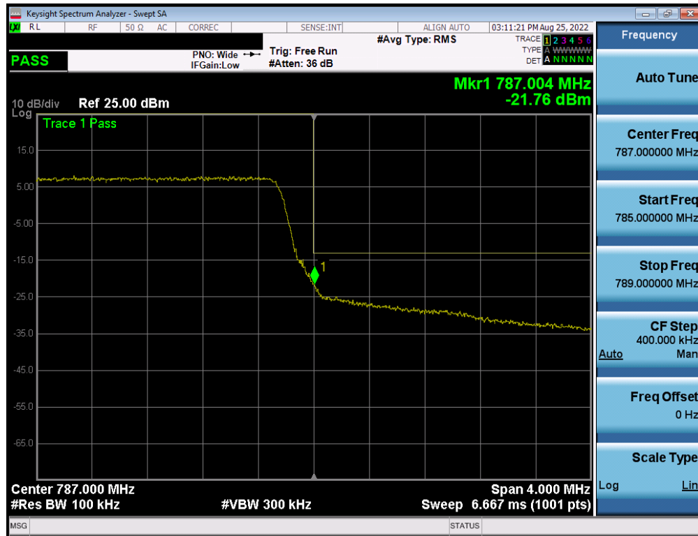
Plot 7-118. Upper Band Edge Plot (LTE Band 13 - 5MHz QPSK – Full RB)
