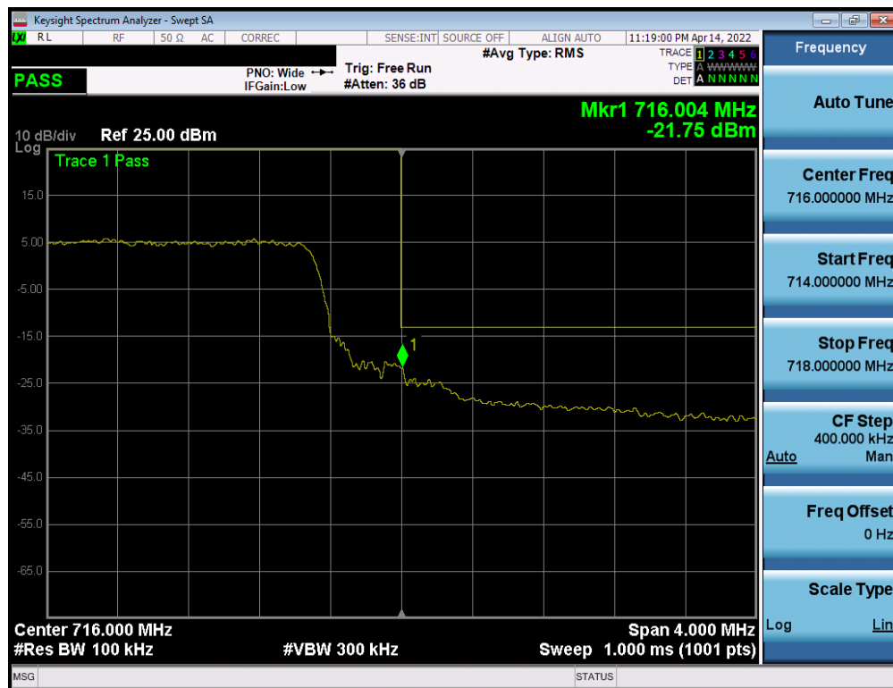
Plot 7-115. Upper Band Edge Plot (LTE Band 17 - 10MHz QPSK – Full RB)
