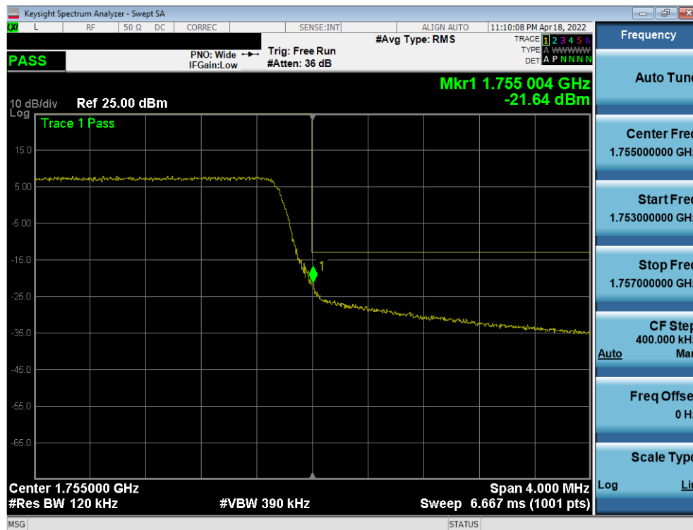
Plot 7-90. Upper Band Edge Plot (LTE Band 4 - 5MHz QPSK – Full RB)
