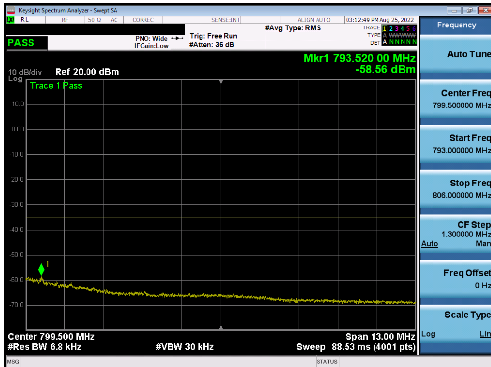
Plot 7-119. Upper Emission Mask Plot (LTE Band 13 - 5MHz QPSK – Full RB)
