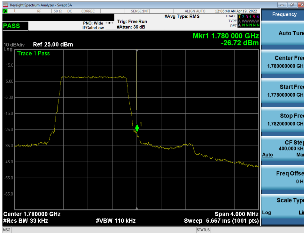
Plot 7-58. Upper Band Edge Plot (LTE Band 66 – 1.4MHz QPSK – Full RB)
