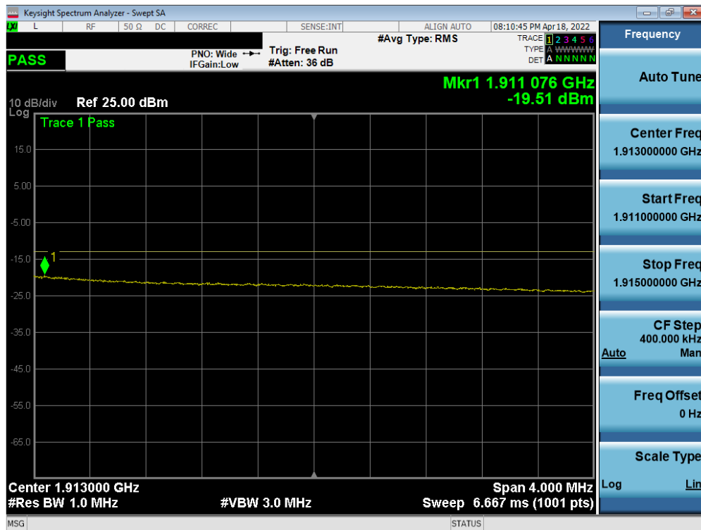
Plot 7-79. Extended Upper Band Edge Plot (LTE Band 2 – 20MHz QPSK – Full RB Configuration)
