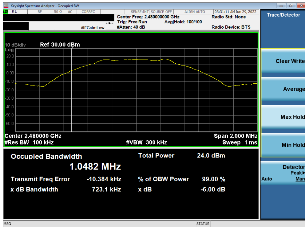
Plot 7-3. 6dB BW & 99% OBW Plot (Bluetooth (LE), 1Mbps, ePA – Ch. 39)
