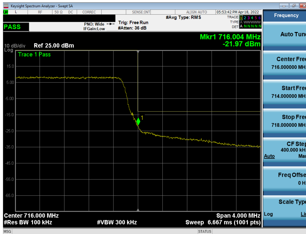
Plot 7-113. Upper Band Edge Plot (LTE Band 17 - 5MHz QPSK – Full RB)
