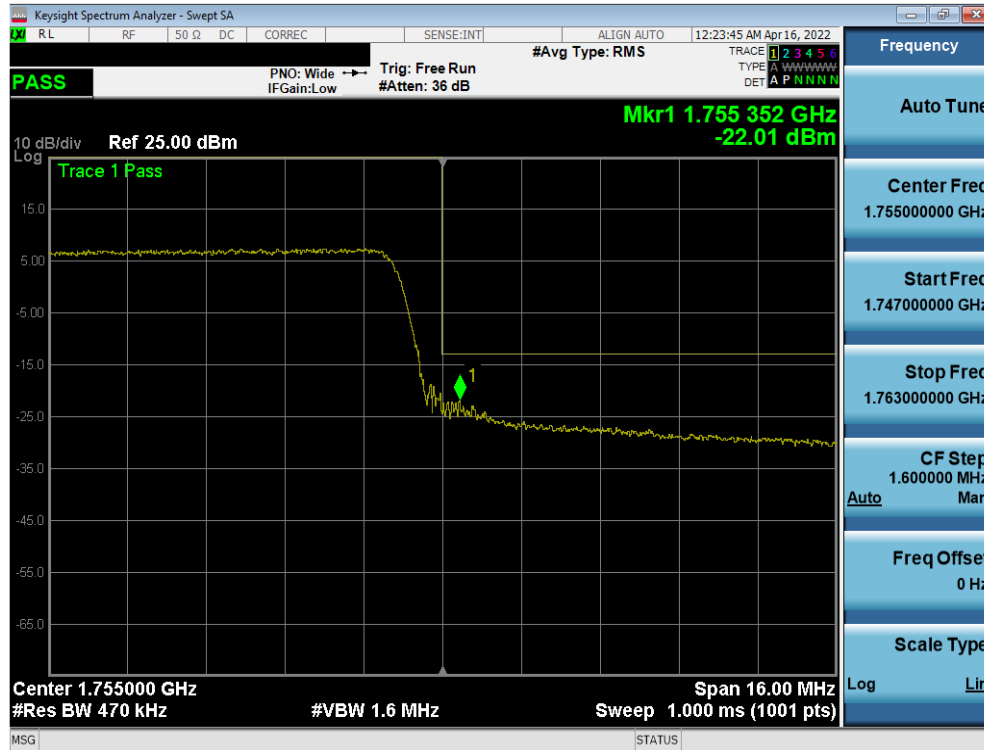
Plot 7-102. Upper Band Edge Plot (LTE Band 4 - 20MHz QPSK – Full RB)
