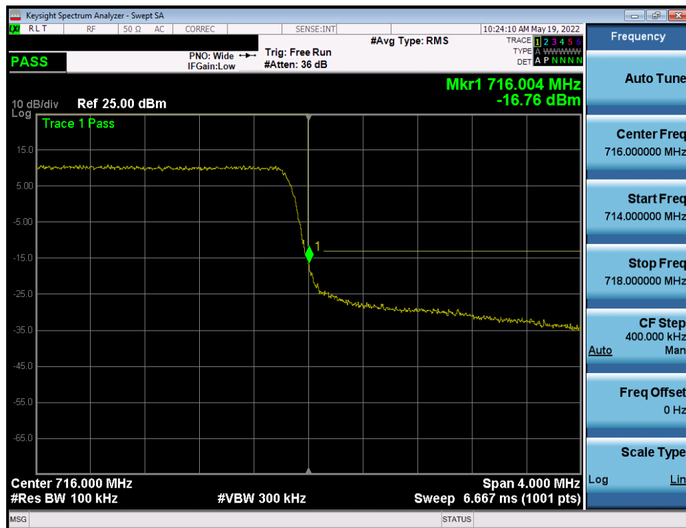
Plot 7-107. Upper Band Edge Plot (LTE Band 12 - 3MHz QPSK – Full RB)
