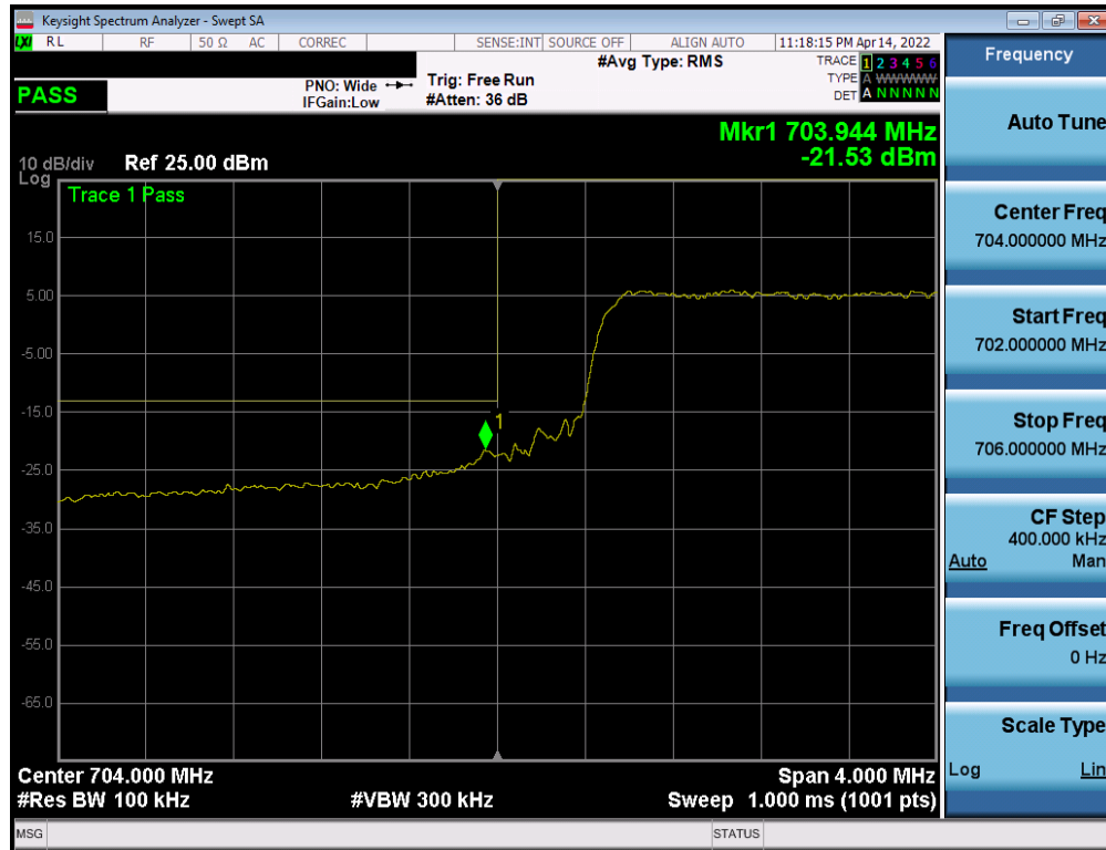
Plot 7-114. Lower Band Edge Plot (LTE Band 17 - 10MHz QPSK – Full RB)
