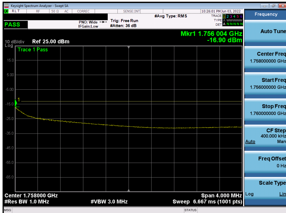
Plot 7-127. Upper Extended Band Edge Plot (WCDMA AWS – Ch. 1513)
