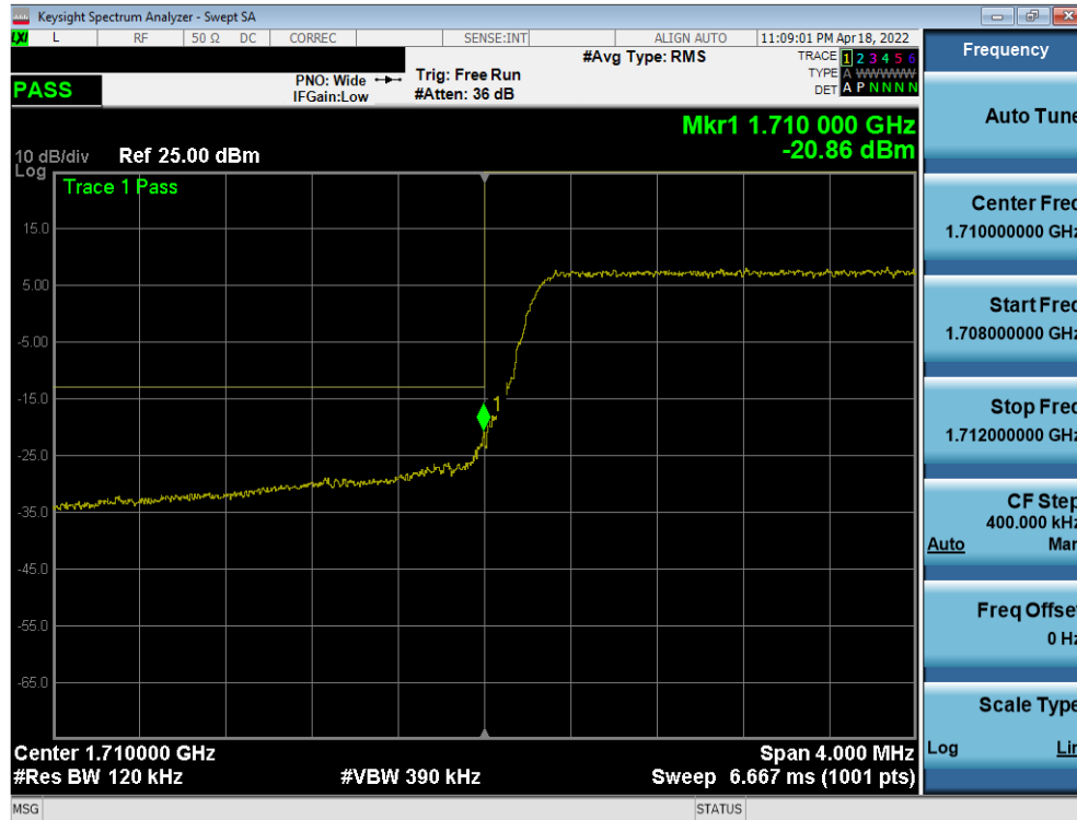
Plot 7-88. Lower Band Edge Plot (LTE Band 4 - 5MHz QPSK – Full RB)
