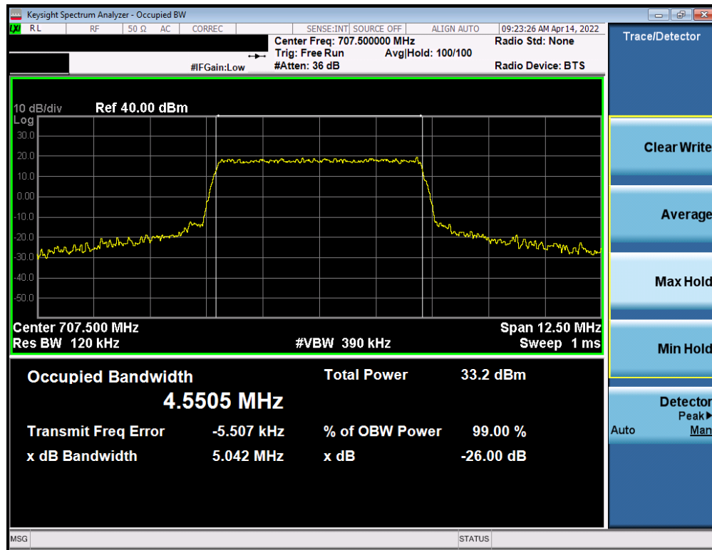
Plot 7-17. Occupied Bandwidth Plot (LTE Band 12/17 - 5MHz QPSK - Full RB)
