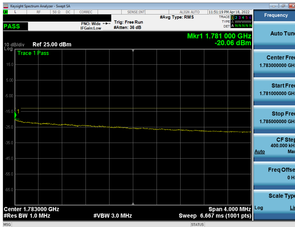
Plot 7-71. Upper Extended Band Edge Plot (LTE Band 66 - 10MHz QPSK – Full RB)
