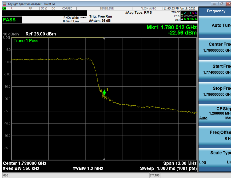
Plot 7-74. Upper Band Edge Plot (LTE Band 66 - 15MHz QPSK – Full RB)
