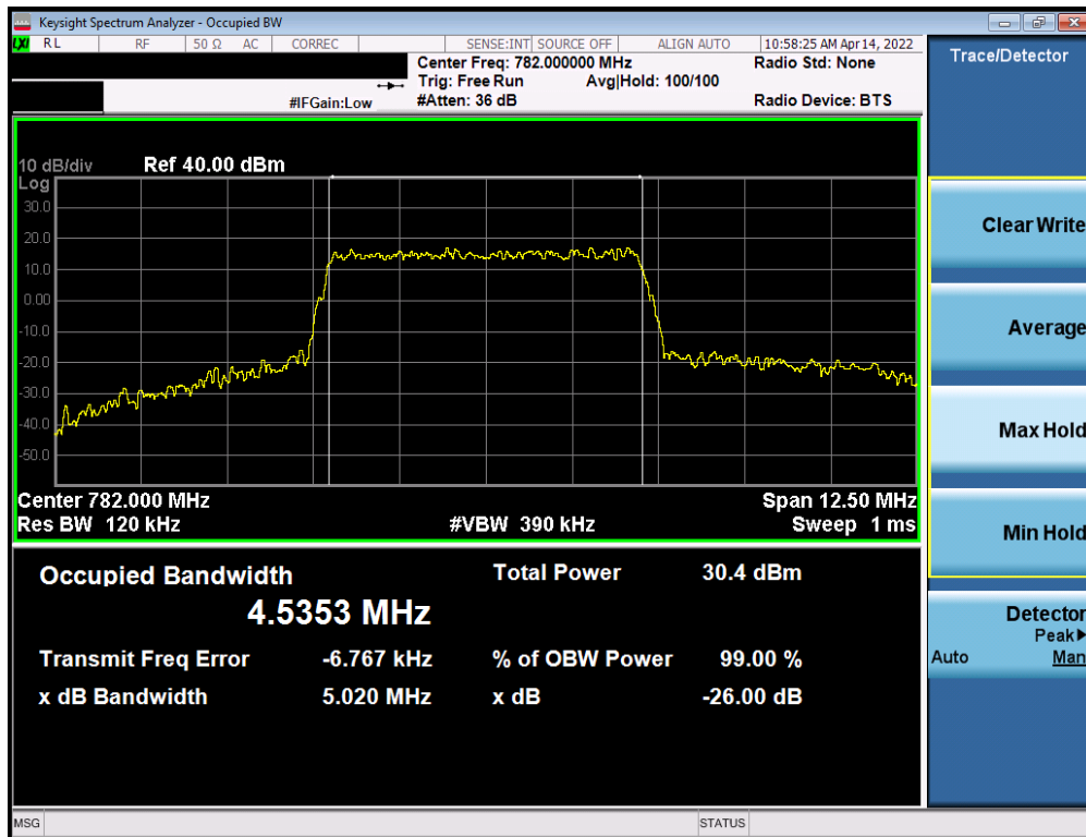
Plot 7-22. Occupied Bandwidth Plot (LTE Band 13 - 5MHz 16-QAM - Full RB)
