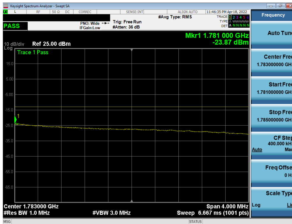
Plot 7-75. Upper Extended Band Edge Plot (LTE Band 66 - 15MHz QPSK – Full RB)
