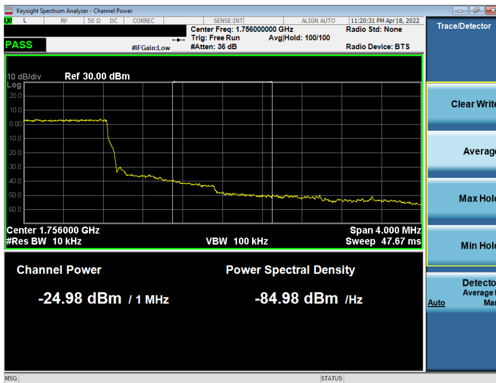
Plot 7-83. Upper Extended Band Edge Plot (LTE Band 4 – 1.4MHz QPSK – Full RB)
