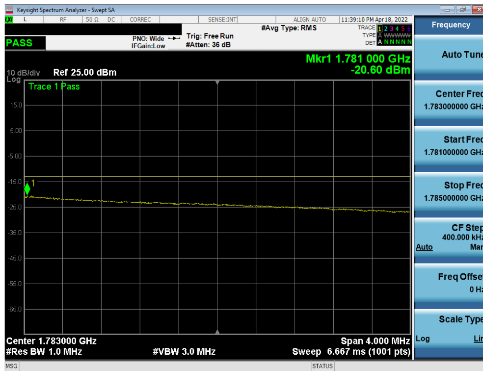
Plot 7-79. Upper Extended Band Edge Plot (LTE Band 66 - 20MHz QPSK – Full RB)
