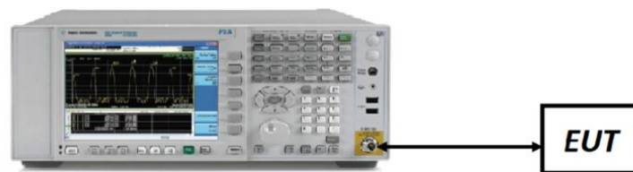
Figure 7-3. Test Instrument & Measurement Setup
