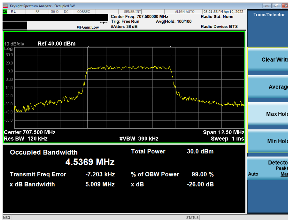
Plot 7-18. Occupied Bandwidth Plot (LTE Band 12/17 - 5MHz 16-QAM - Full RB)
