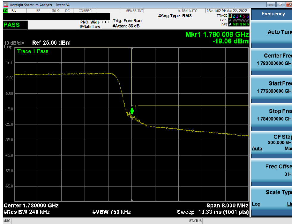
Plot 7-70. Upper Band Edge Plot (LTE Band 66 - 10MHz QPSK – Full RB)
