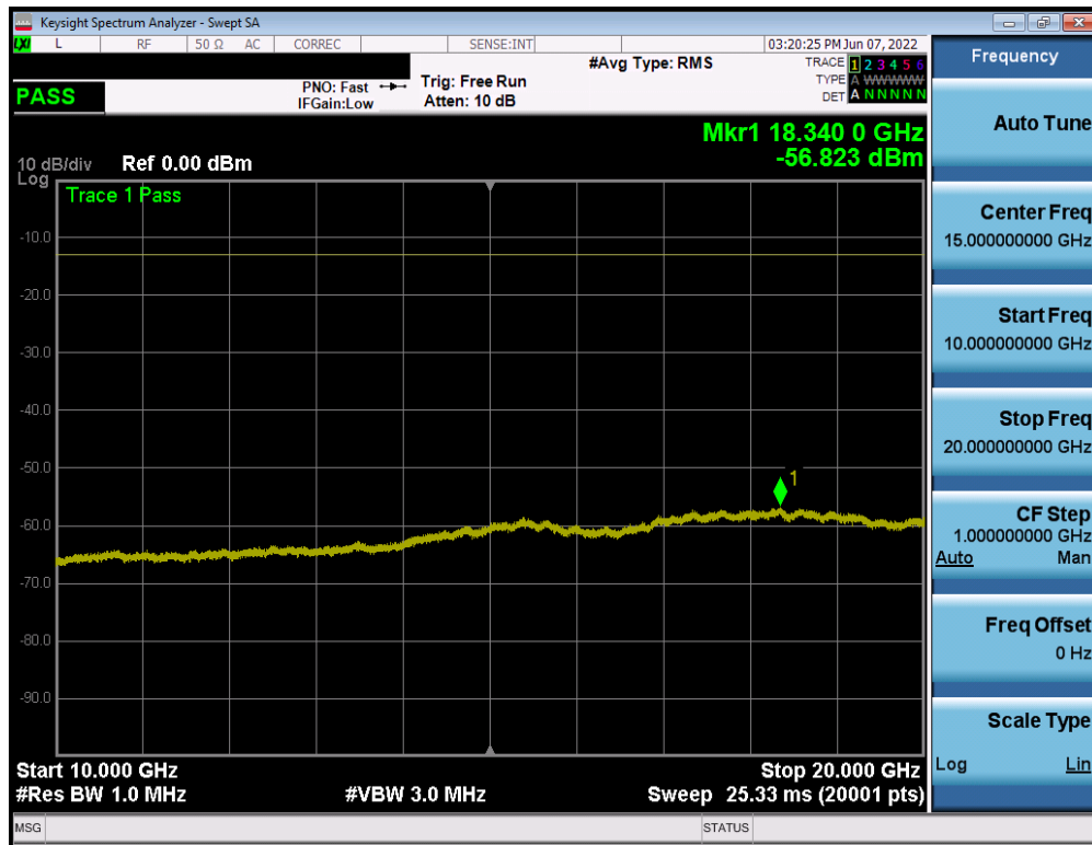
Plot 7-28. Conducted Spurious Plot (LTE Band 66/4 - 20MHz QPSK - RB Size 1, RB Offset 0 - Low Channel)
