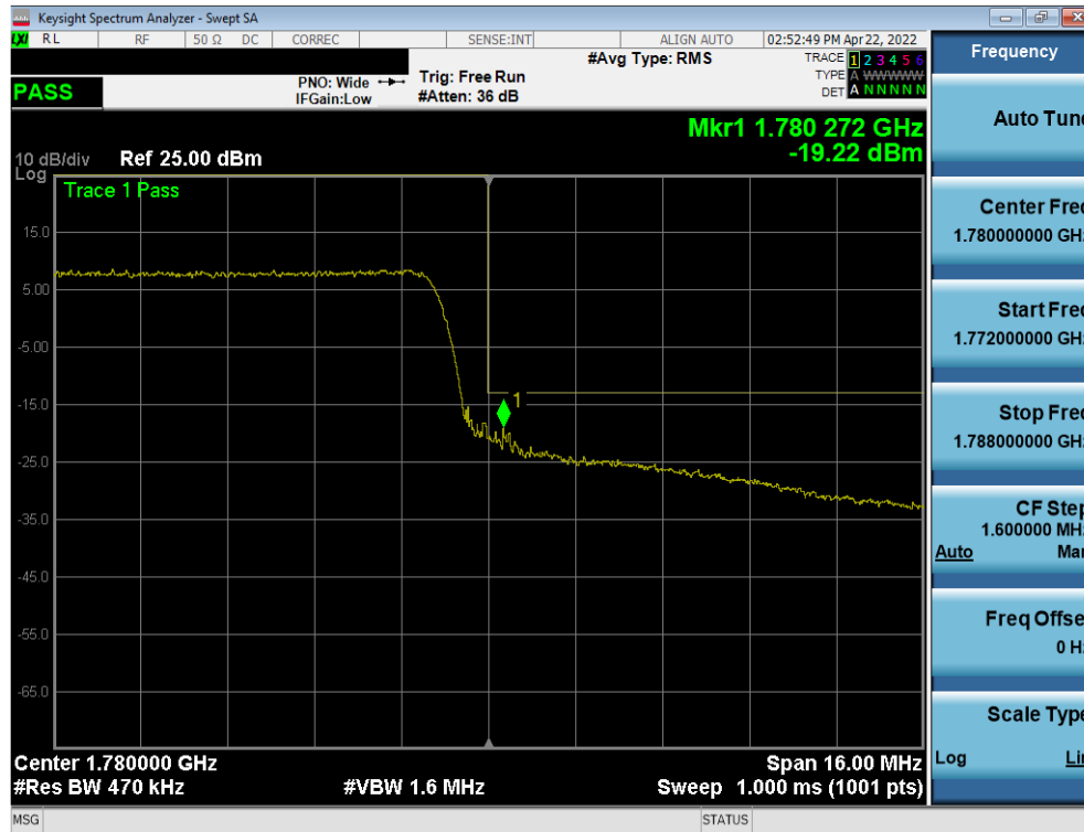
Plot 7-78. Upper Band Edge Plot (LTE Band 66 - 20MHz QPSK – Full RB)
