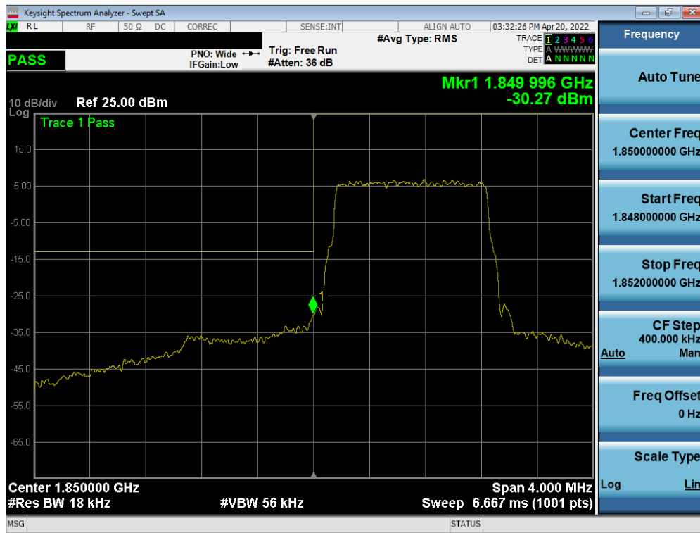
Plot 7-56. Lower Band Edge Plot (LTE Band 2 – 1.4MHz QPSK – Full RB Configuration)
