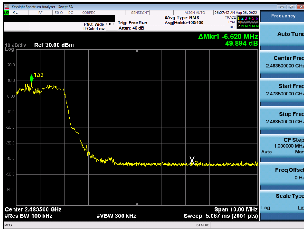
Plot 7-14. Band Edge Plot (Bluetooth with Hopping Enabled, 8DPSK, ePA)
