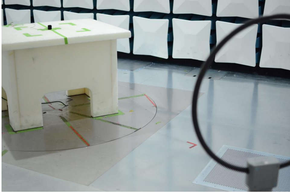
Figure 25: 9kHz-30MHz Test Setup (Front View)
