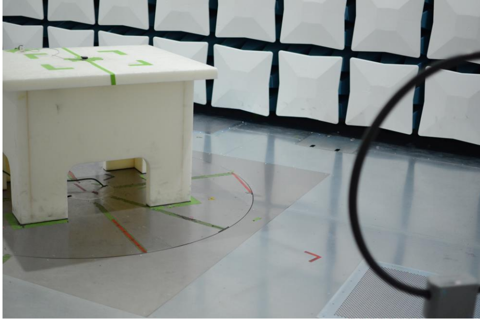
Figure 23: 9kHz-30MHz Test Setup (Front View)
