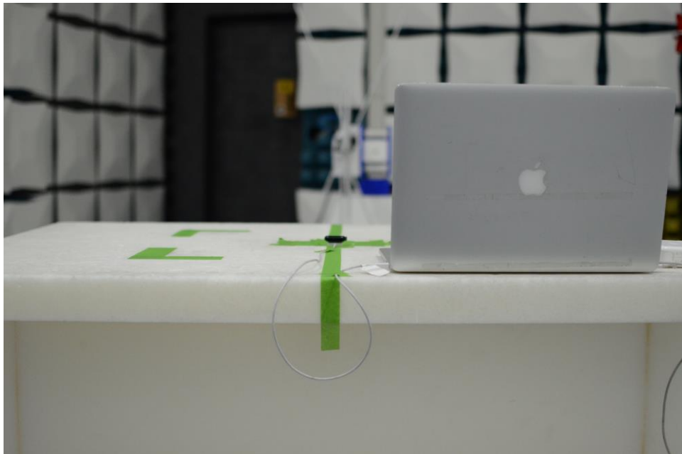
Figure 18: 30MHz-1GHz Test Setup (Rear View)
