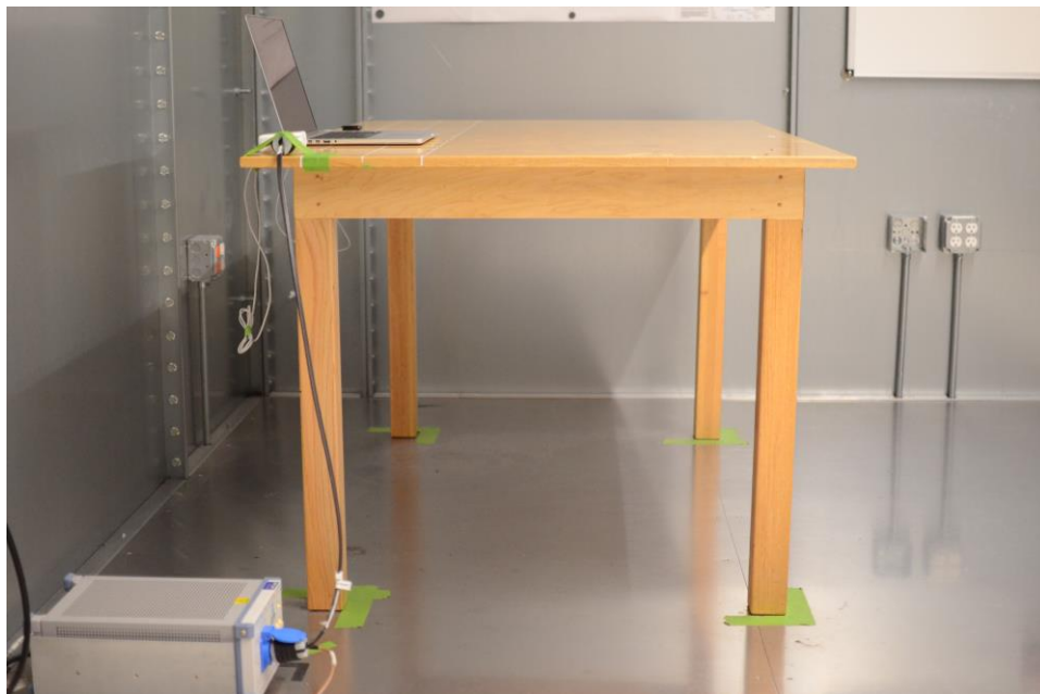
Figure 4: AC Line Conducted Emissions (Side View)
