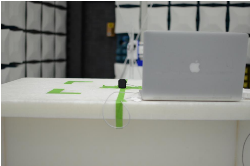
Figure 22: 30MHz-1GHz Test Setup (Rear View)
