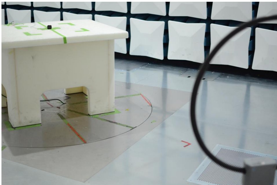
Figure 24: 9kHz-30MHz Test Setup (Front View)
