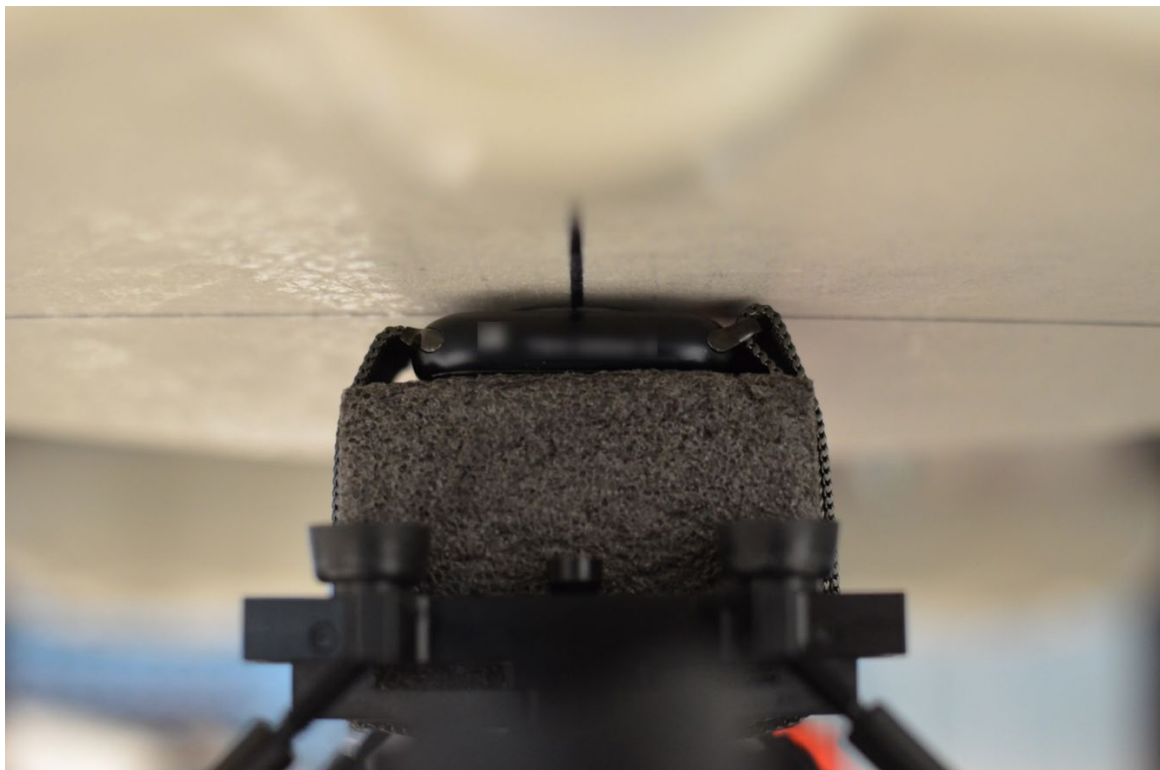
SAR Test Setup Photo 6: Aluminum with Metal Loop Wristband, Extremity, Back Side at 0.0 mm
