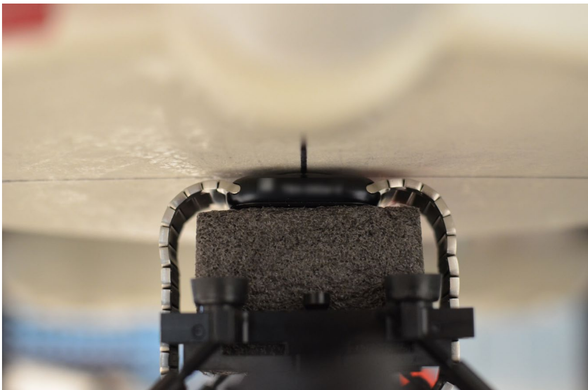
SAR Test Setup Photo 5: Aluminum with Metal Links Wristband, Extremity, Back Side at 0.0 mm
