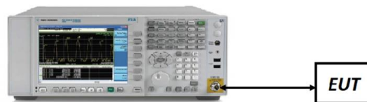
Figure 7-7. Test Instrument & Measurement Setup
