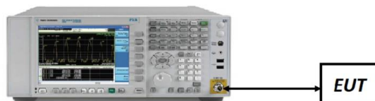
Figure 7-1. Test Instrument & Measurement Setup
