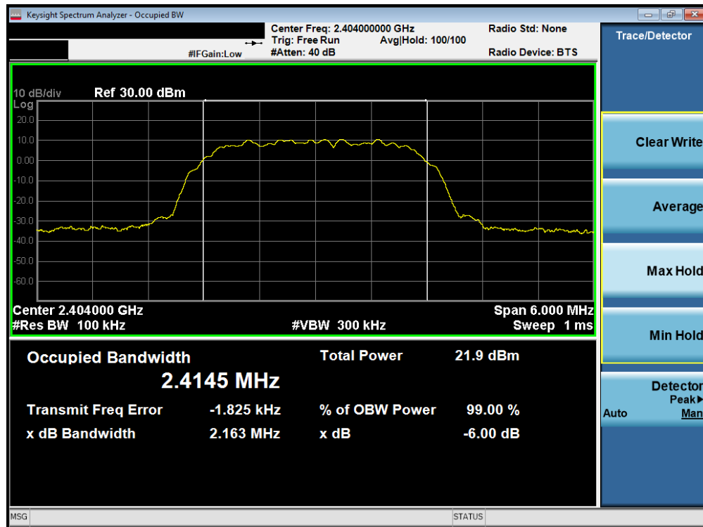
Plot 7-1. 6dB BW & 99% OBW Plot (Bluetooth (HDR4), 4Mbps, ePA – Ch. 1)
