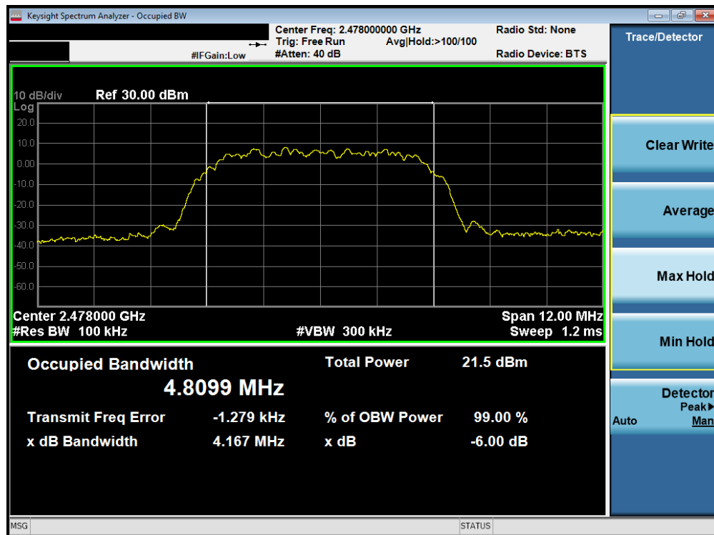
Plot 7-6. 6dB BW & 99% OBW Plot (Bluetooth (HDR8), 8Mbps, ePA – Ch. 75)
