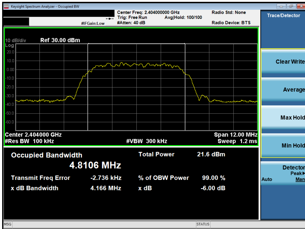
Plot 7-4. 6dB BW & 99% OBW Plot (Bluetooth (HDR8), 8Mbps, ePA – Ch. 1)
