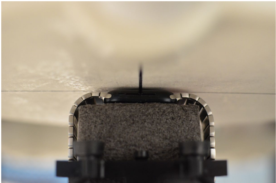
SAR Test Setup Photo 5: Aluminum with Metal Links Wristband, Extremity, Back Side at 0.0 cm
