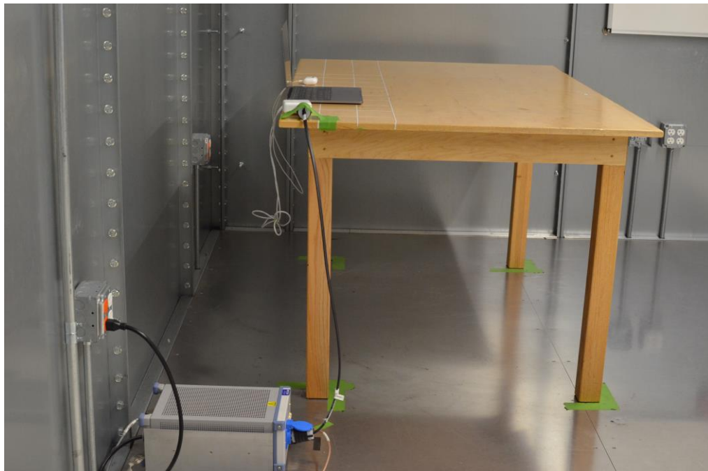
Figure 4: AC Line Conducted Emissions (Side View)
