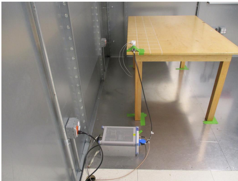
Figure 2: AC Line Conducted Emissions (Side View)
