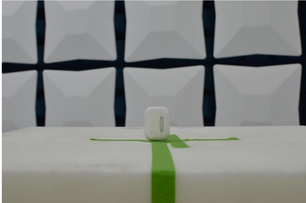
Figure 7: 1-18GHz Test Setup (Front View)
