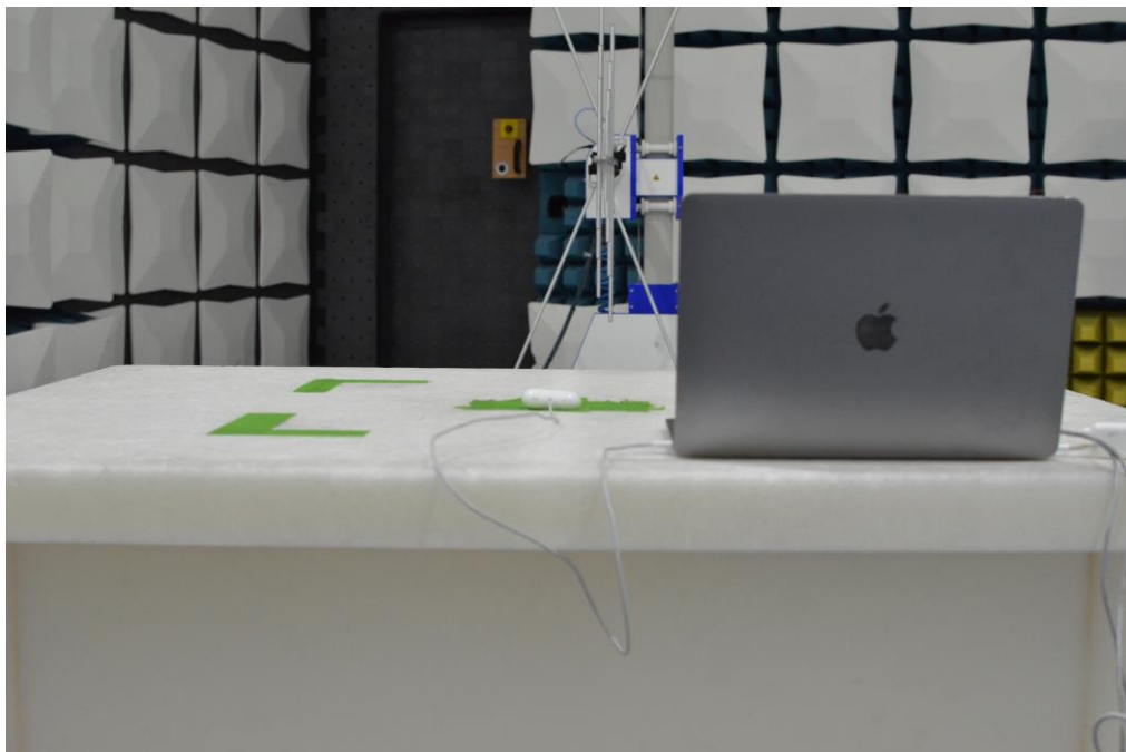
Figure 18: 30MHz-1GHz Test Setup (Rear View)
