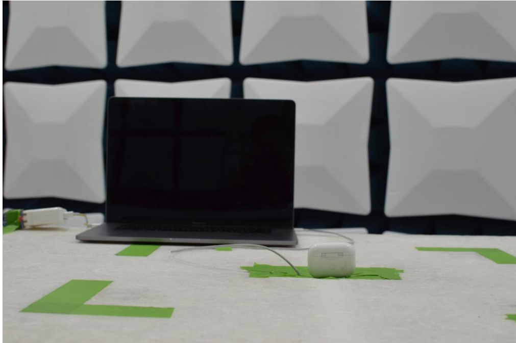
Figure 21: 30MHz-1GHz Test Setup (Front View)
