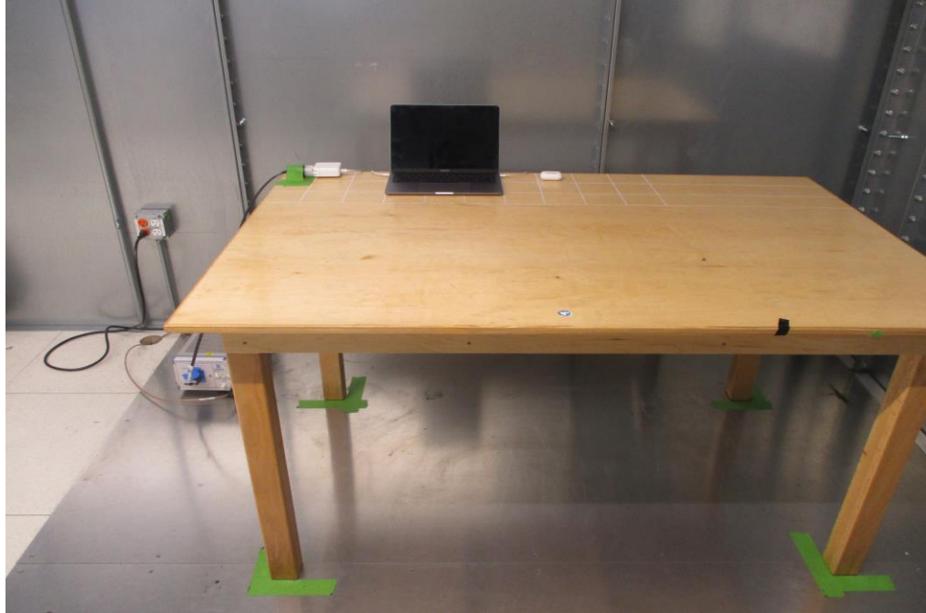
Figure 3: AC Line Conducted Emissions (Front View)
