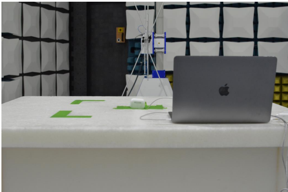
Figure 22: 30MHz-1GHz Test Setup (Rear View)
