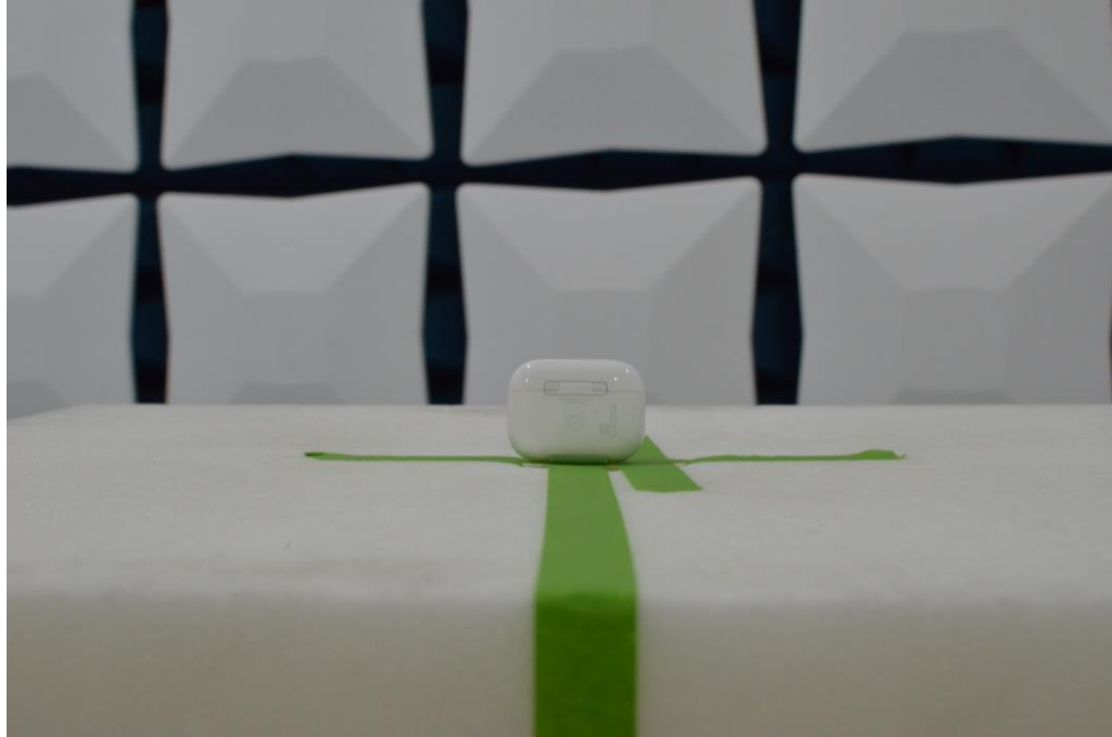
Figure 9: 1-18GHz Test Setup (Front View)
