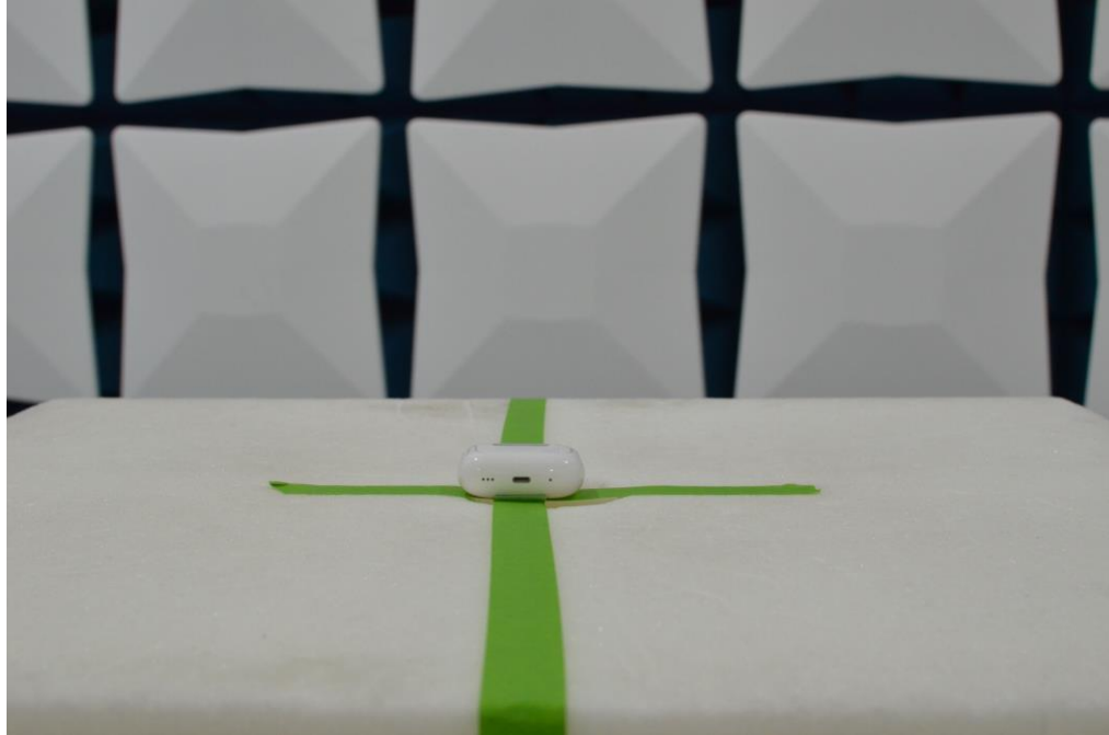
Figure 5: 1-18GHz Test Setup (Front View)
