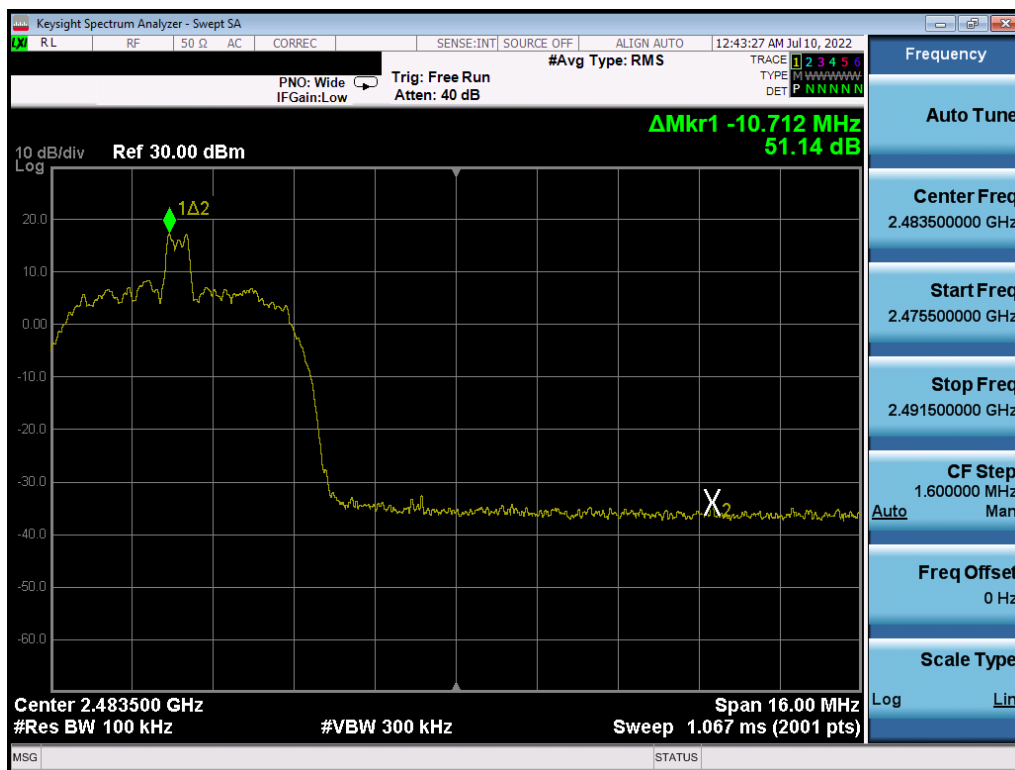
Plot 7-28. Band Edge Plot (Bluetooth (HDR8) – Ch. 75)
