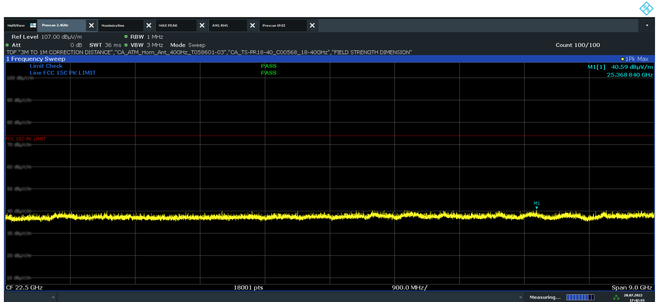
Plot 7-43. Radiated Spurious Emissions Above 18GHz V Polarity (4Mbps, HDR4 – Ch. 75)
