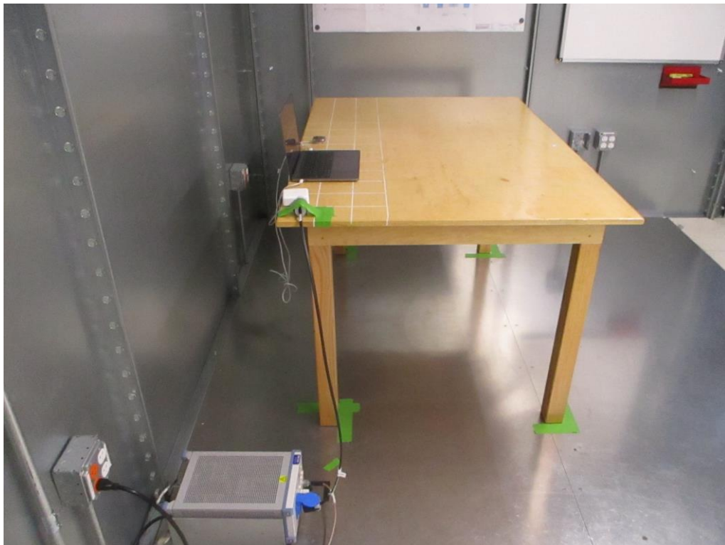
Figure 4: AC Line Conducted Emissions (Side View)
