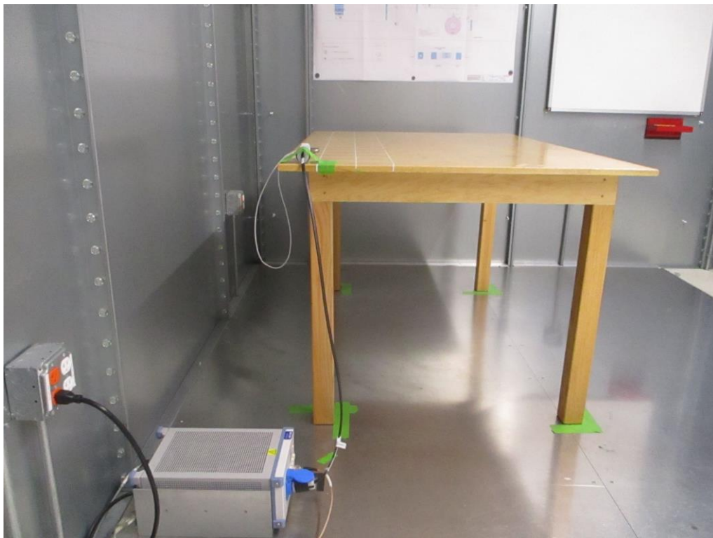
Figure 2: AC Line Conducted Emissions (Side View)
