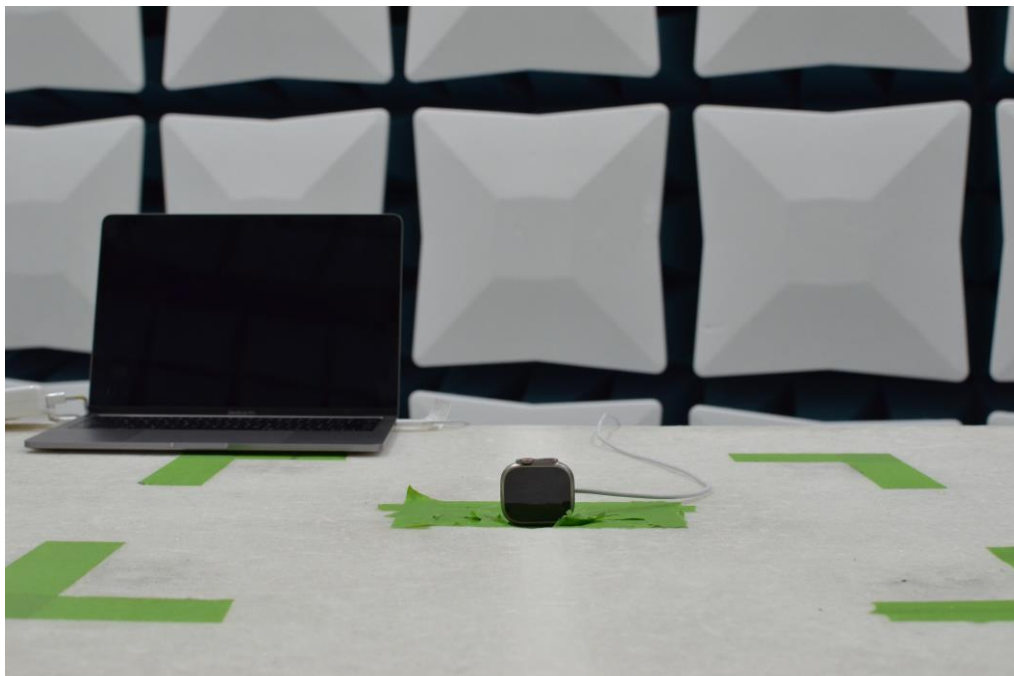
Figure 19: 30MHz-1GHz Test Setup (Front View)
