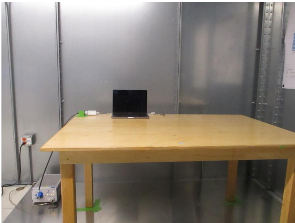
Figure 3: AC Line Conducted Emissions (Front View)
