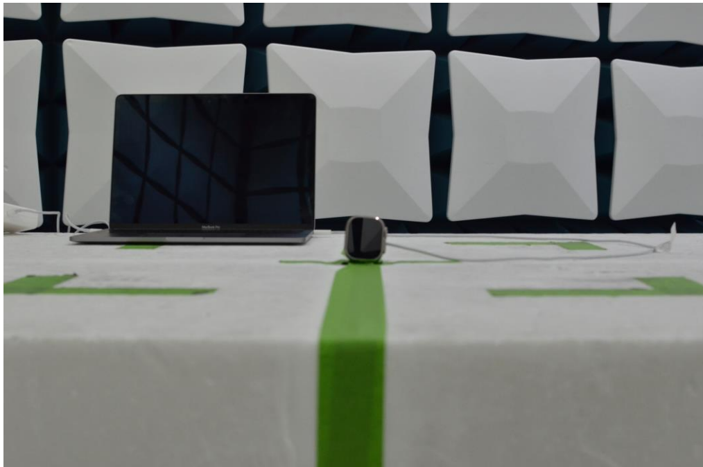
Figure 21: 30MHz-1GHz Test Setup (Front View)
