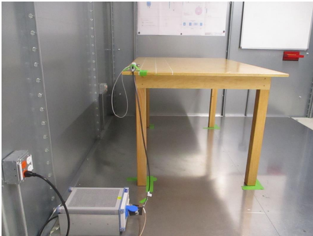
Figure 2: AC Line Conducted Emissions (Side View)
