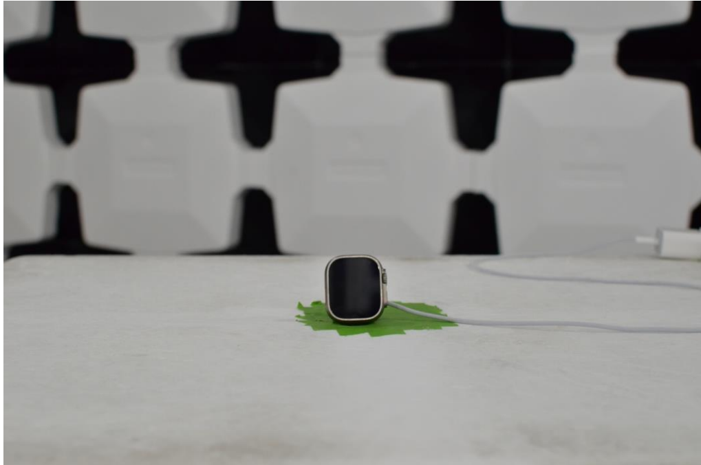
Figure 9: 1-18GHz Test Setup (Front View)
