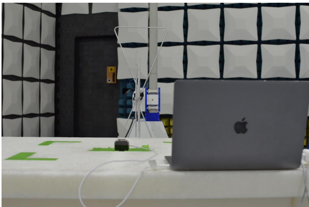
Figure 20: 30MHz-1GHz Test Setup (Rear View)
