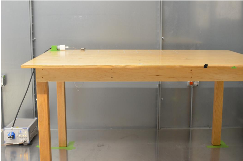
Figure 1: AC Line Conducted Emissions (Front View)
