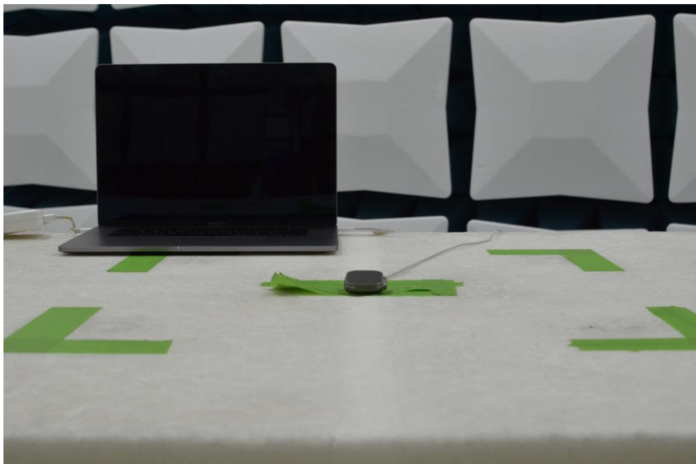
Figure 17: 30MHz-1GHz Test Setup (Front View)
