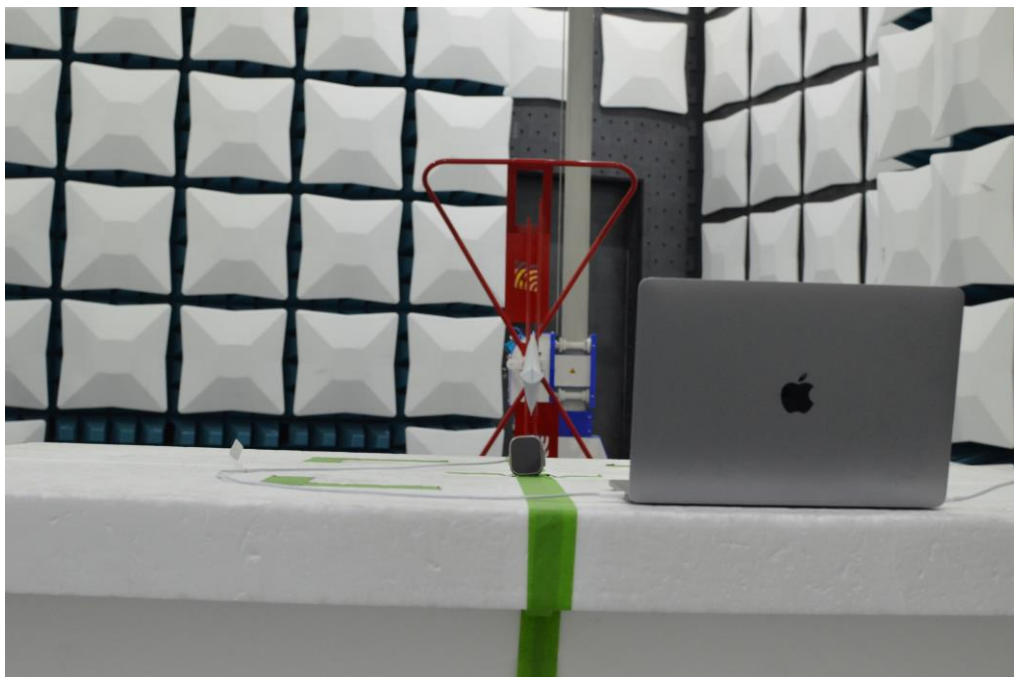
Figure 22: 30MHz-1GHz Test Setup (Rear View)
