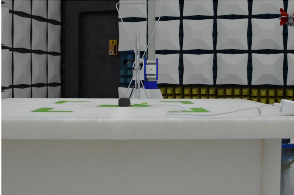
Figure 11: 30MHz-960MHz Test Setup (Rear View)
