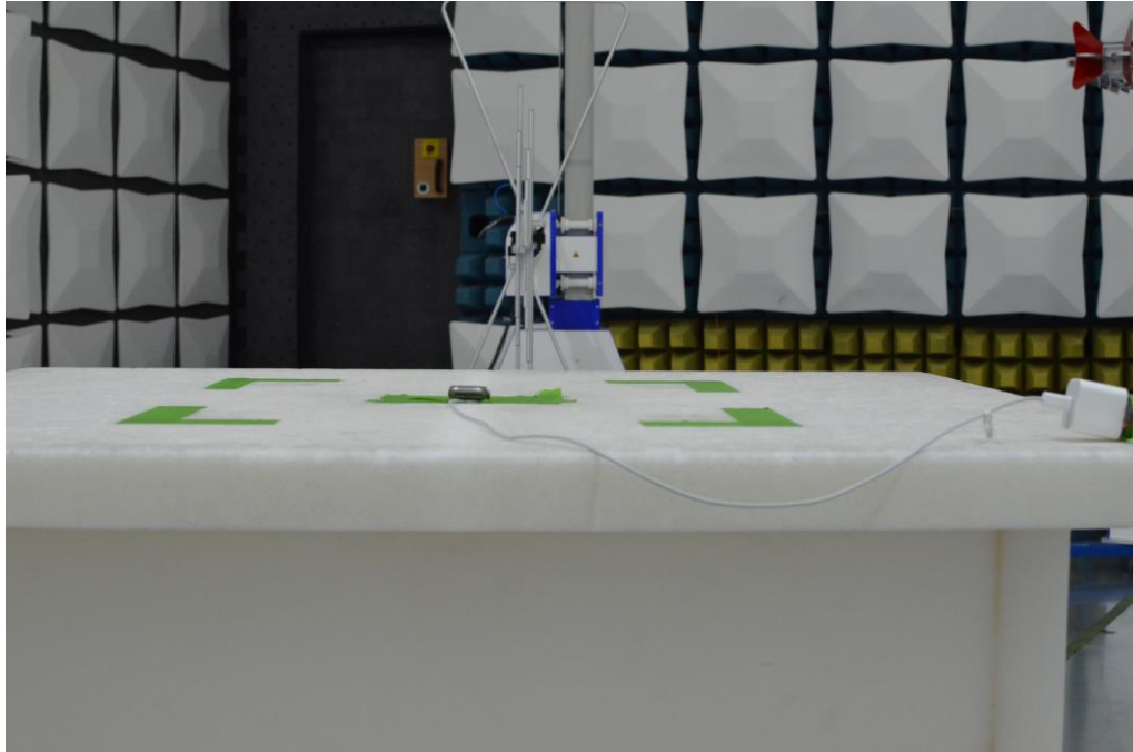
Figure 9: 30MHz-960MHz Test Setup (Rear View)
