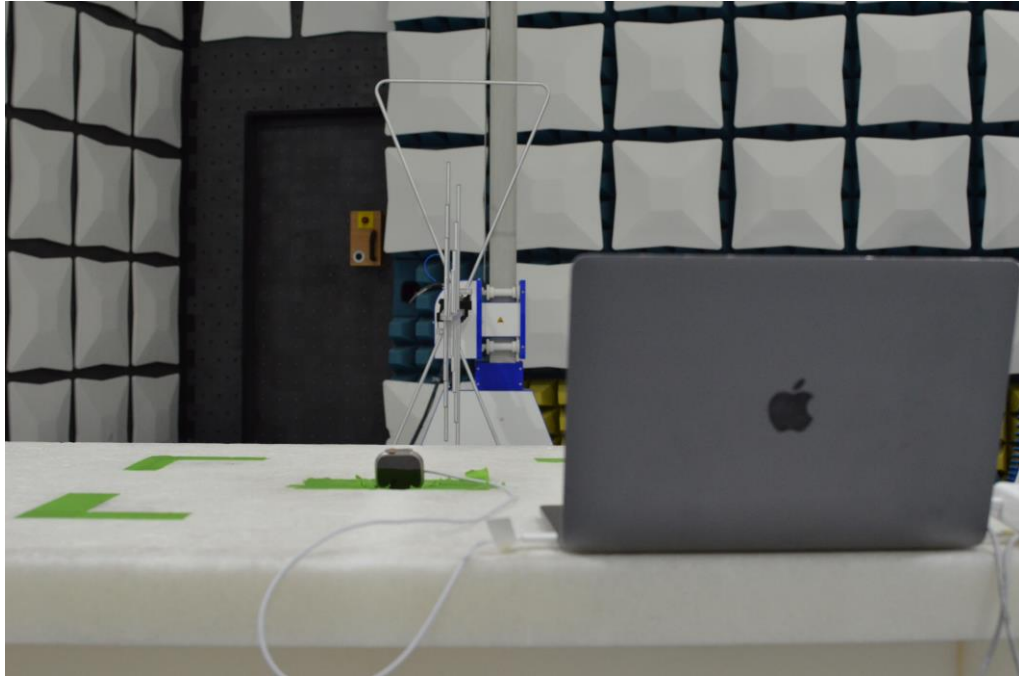
Figure 17: 30MHz-960MHz Test Setup (Rear View)
