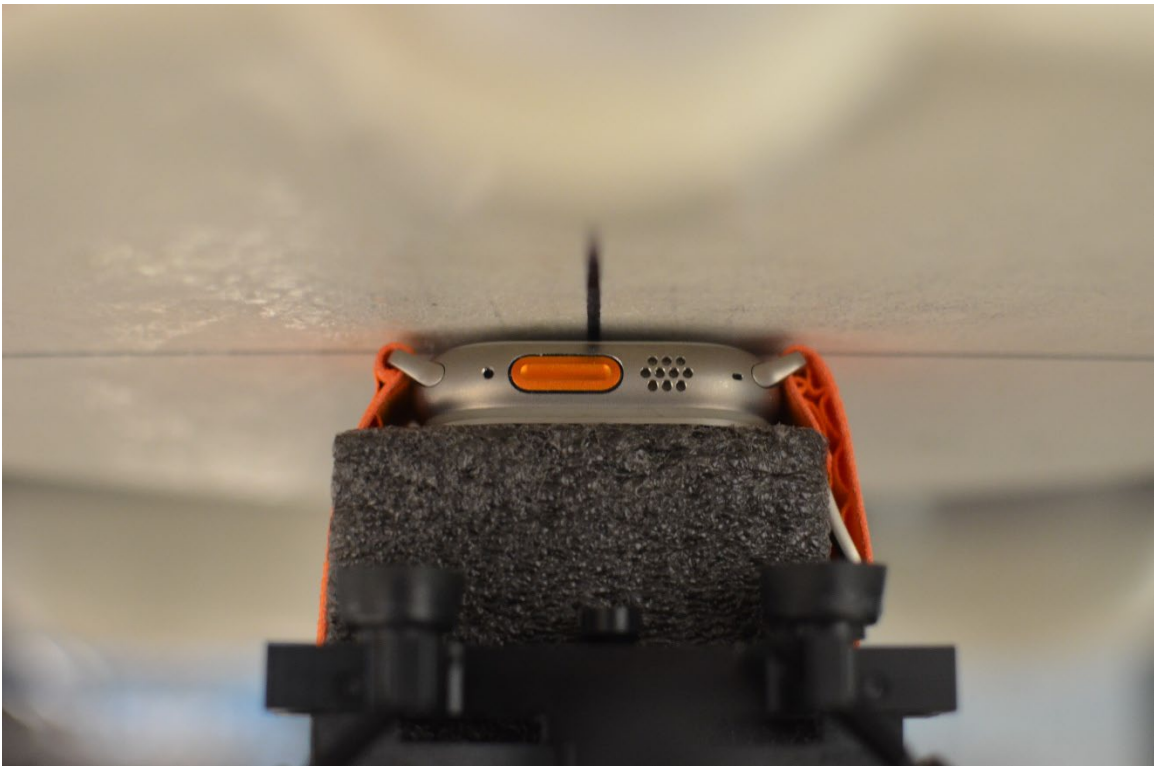
SAR Test Setup Photo 4: Titanium with Fabric Wristband, Extremity, Back Side at 0.0 cm
