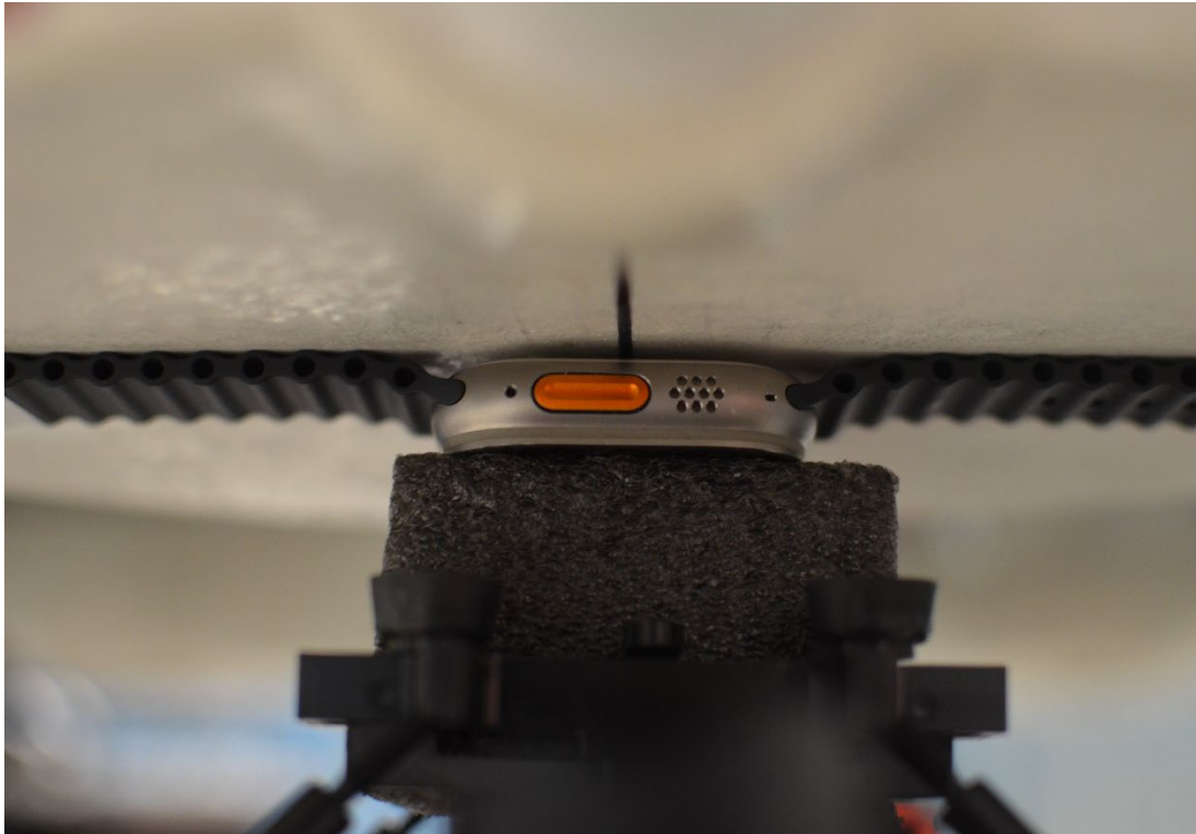
SAR Test Setup Photo 3: Titanium with Sport Wristband, Extremity, Back Side at 0.0 cm
