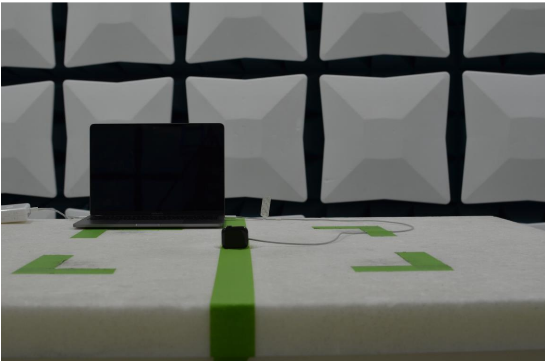
Figure 16: 30MHz-960MHz Test Setup (Front View)
