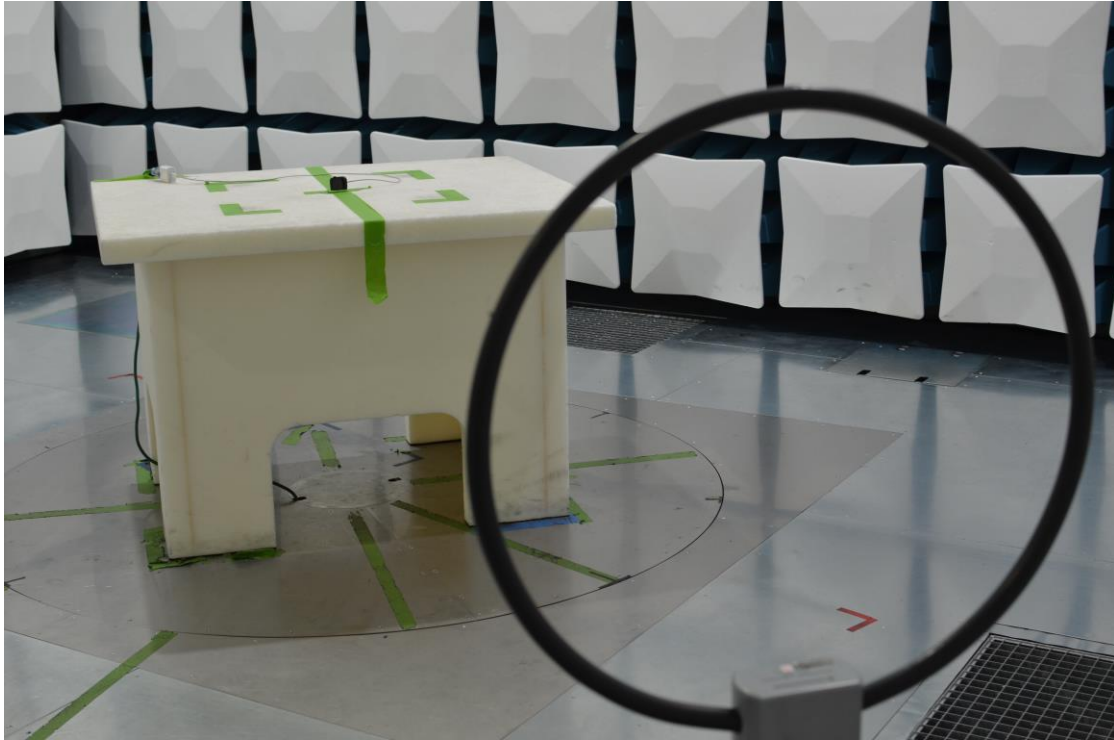
Figure 21: 9kHz-30MHz Test Setup (Front View)
