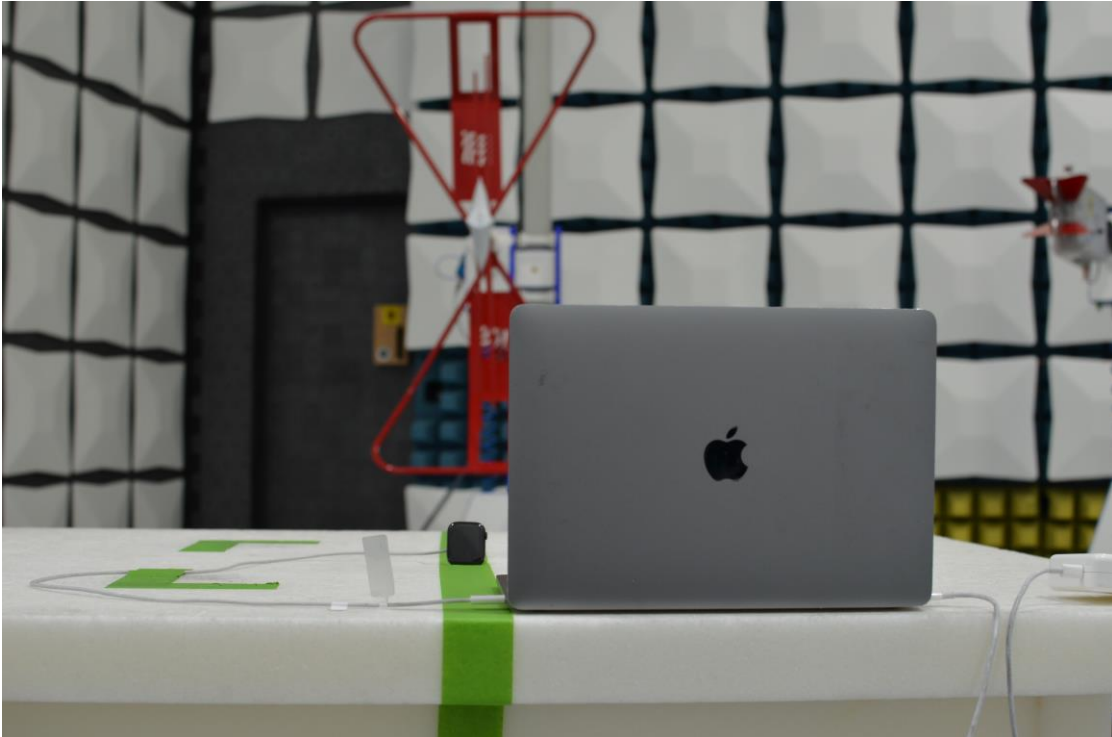
Figure 19: 30MHz-960MHz Test Setup (Rear View)
