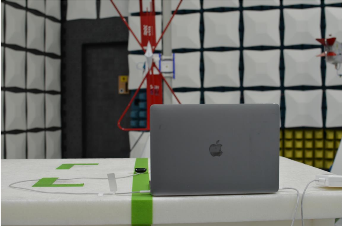
Figure 15: 30MHz-960MHz Test Setup (Rear View)
