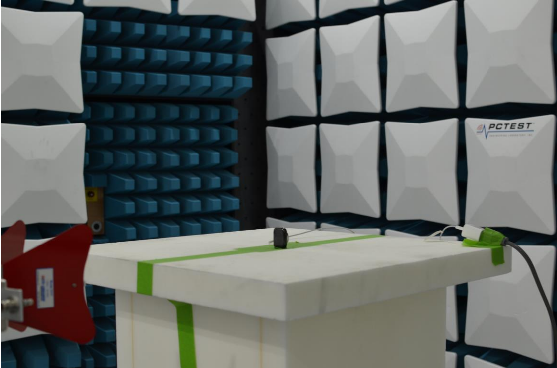
Figure 7: Above 960MHz Test Setup
