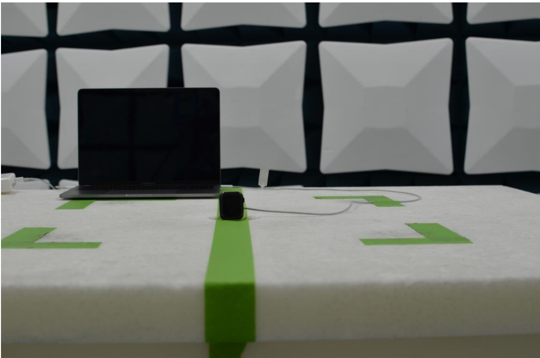
Figure 18: 30MHz-960MHz Test Setup (Front View)
