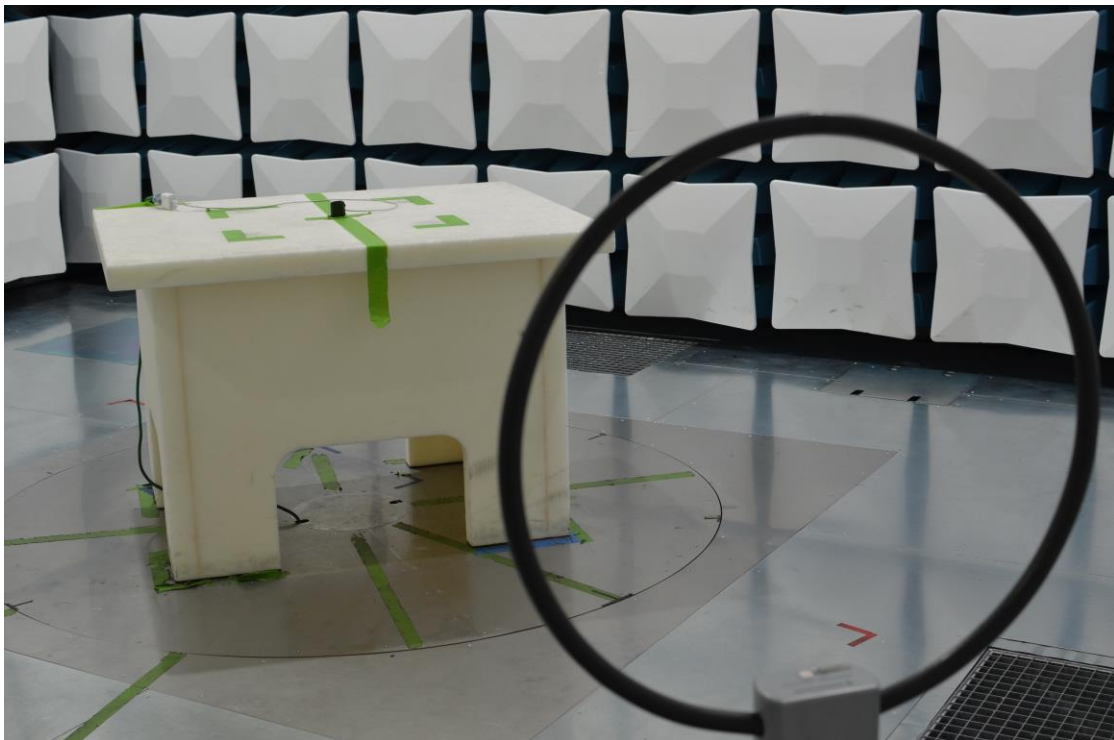
Figure 22: 9kHz-30MHz Test Setup (Front View)
