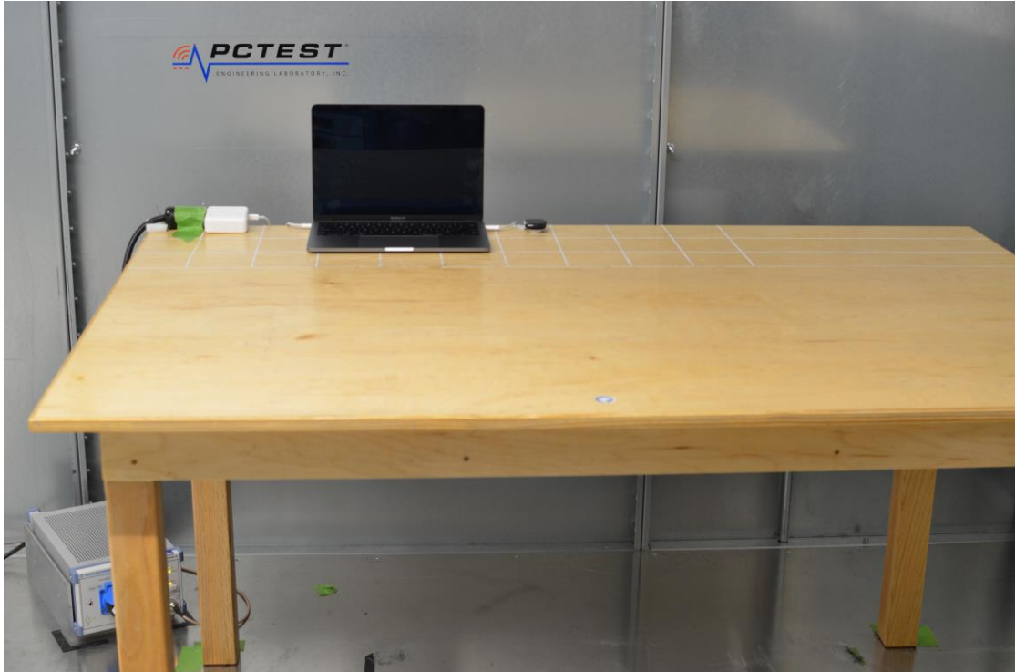
Figure 3: AC Line Conducted Emissions (Front View)
