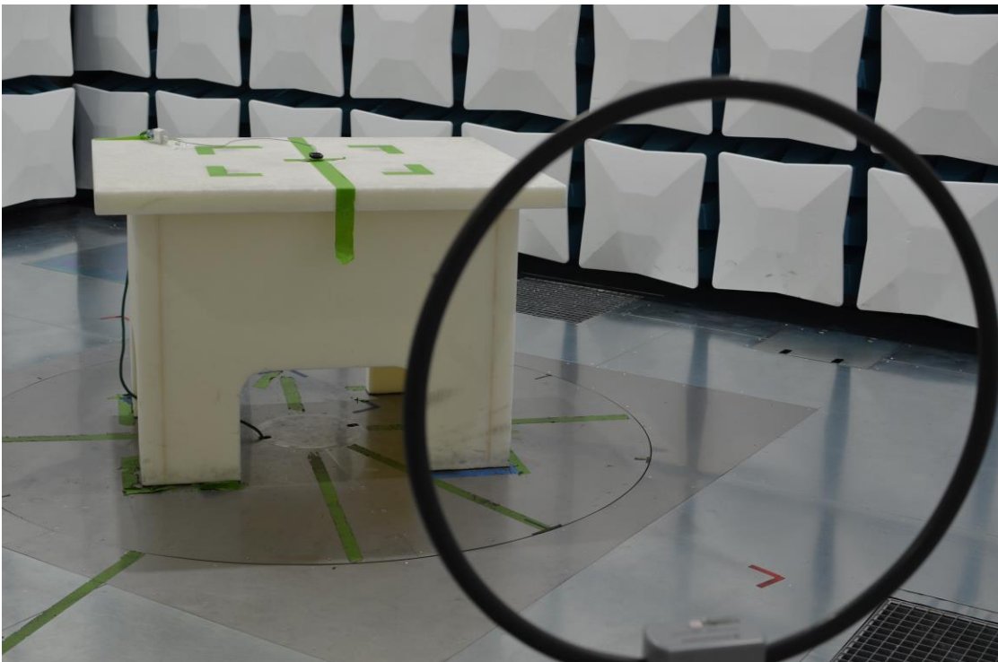
Figure 20: 9kHz-30MHz Test Setup (Front View)
