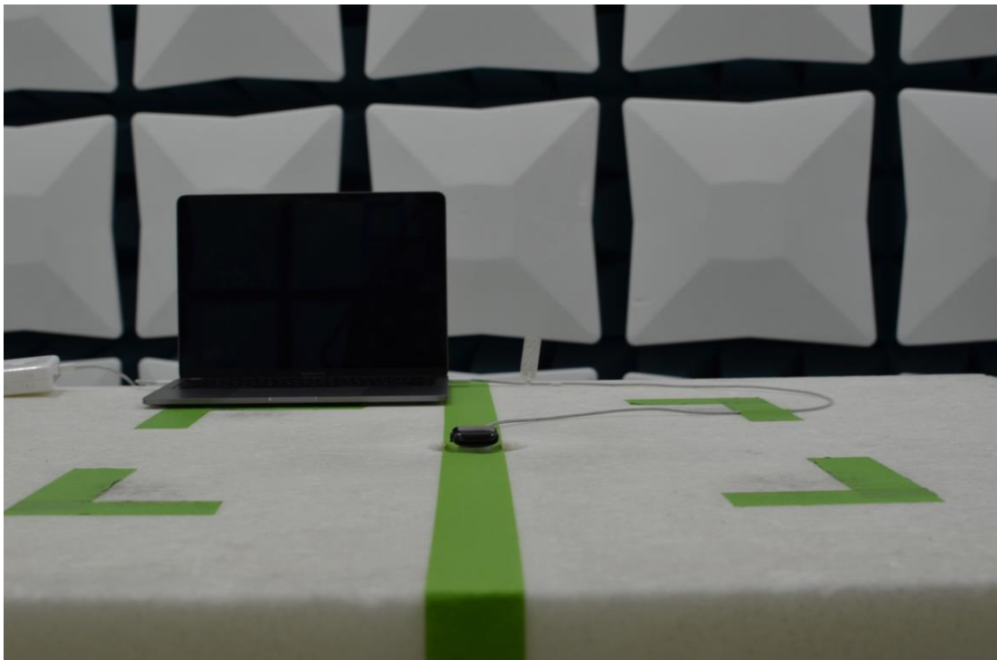
Figure 14: 30MHz-960MHz Test Setup (Front View)
