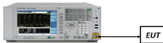
Figure 7-5. Test Instrument & Measurement Setup
