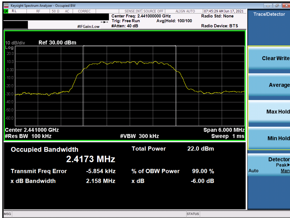
Plot 7-2. 6dB and 99% OBW Plot (Bluetooth (HDR4), 4Mbps, ePA – Ch. 38)
