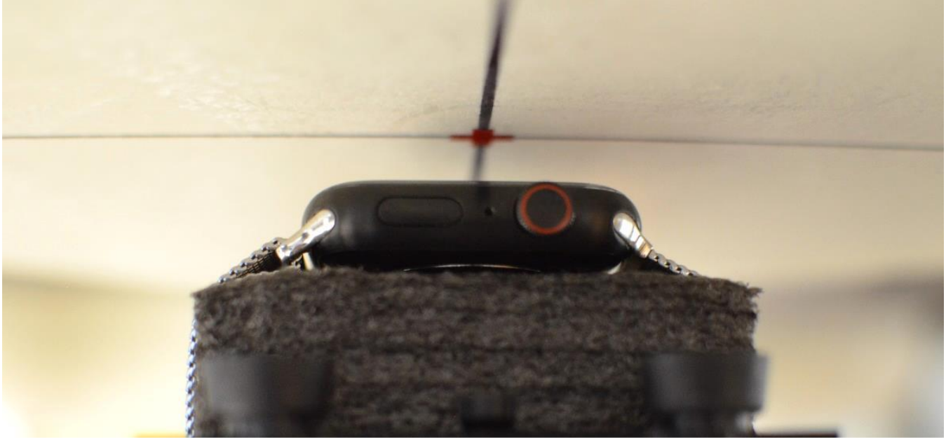
SAR Test Setup Photo 9: Titanium with Metal Loop Wristband, Head, Front Side at 1.0 cm
