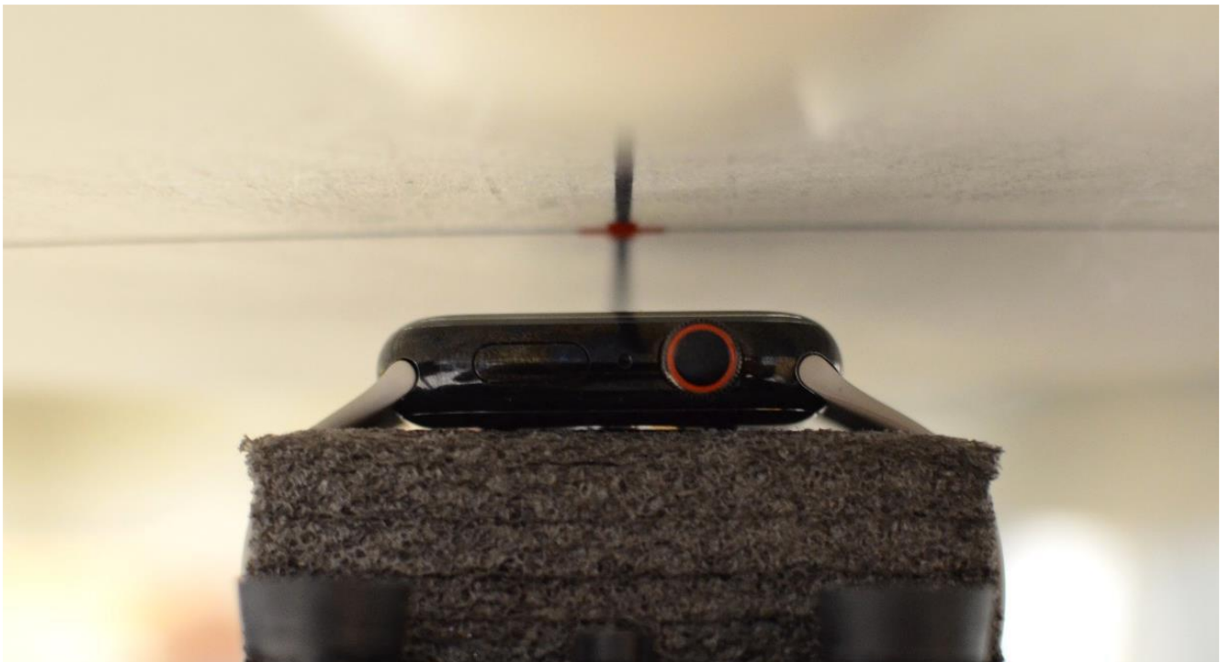
SAR Test Setup Photo 4: Stainless Steel with Sport Wristband, Head, Front Side at 1.0 cm
