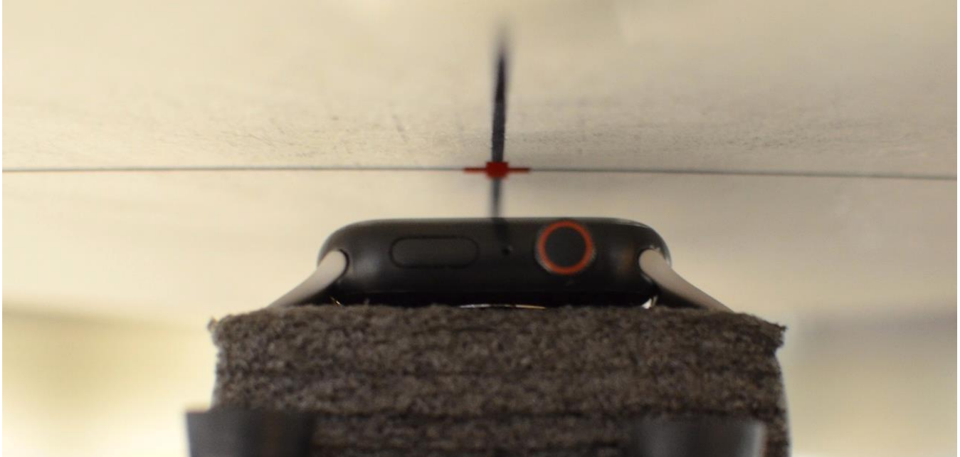
SAR Test Setup Photo 7: Titanium with Sport Wristband, Head, Front Side at 1.0 cm
