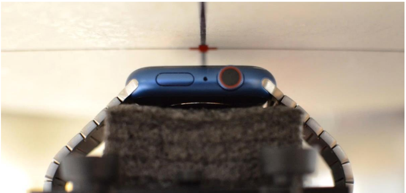
SAR Test Setup Photo 2: Aluminum with Metal Links Wristband, Head, Front Side at 1.0 cm
