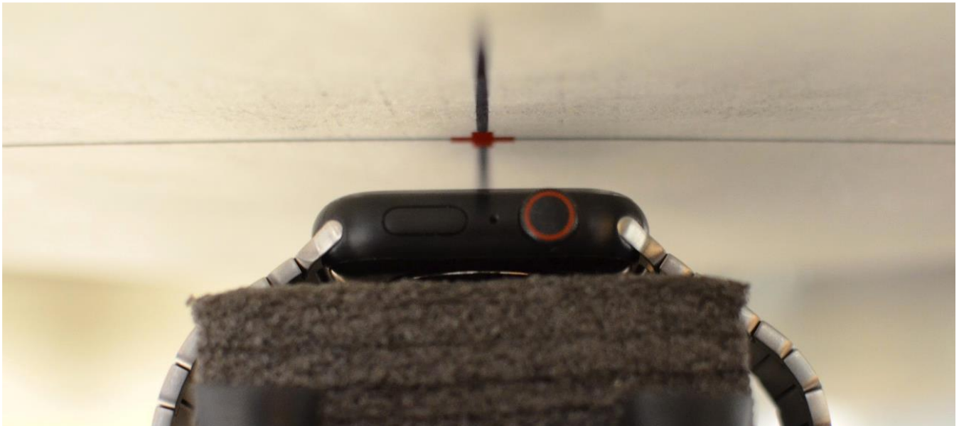
SAR Test Setup Photo 8: Titanium with Metal Links Wristband, Head, Front Side at 1.0 cm
