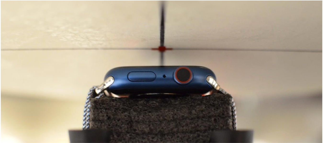
SAR Test Setup Photo 3: Aluminum with Metal Loop Wristband, Head, Front Side at 1.0 cm
