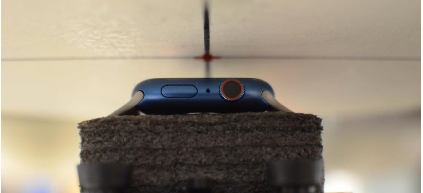
SAR Test Setup Photo 1: Aluminum with Sport Wristband, Head, Front Side at 1.0 cm
