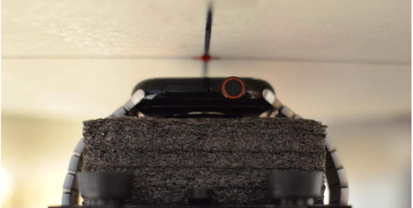
SAR Test Setup Photo 5: Stainless Steel with Metal Links Wristband, Head, Front Side at 1.0 cm
