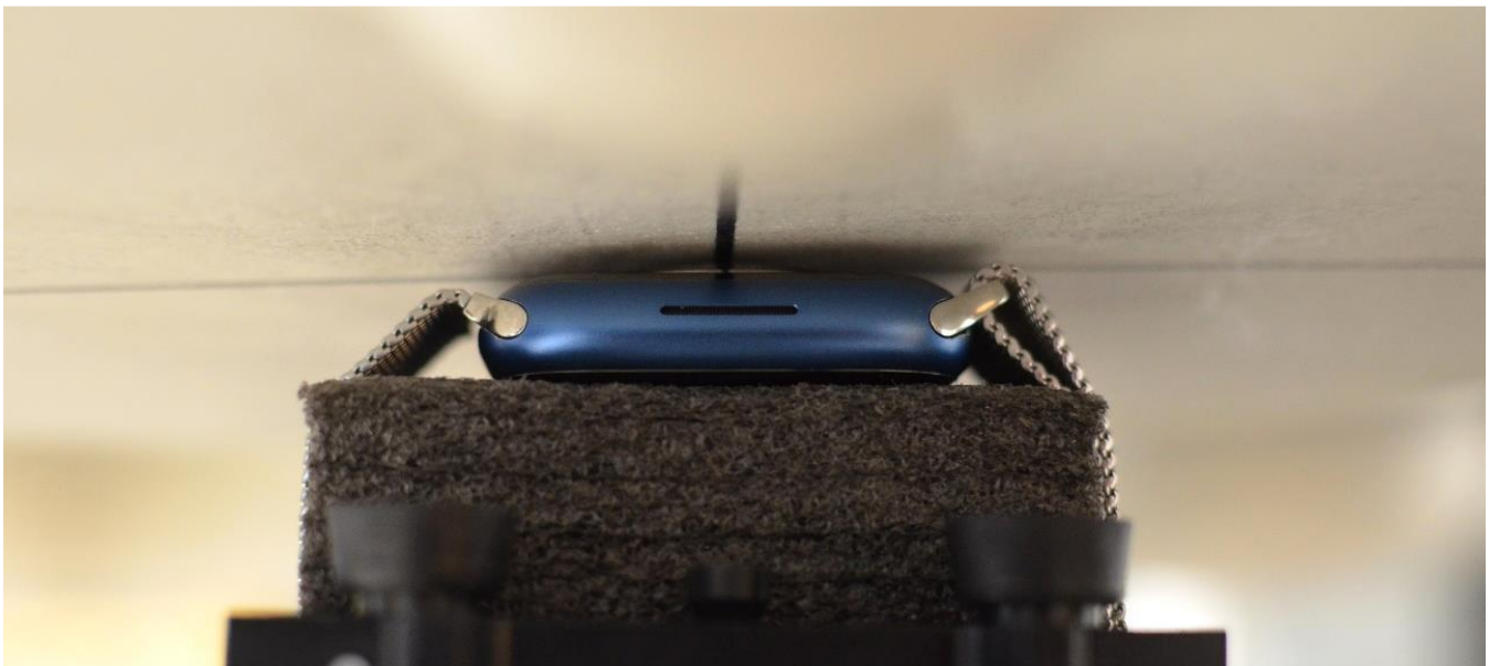
SAR Test Setup Photo 12: Aluminum with Metal Loop Wristband, Extremity, Back Side at 0.0 cm
