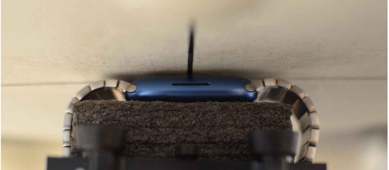
SAR Test Setup Photo 11: Aluminum with Metal Links Wristband, Extremity, Back Side at 0.0 cm
