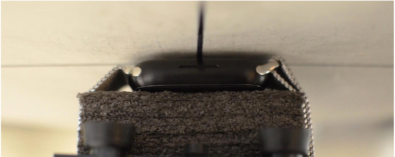
SAR Test Setup Photo 18: Titanium with Metal Loop Wristband, Extremity, Back Side at 0.0 cm
