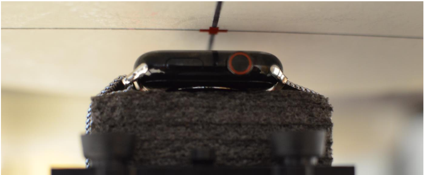
SAR Test Setup Photo 6: Stainless Steel with Metal Loop Wristband, Head, Front Side at 1.0 cm
