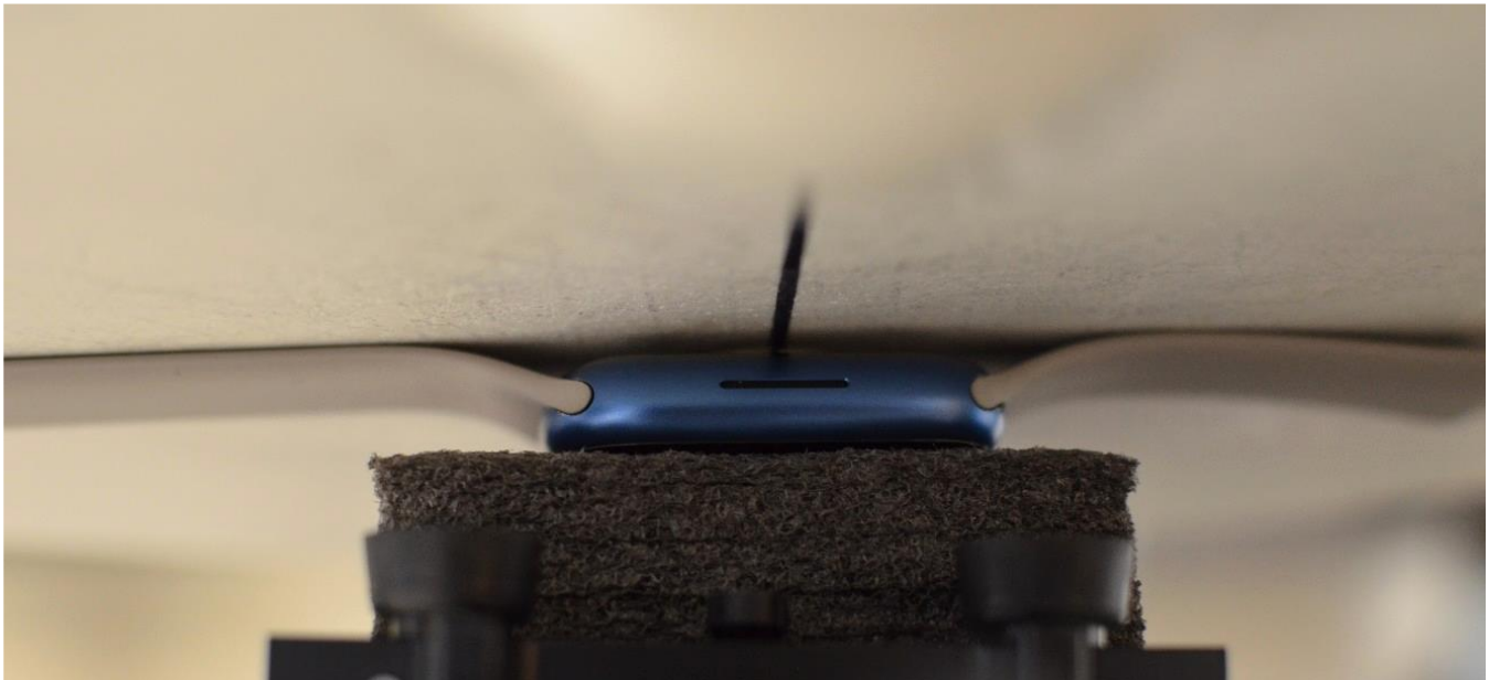
SAR Test Setup Photo 10: Aluminum with Sport Wristband, Extremity, Back Side at 0.0 cm
