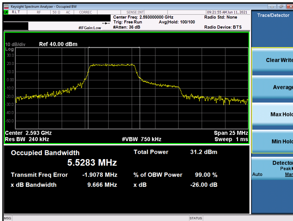
Plot 7-12. Occupied Bandwidth Plot (LTE Band 41 - 10MHz 16-QAM - Full RB)
