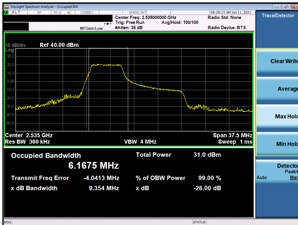
Plot 7-6. Occupied Bandwidth Plot (LTE Band 7 - 15MHz 16-QAM - Full RB)
