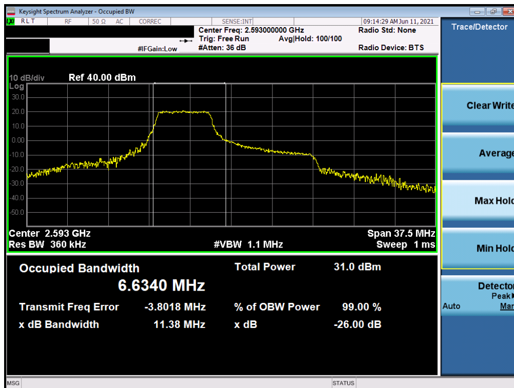
Plot 7-14. Occupied Bandwidth Plot (LTE Band 41 - 15MHz 16-QAM - Full RB)
