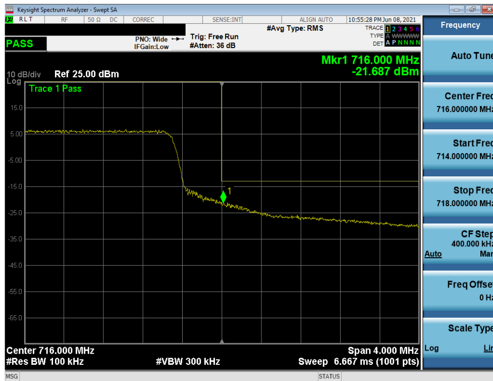
Plot 7-111. Upper Band Edge Plot (LTE Band 12 - 10MHz QPSK – Full RB)
