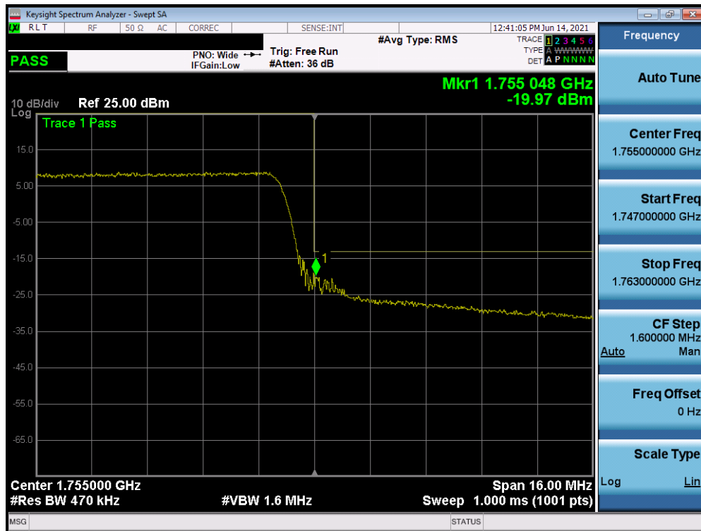
Plot 7-102. Upper Band Edge Plot (LTE Band 4 - 20MHz QPSK – Full RB)
