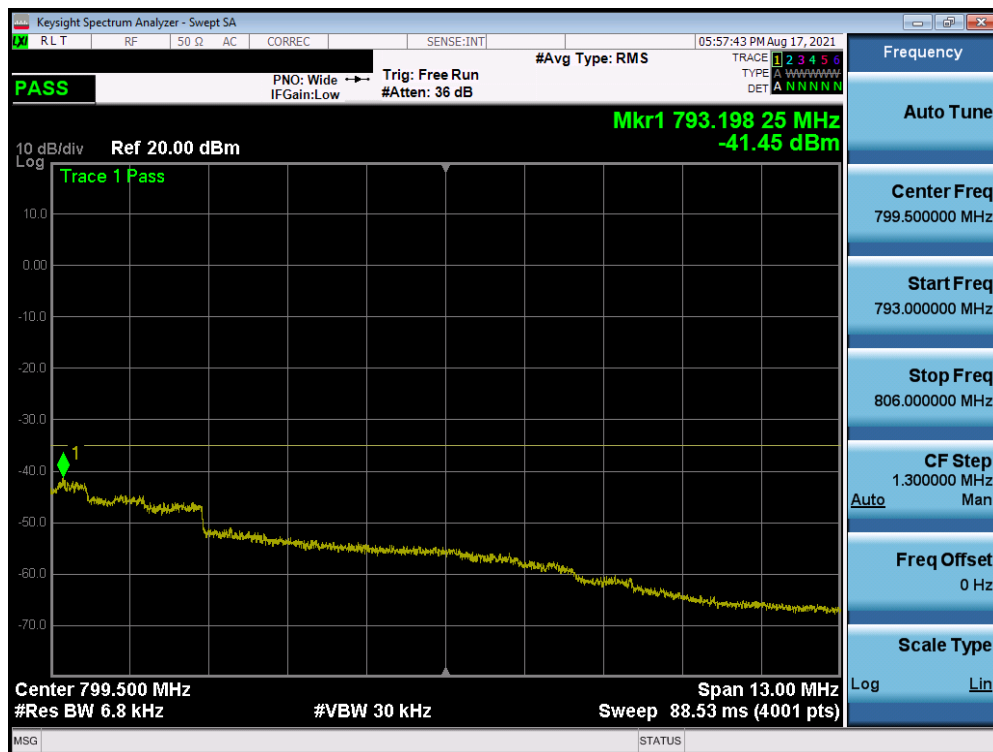
Plot 7-123. Upper Band Edge Plot (LTE Band 13 - 10MHz QPSK – Full RB)
