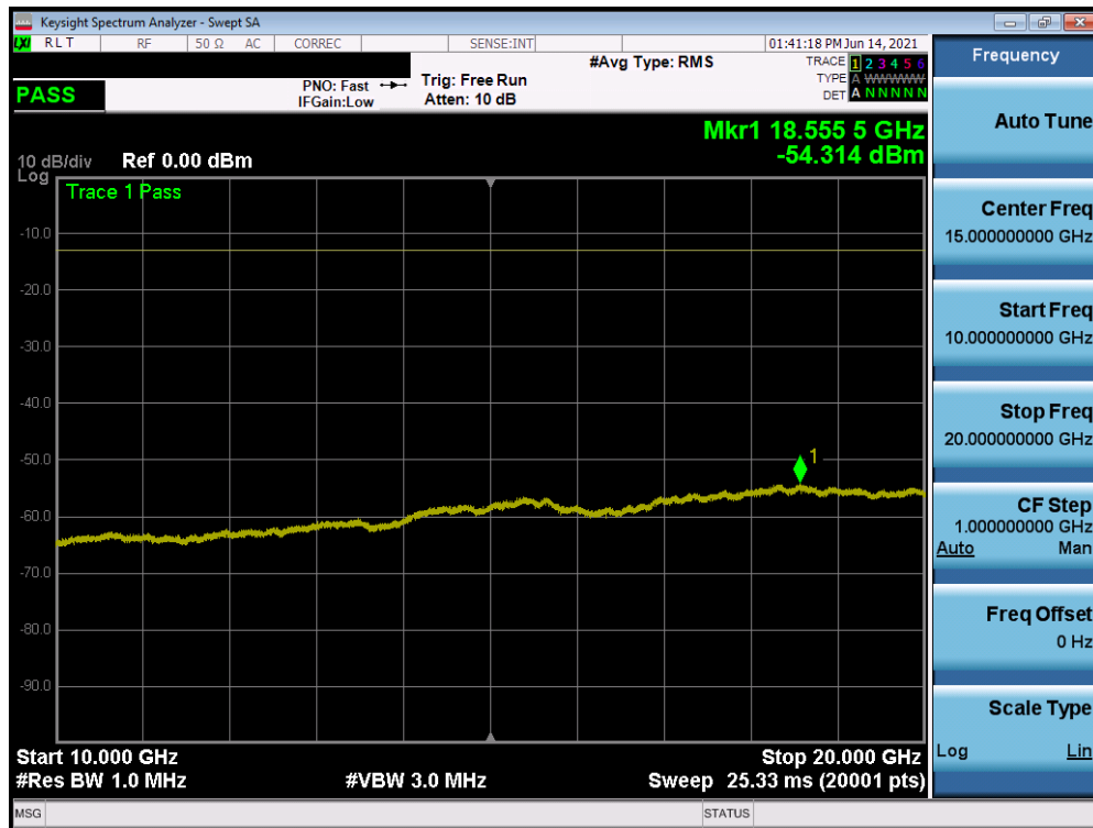
Plot 7-34. CSE (LTE Band 66/4 - 20MHz QPSK - RB Size 1, RB Offset 0 - High Channel)
