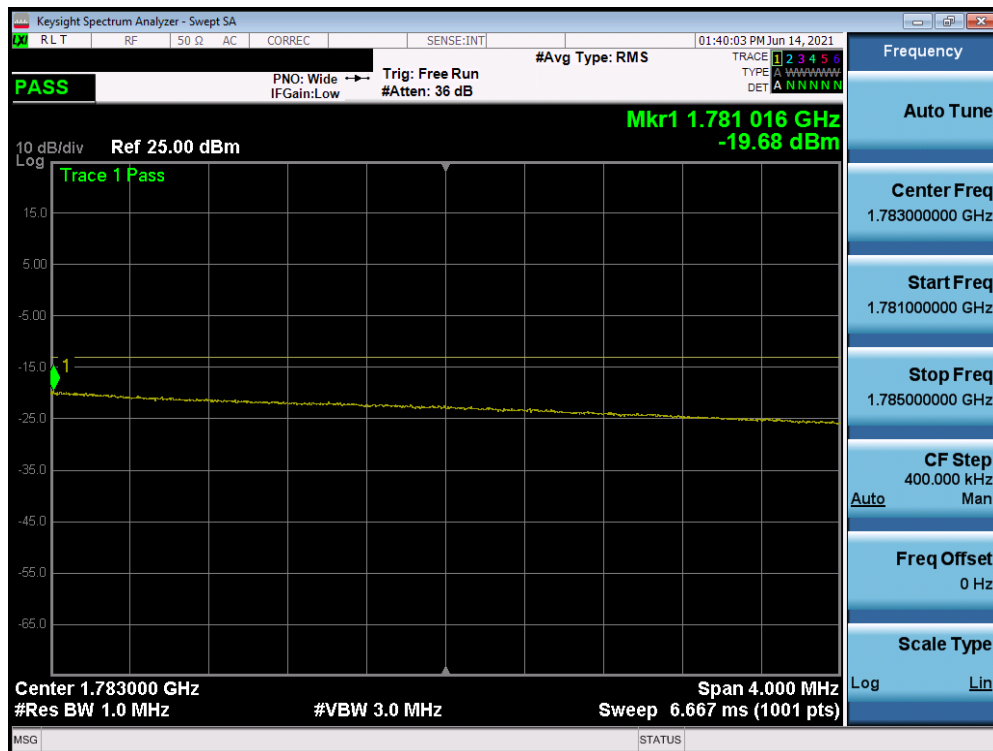
Plot 7-79. Upper Extended Band Edge Plot (LTE Band 66 - 20MHz QPSK – Full RB)
