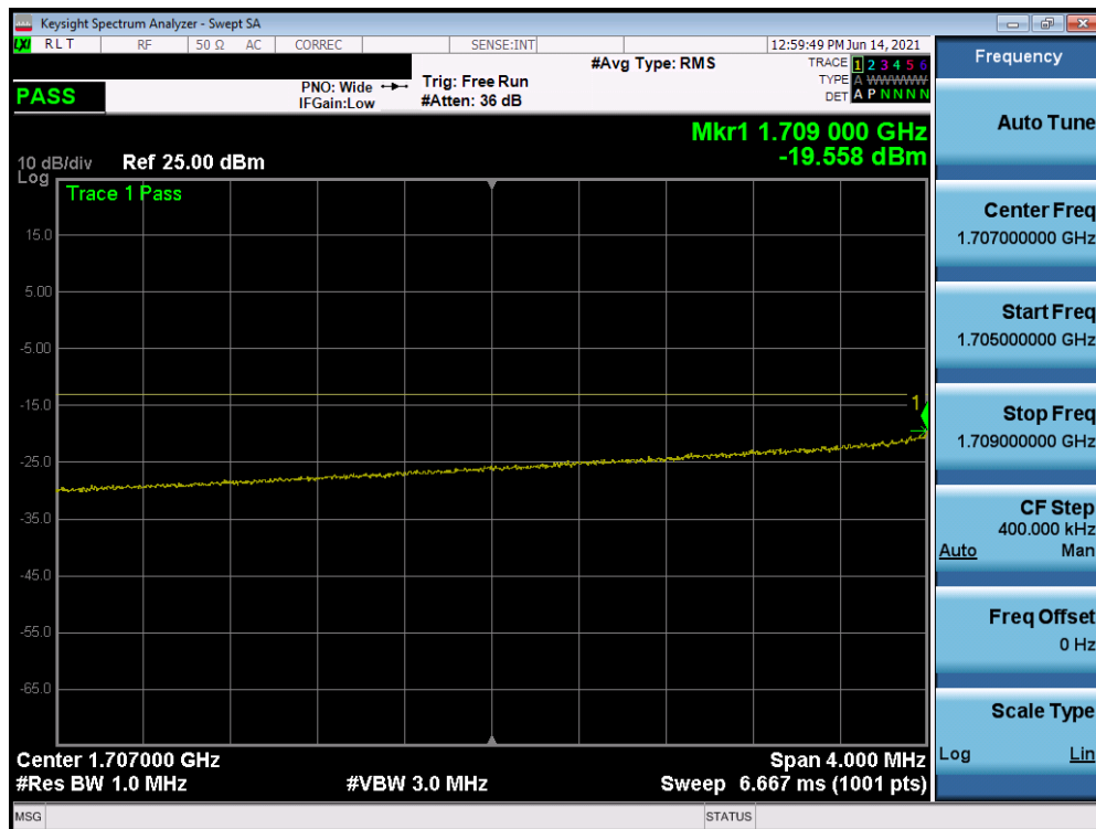
Plot 7-93. Lower Extended Band Edge Plot (LTE Band 4 - 10MHz QPSK – Full RB)
