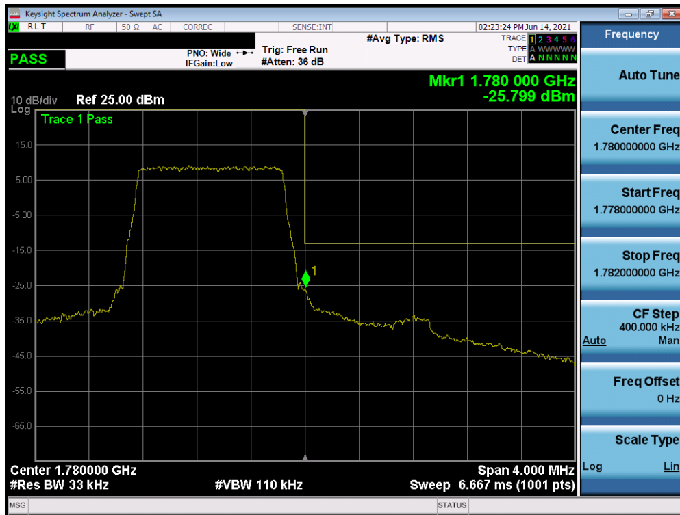
Plot 7-58. Upper Band Edge Plot (LTE Band 66 – 1.4MHz QPSK – Full RB)
