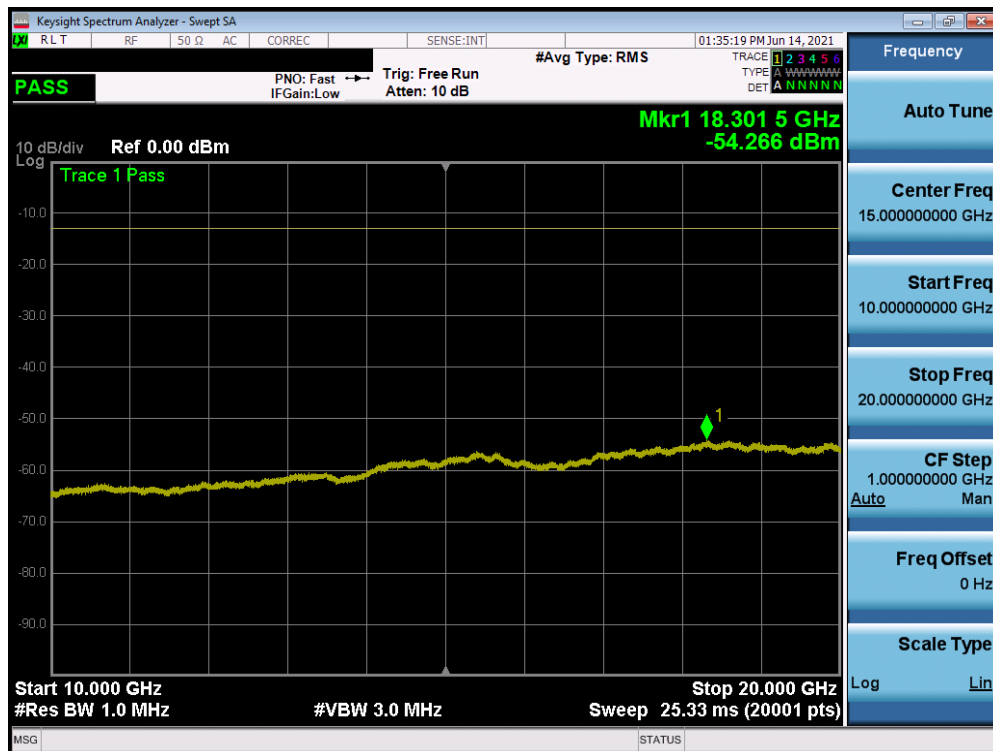
Plot 7-31. CSE (LTE Band 66/4 - 20MHz QPSK - RB Size 1, RB Offset 0 - Mid Channel)
