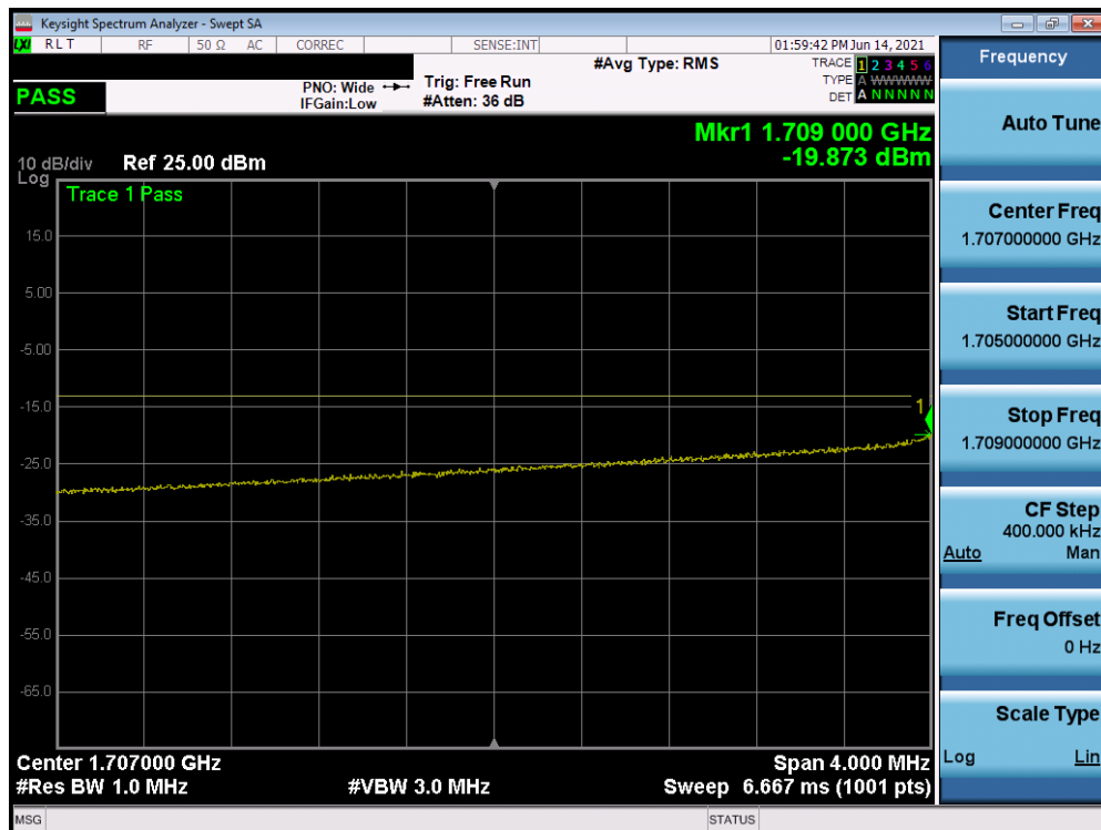
Plot 7-69. Lower Extended Band Edge Plot (LTE Band 66 - 10MHz QPSK – Full RB)
