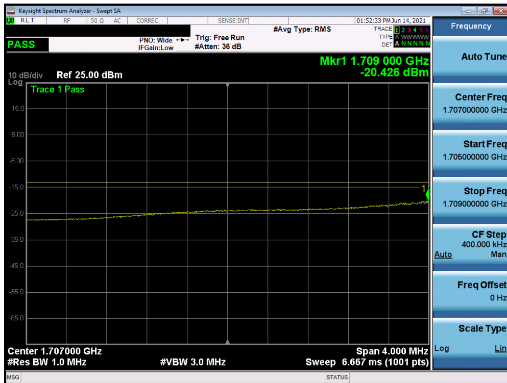
Plot 7-73. Lower Extended Band Edge Plot (LTE Band 66 - 15MHz QPSK – Full RB)
