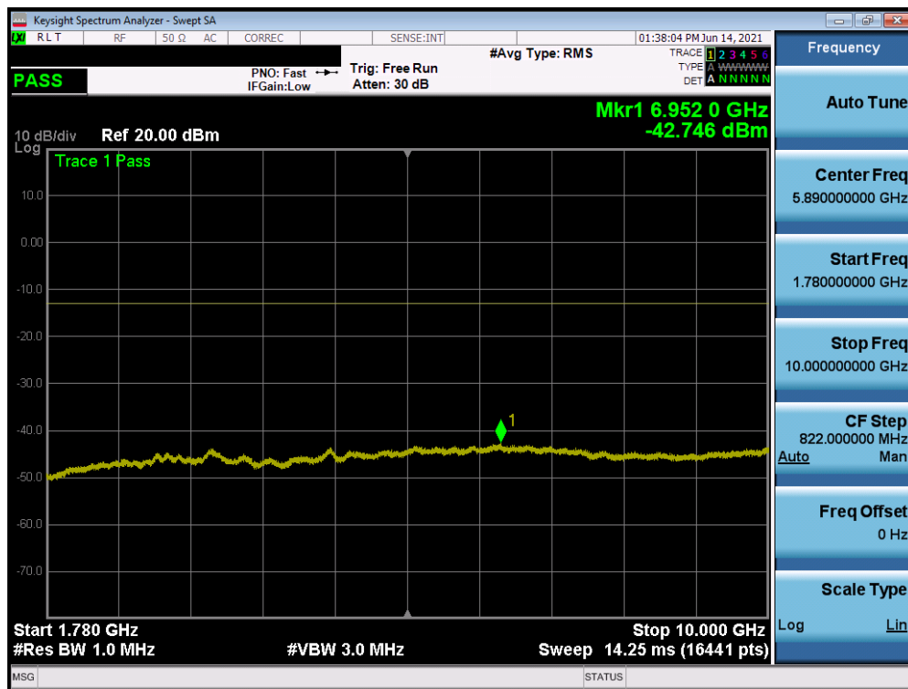
Plot 7-27. CSE (LTE Band 66/4 - 20MHz QPSK - RB Size 1, RB Offset 0 - Low Channel)
