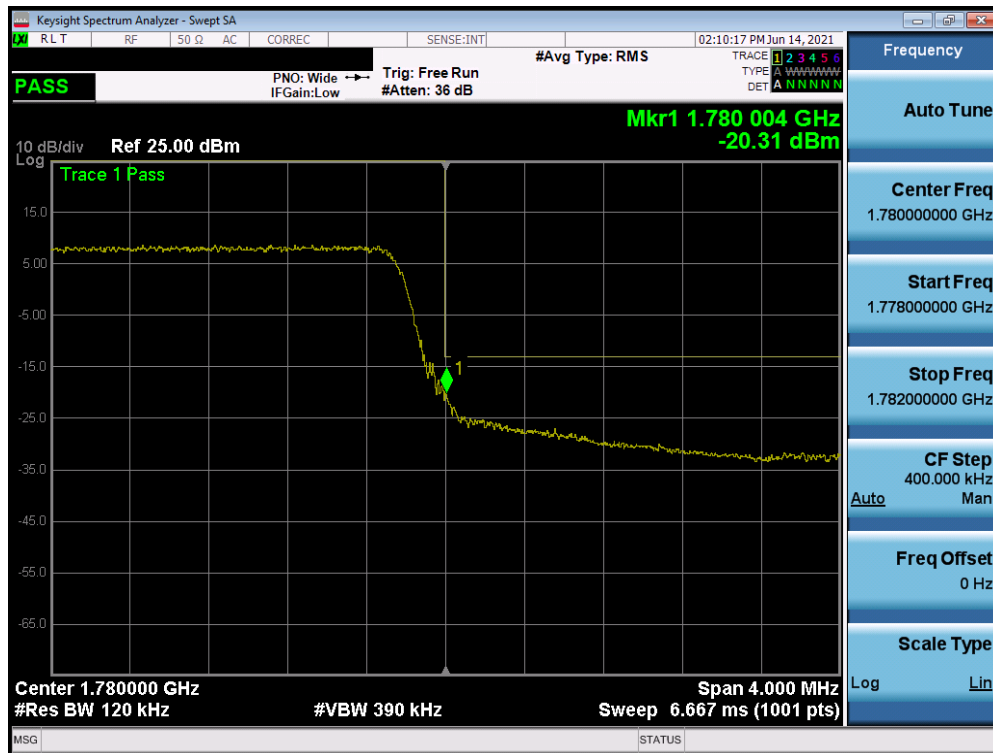
Plot 7-66. Upper Band Edge Plot (LTE Band 66 - 5MHz QPSK - Full RB)
