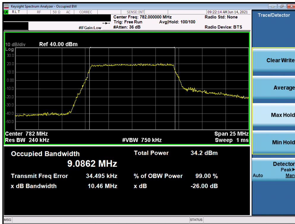
Plot 7-23. Occupied Bandwidth Plot (LTE Band 13 - 10MHz QPSK - Full RB)
