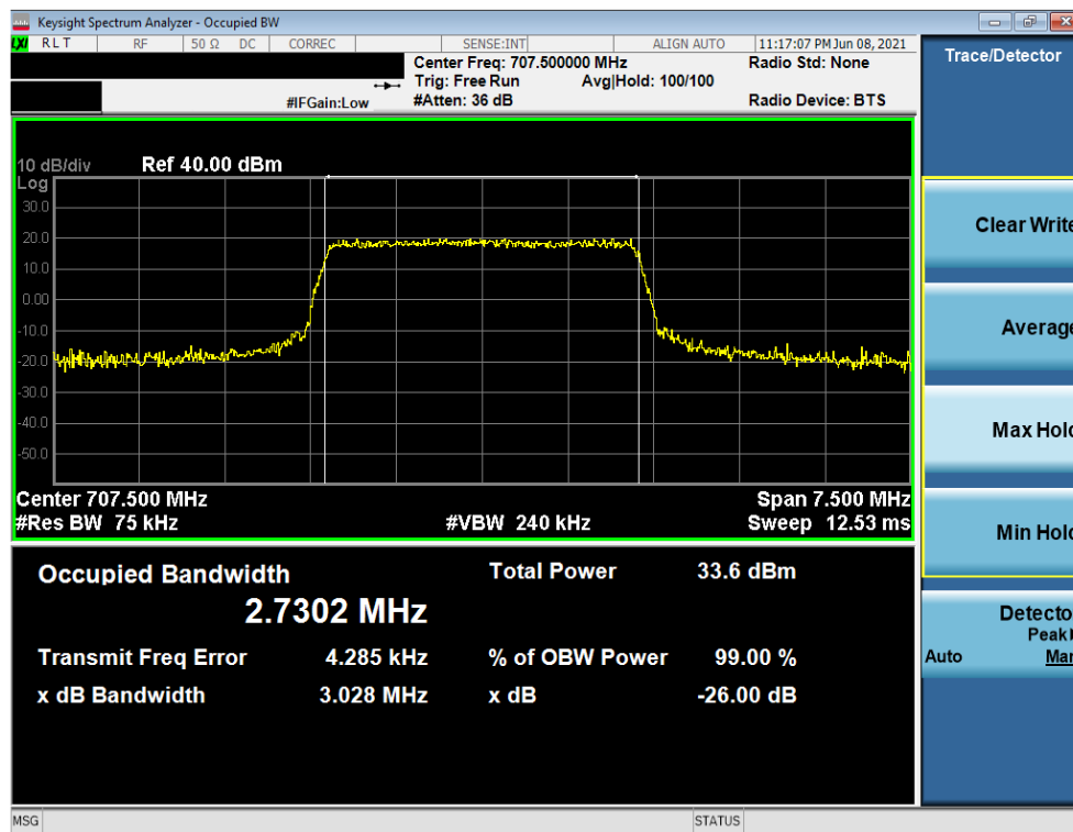
Plot 7-15. Occupied Bandwidth Plot (LTE Band 12 - 3MHz QPSK - Full RB)
