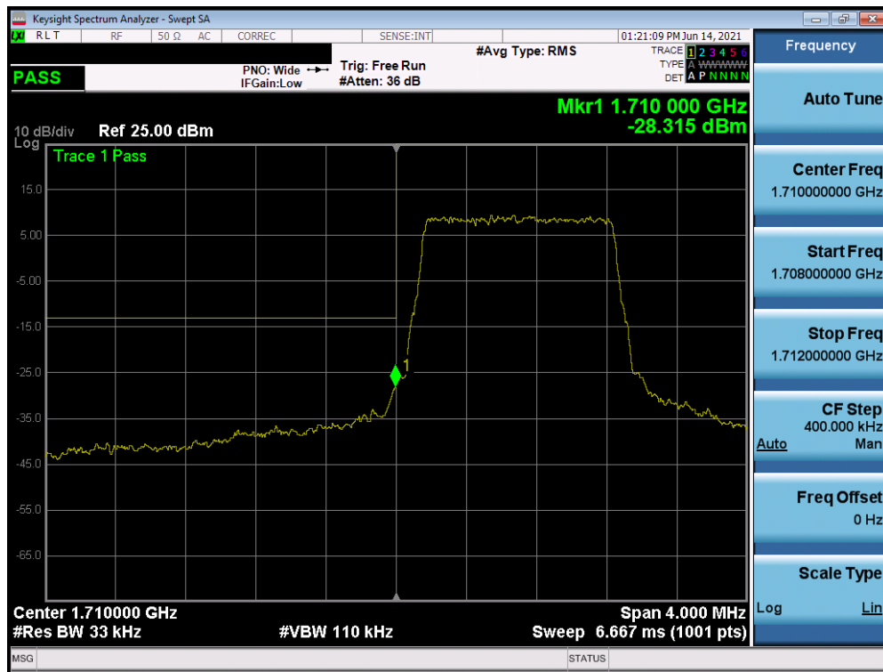
Plot 7-80. Lower Band Edge Plot (LTE Band 4 – 1.4MHz QPSK – Full RB)
