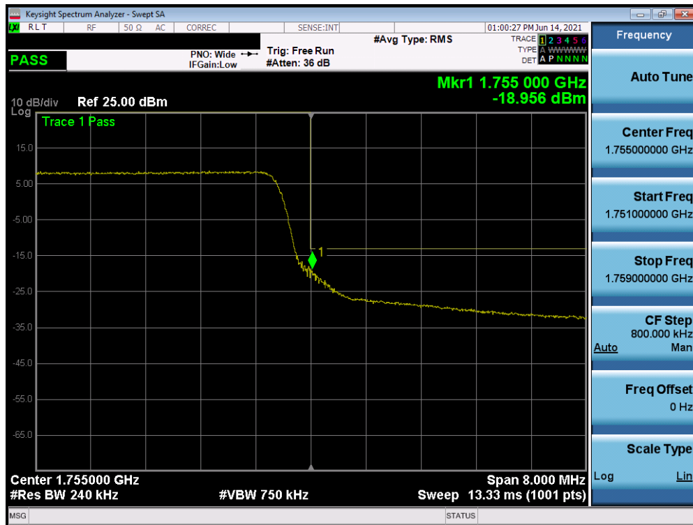
Plot 7-94. Upper Band Edge Plot (LTE Band 4 - 10MHz QPSK – Full RB)
