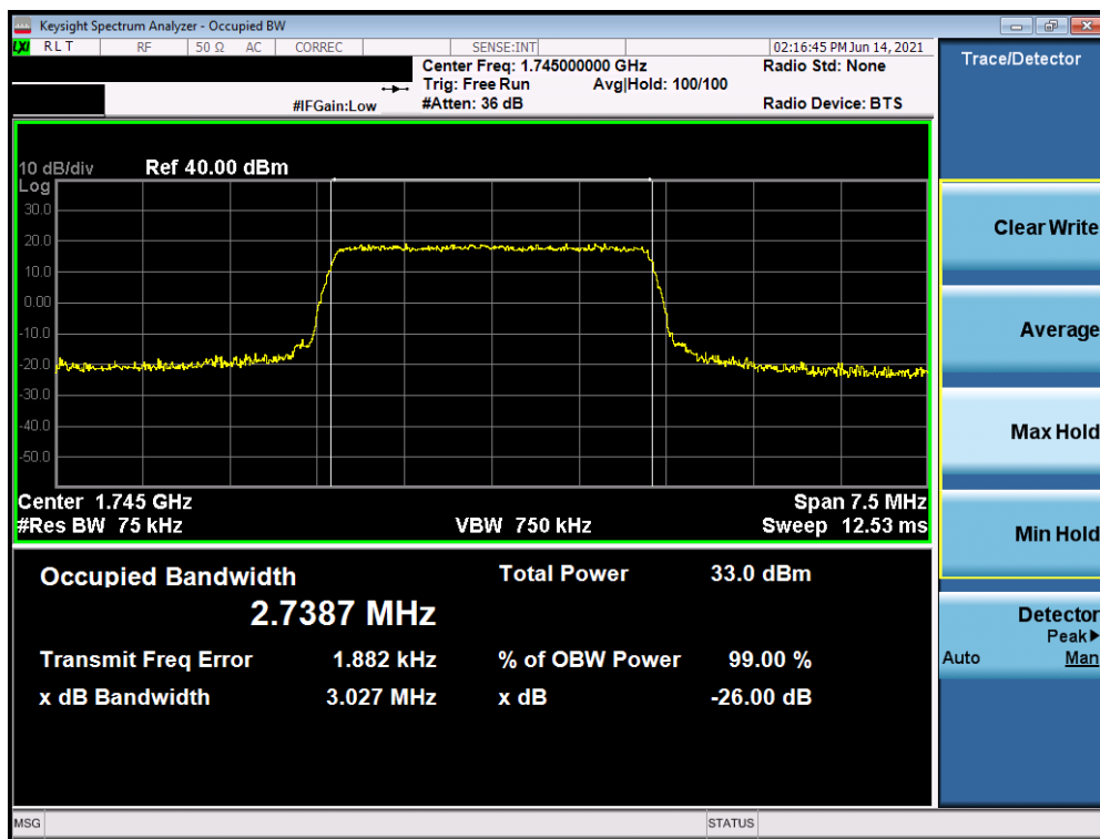
Plot 7-3. Occupied Bandwidth Plot (LTE Band 66/4 - 3MHz QPSK - Full RB)
