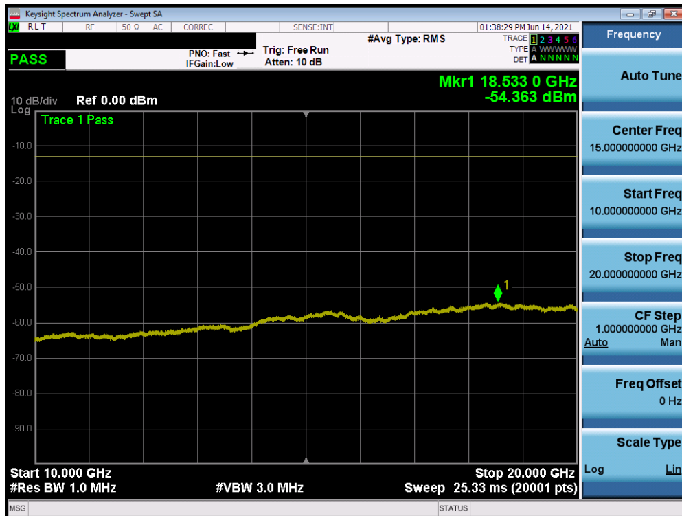
Plot 7-28. CSE (LTE Band 66/4 - 20MHz QPSK - RB Size 1, RB Offset 0 - Low Channel)
