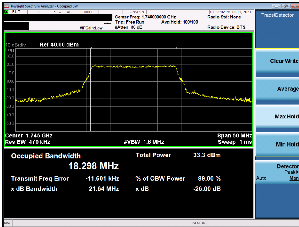
Plot 7-11. Occupied Bandwidth Plot (LTE Band 66/4 - 20MHz QPSK - Full RB)
