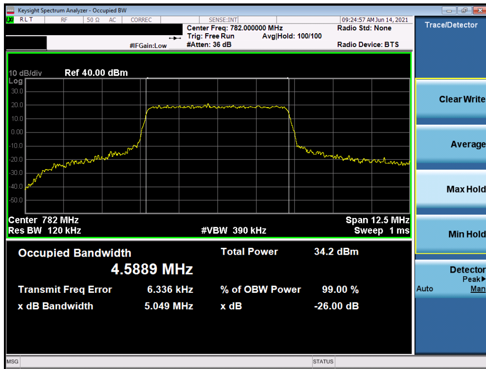
Plot 7-21. Occupied Bandwidth Plot (LTE Band 13 - 5MHz QPSK - Full RB)
