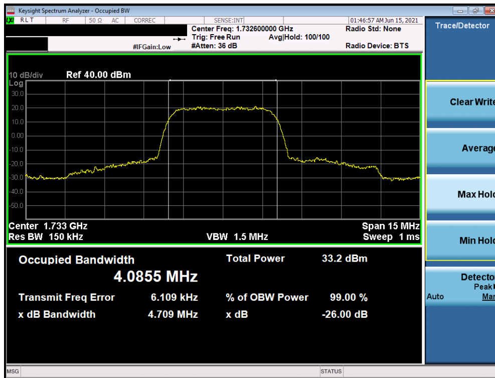
Plot 7-25. Occupied Bandwidth Plot (WCDMA, Ch. 1413)
