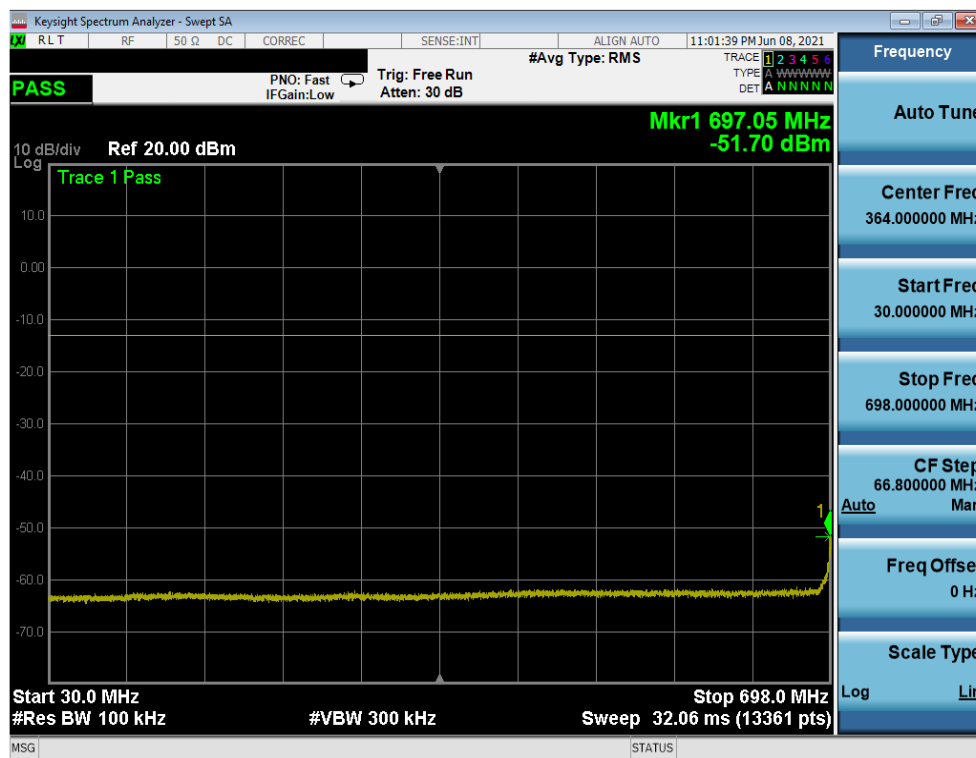
Plot 7-38. CSE (LTE Band 12/17 - 10MHz QPSK - RB Size 1, RB Offset 0 - Mid Channel)
