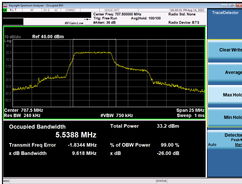
Plot 7-20. Occupied Bandwidth Plot (LTE Band 12/17 - 10MHz 16-QAM - Full RB)
