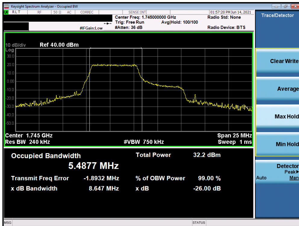
Plot 7-8. Occupied Bandwidth Plot (LTE Band 66/4 - 10MHz 16-QAM - Full RB)
