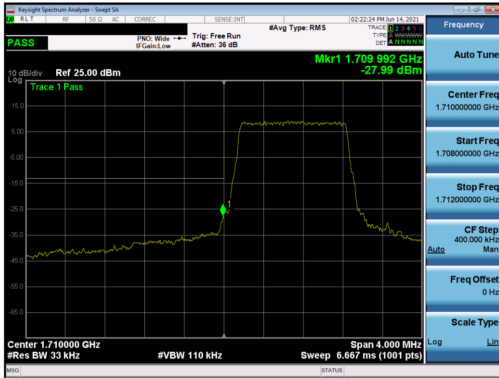
Plot 7-56. Lower Band Edge Plot (LTE Band 66 – 1.4MHz QPSK – Full RB)
