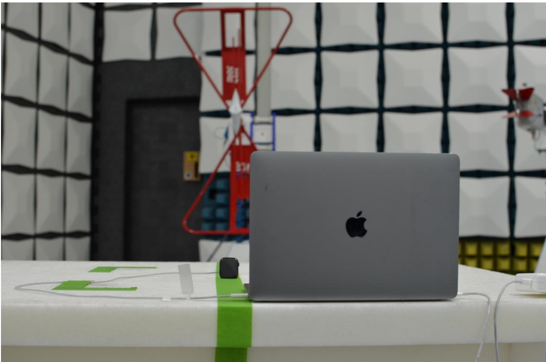
Figure 18: 30MHz-1GHz Test Setup (Rear View)
