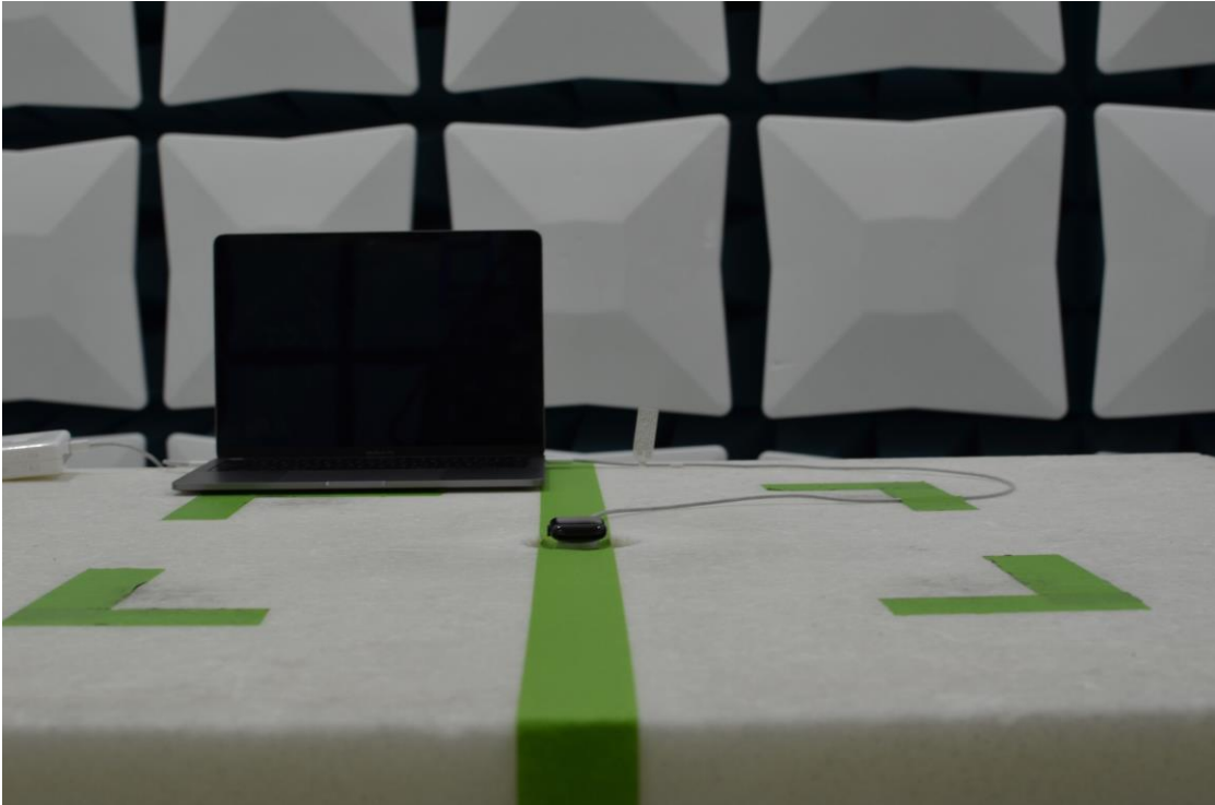
Figure 13: 30MHz-1GHz Test Setup (Front View)
