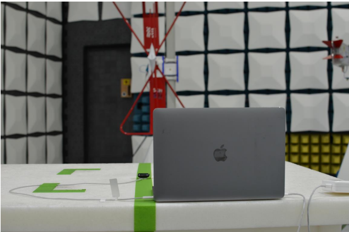
Figure 14: 30MHz-1GHz Test Setup (Rear View)
