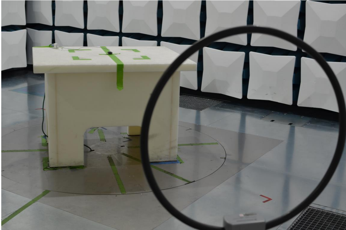
Figure 19: 9kHz-30MHz Test Setup (Front View)
