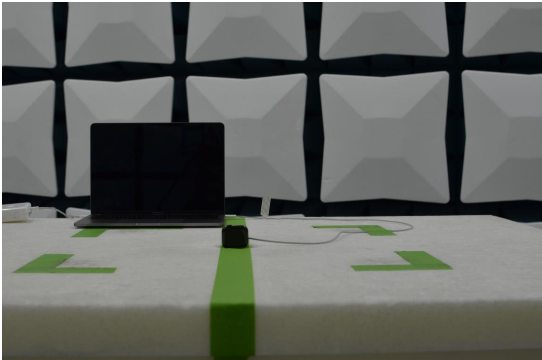
Figure 15: 30MHz-1GHz Test Setup (Front View)
