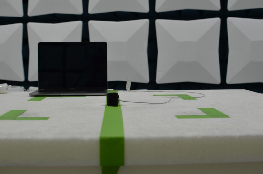
Figure 17: 30MHz-1GHz Test Setup (Front View)
