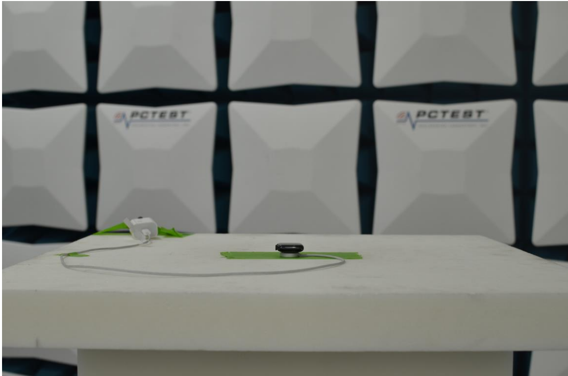
Figure 1: 1-18GHz Test Setup (Front View)
