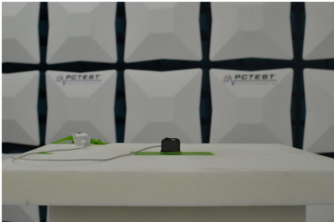
Figure 3: 1-18GHz Test Setup (Front View)
