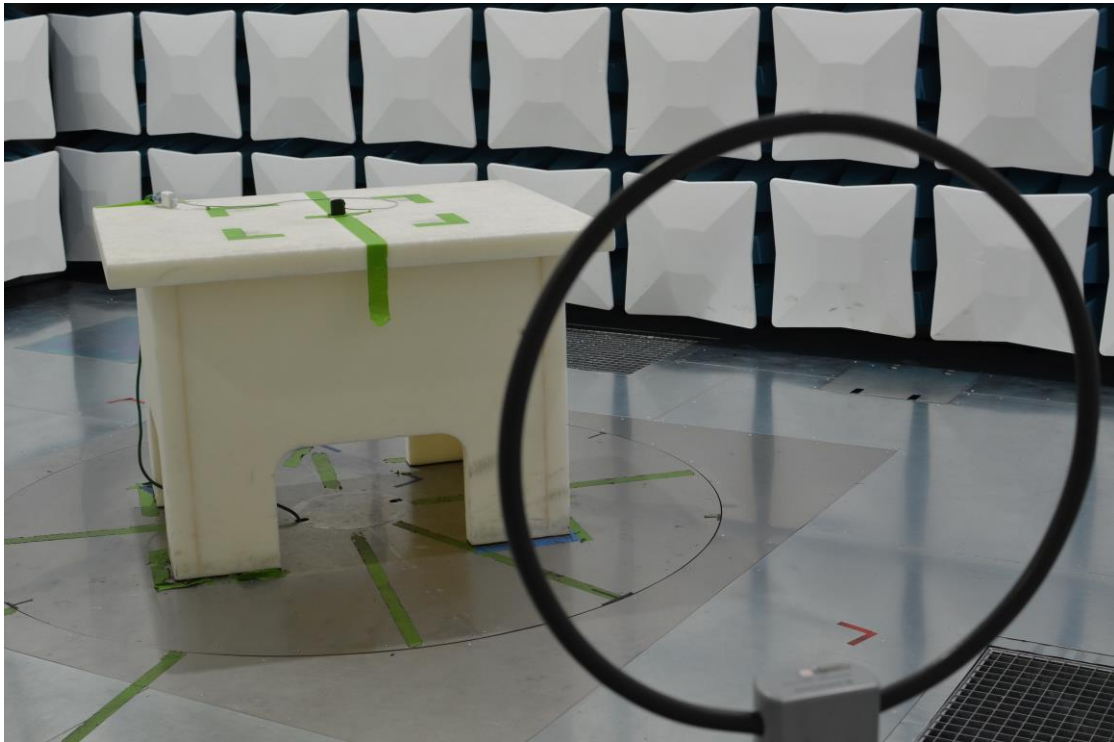
Figure 21: 9kHz-30MHz Test Setup (Front View)
