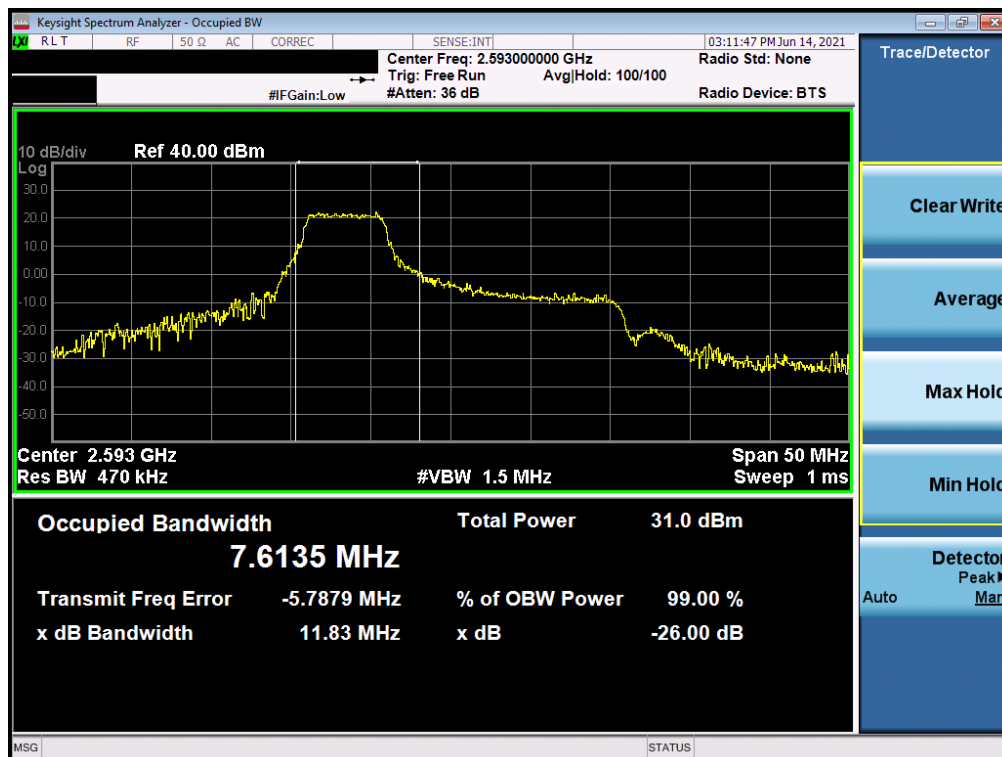
Plot 7-16. Occupied Bandwidth Plot (LTE Band 41 - 20MHz 16-QAM - Full RB)
