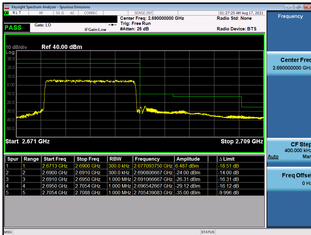
Plot 7-48. Upper ACP Plot (LTE Band 41 - 15MHz QPSK - Full RB)
