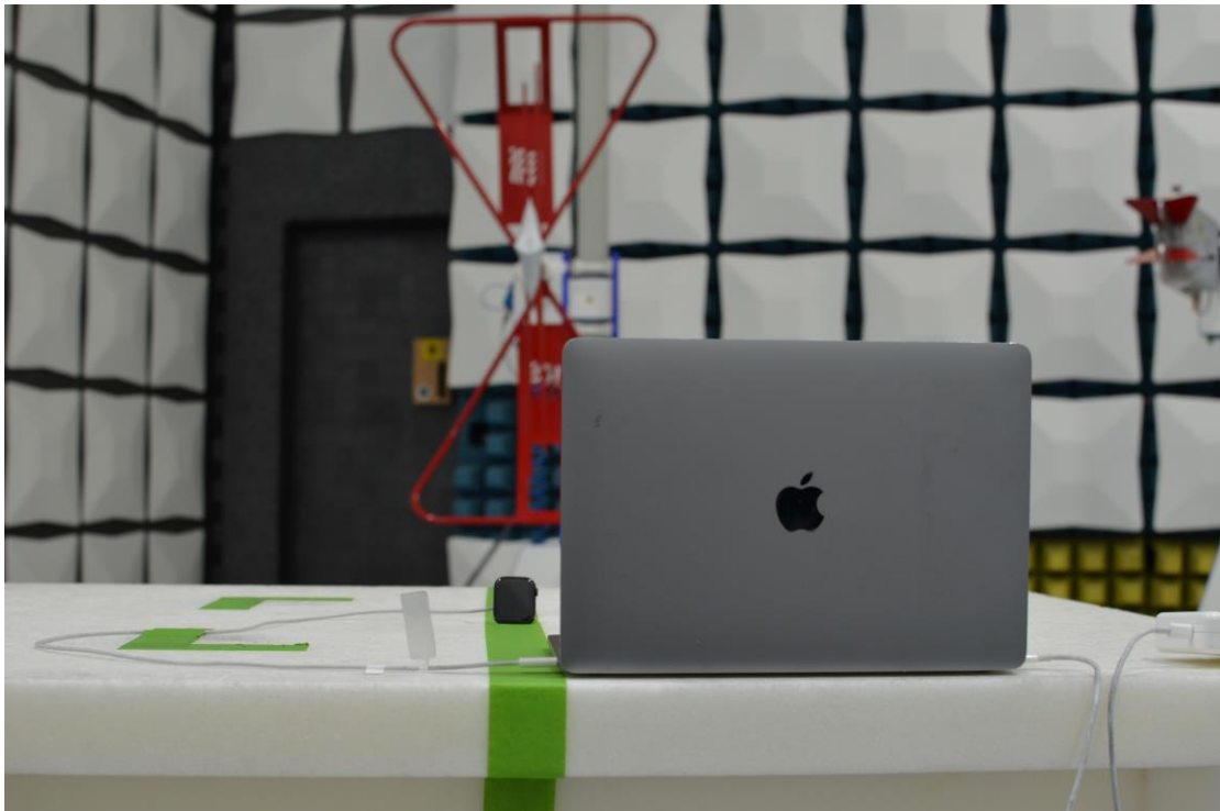
Figure 19: 30MHz-960MHz Test Setup (Rear View)
