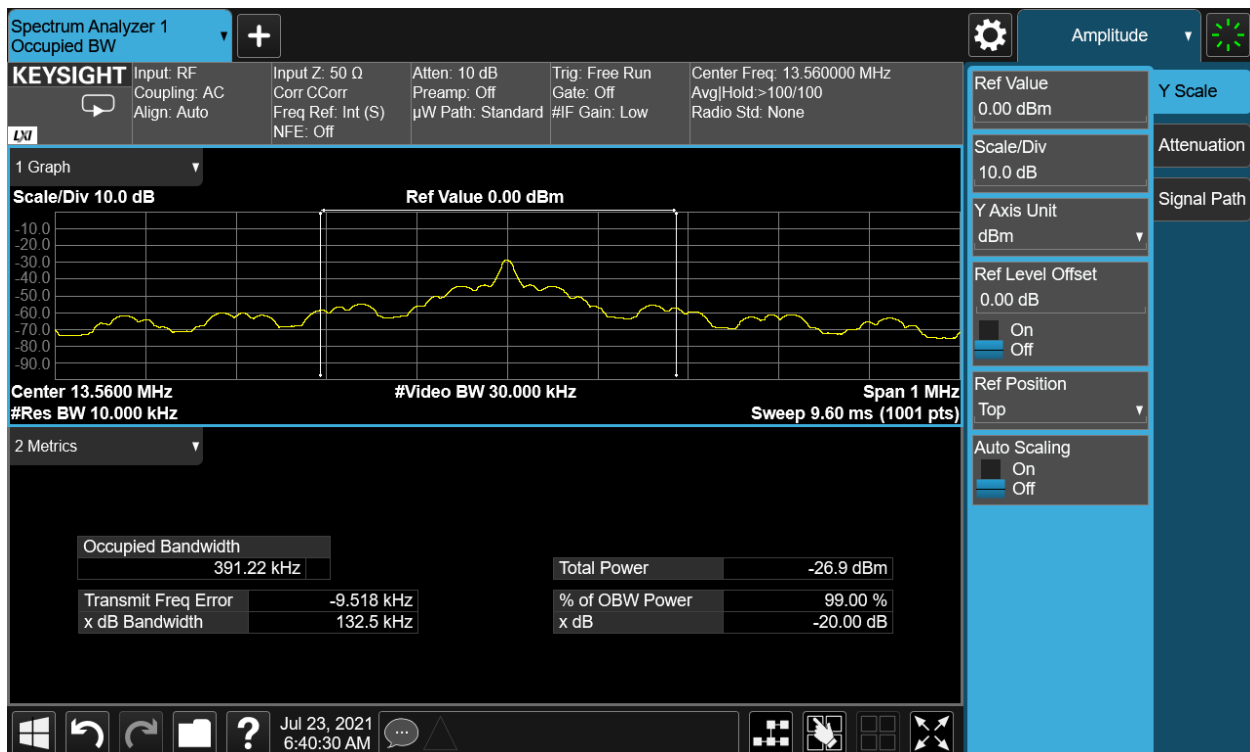
Plot 7-5. 20dB and 99% Bandwidth Plot (Reader 10% ASK 1 out of 256)
