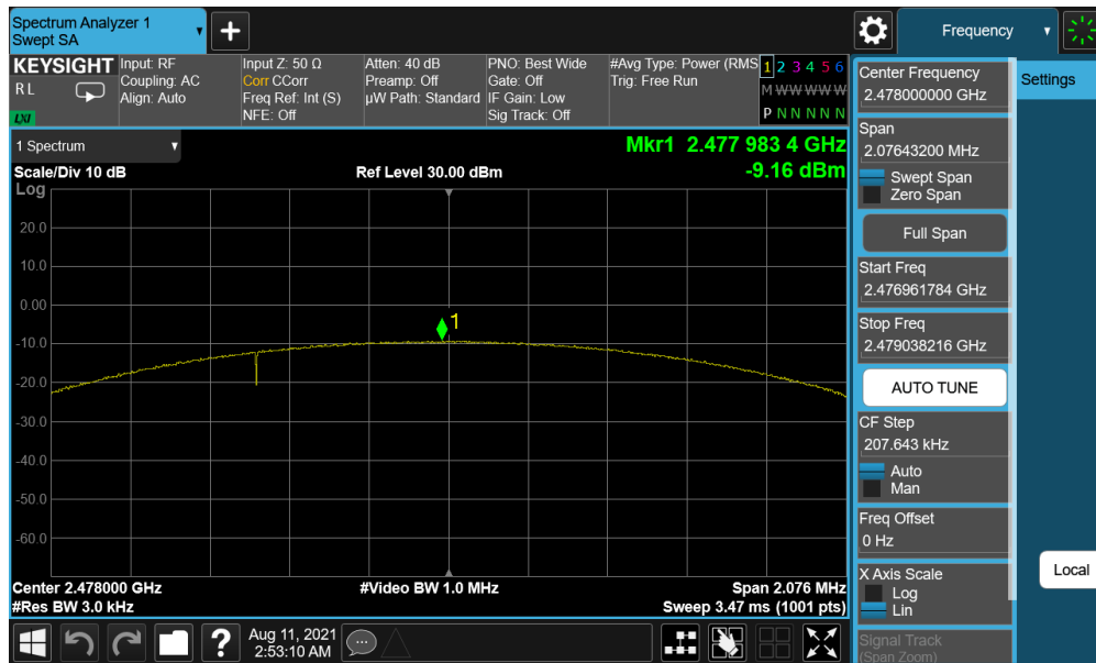
Plot 7-18. Power Spectral Density Plot (Bluetooth (LE), 2Mbps, iPA – Ch. 38)
