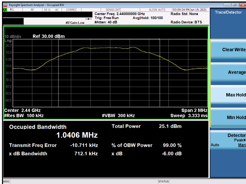
Plot 7-2. 6dB Bandwidth & 99% OBW Plot (Bluetooth (LE), 1Mbps, ePA – Ch. 19)
