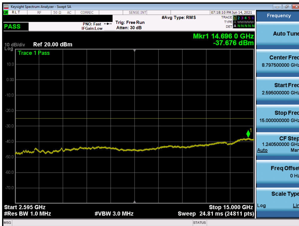
Plot 7-24. Conducted Spurious Plot (LTE Band 7 - 20MHz QPSK - RB Size 1, RB Offset 0 - High Channel)
