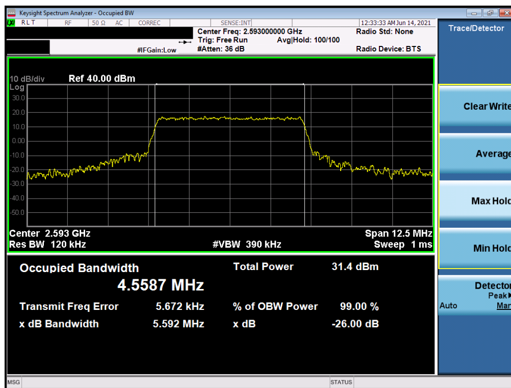
Plot 7-10. Occupied Bandwidth Plot (LTE Band 41 - 5MHz 16-QAM - Full RB)
