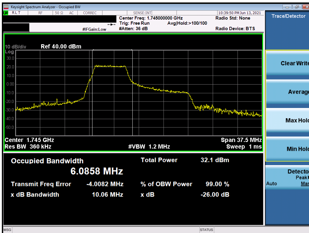
Plot 7-10. Occupied Bandwidth Plot (LTE Band 66/4 - 15MHz 16-QAM - Full RB)
