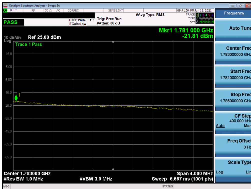
Plot 7-51. Upper Extended Band Edge Plot (LTE Band 66 - 15MHz QPSK – Full RB)
