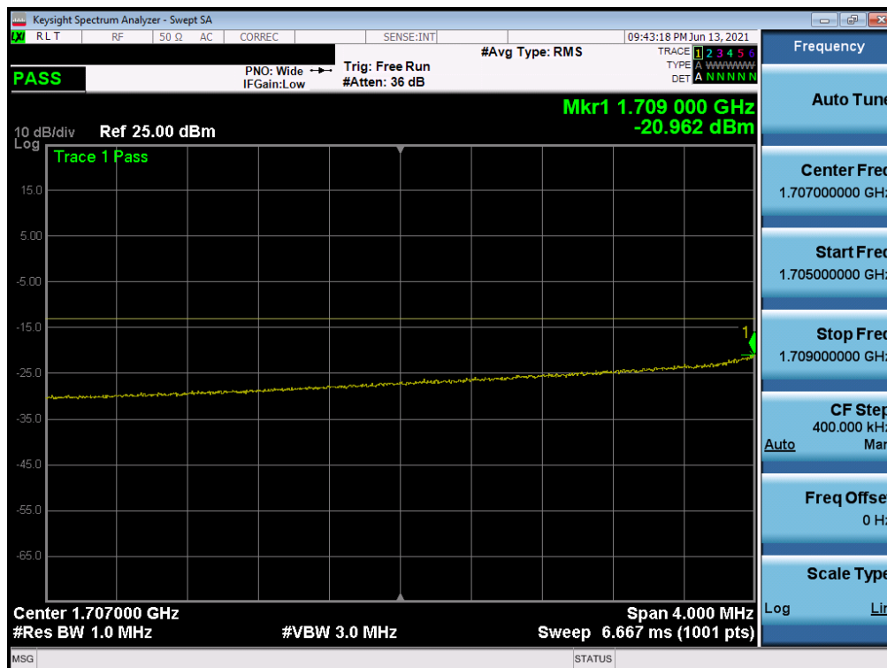
Plot 7-45. Lower Extended Band Edge Plot (LTE Band 66 - 10MHz QPSK – Full RB)
