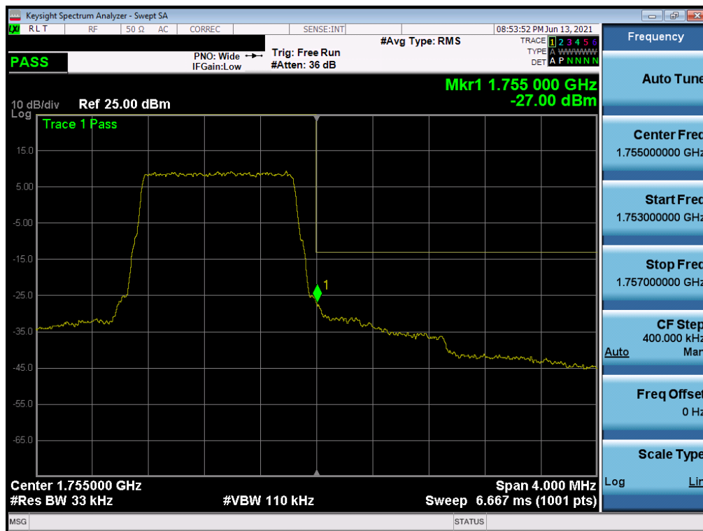
Plot 7-58. Upper Band Edge Plot (LTE Band 4 – 1.4MHz QPSK – Full RB)
