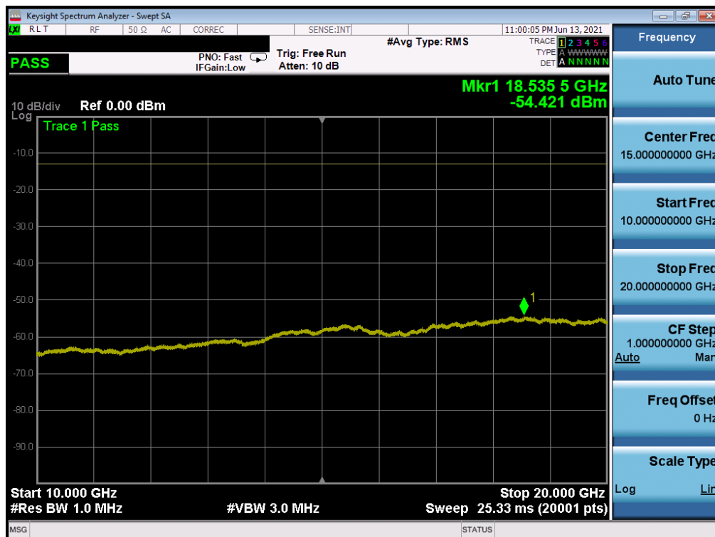
Plot 7-19. CSE (LTE Band 66/4 - 20MHz QPSK - RB Size 1, RB Offset 0 - Mid Channel)
