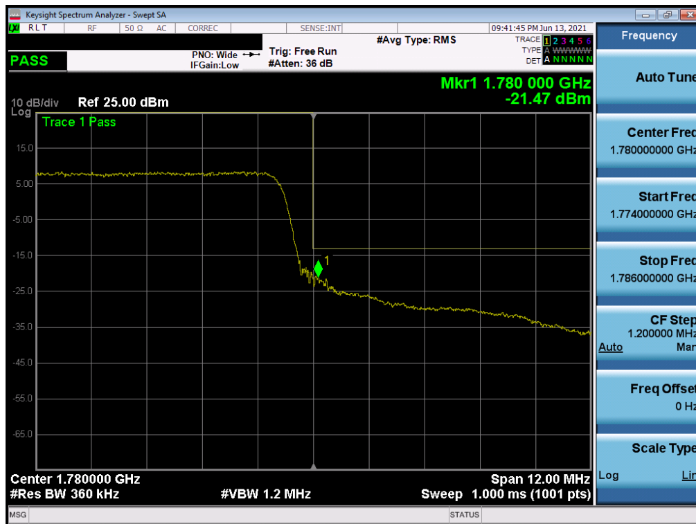
Plot 7-50. Upper Band Edge Plot (LTE Band 66 - 15MHz QPSK – Full RB)
