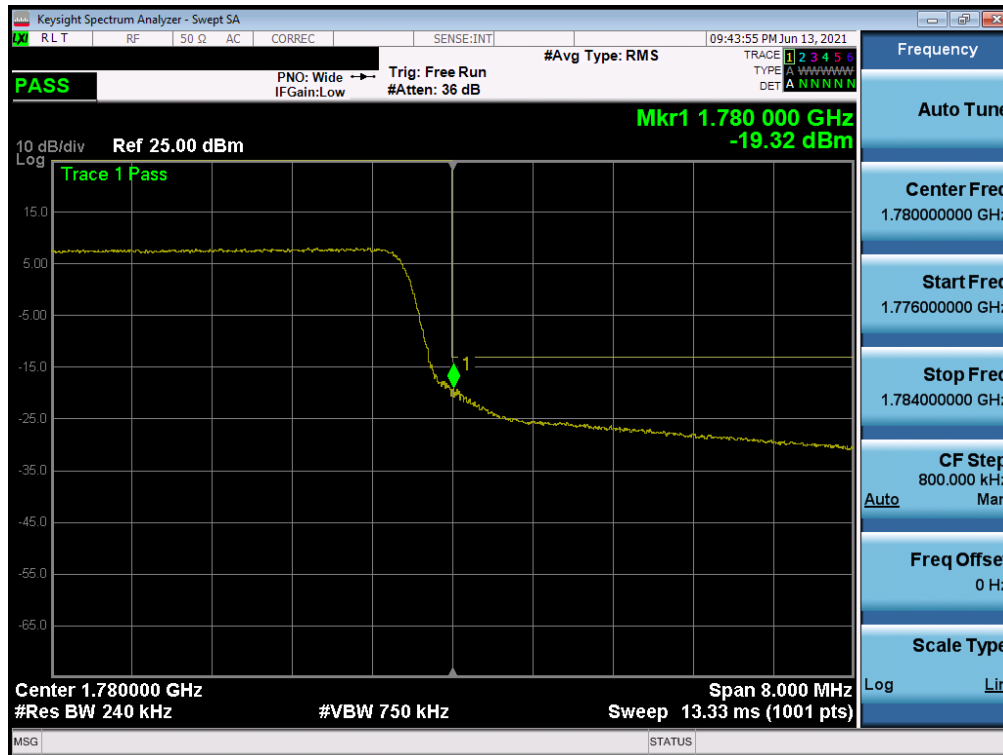
Plot 7-46. Upper Band Edge Plot (LTE Band 66 - 10MHz QPSK – Full RB)
