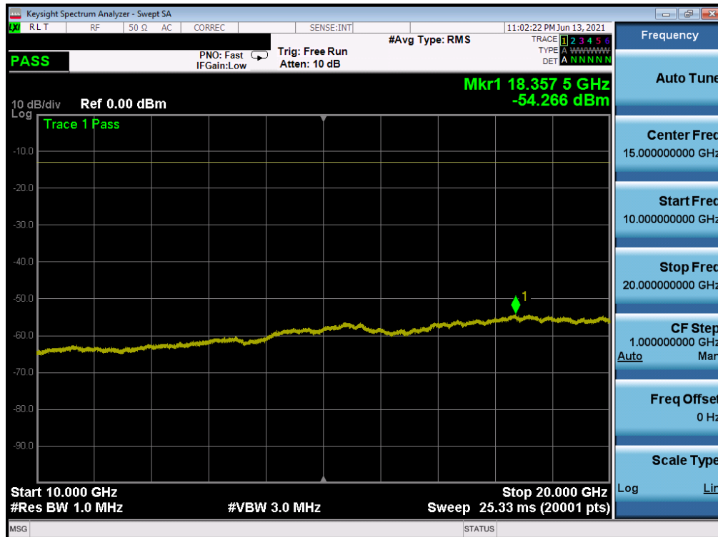
Plot 7-22. CSE (LTE Band 66/4 - 20MHz QPSK - RB Size 1, RB Offset 0 - High Channel)
